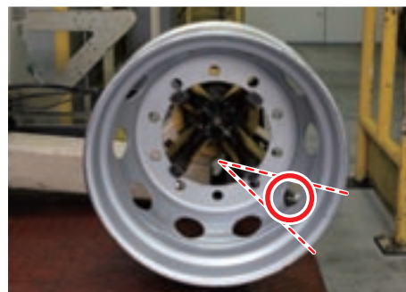
Valve is between 4 to 5 o'clock position.
