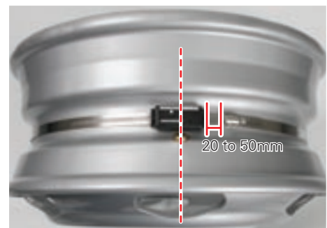
Center of sensor aligned with position of valve
