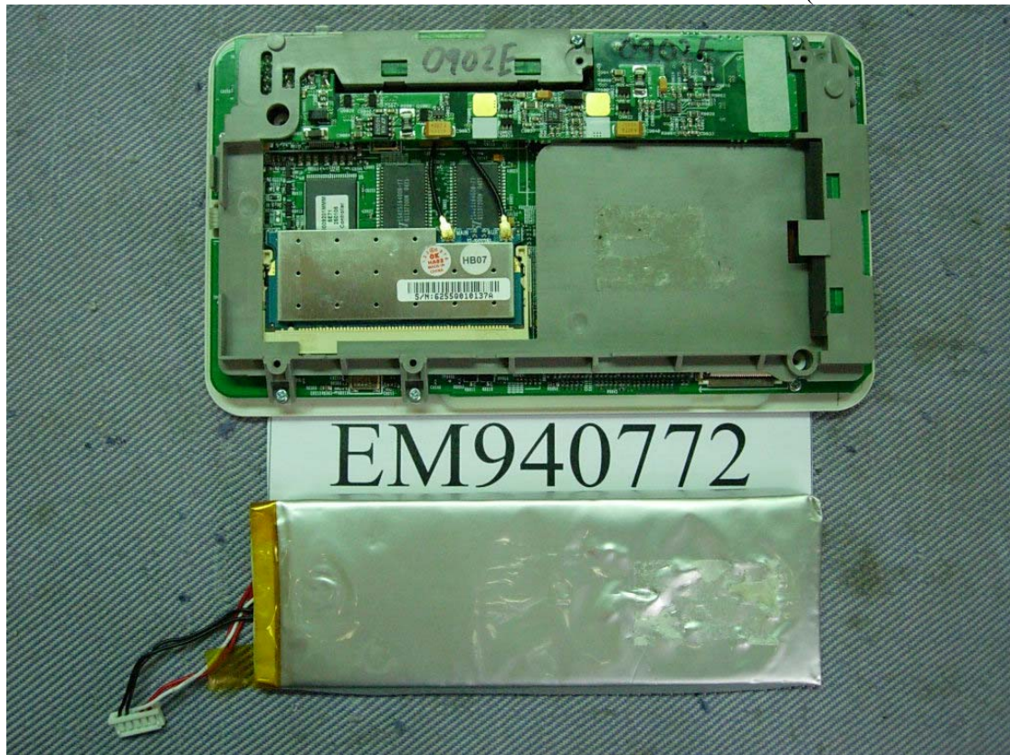
Figure 5 Internal View (Removed Battery)
