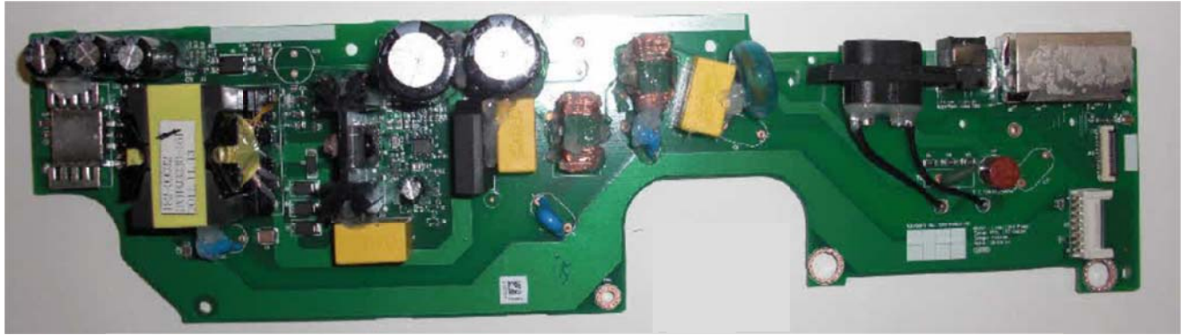
Power Supply Side 1
