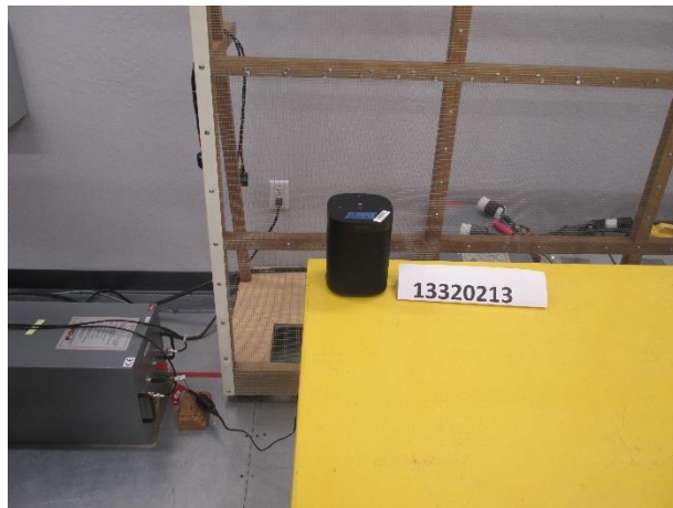
AC LINE CONDUCTED (FRONT)
