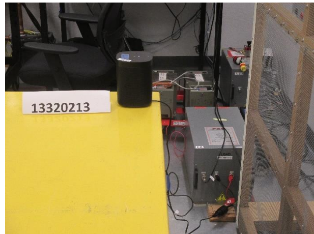
AC LINE CONDUCTED (BACK)
