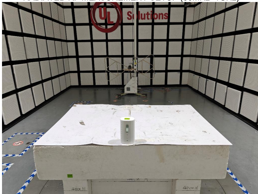
RADIATED RF MEASUREMENT SETUP (Below 30MHz)
