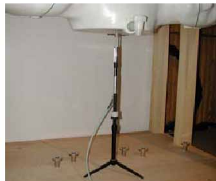
Figure 12.1 Dipole Validation Test Setup
