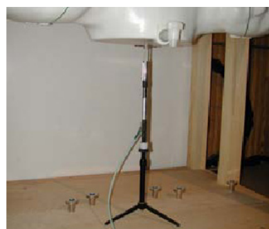
Figure 12.1 Dipole Validation Test Setup
