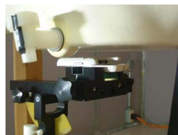
Figure 14.5 Body SAR Test Setup -- Body Position --
