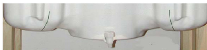
Figure 7.2 SAM Twin Phantom shell
