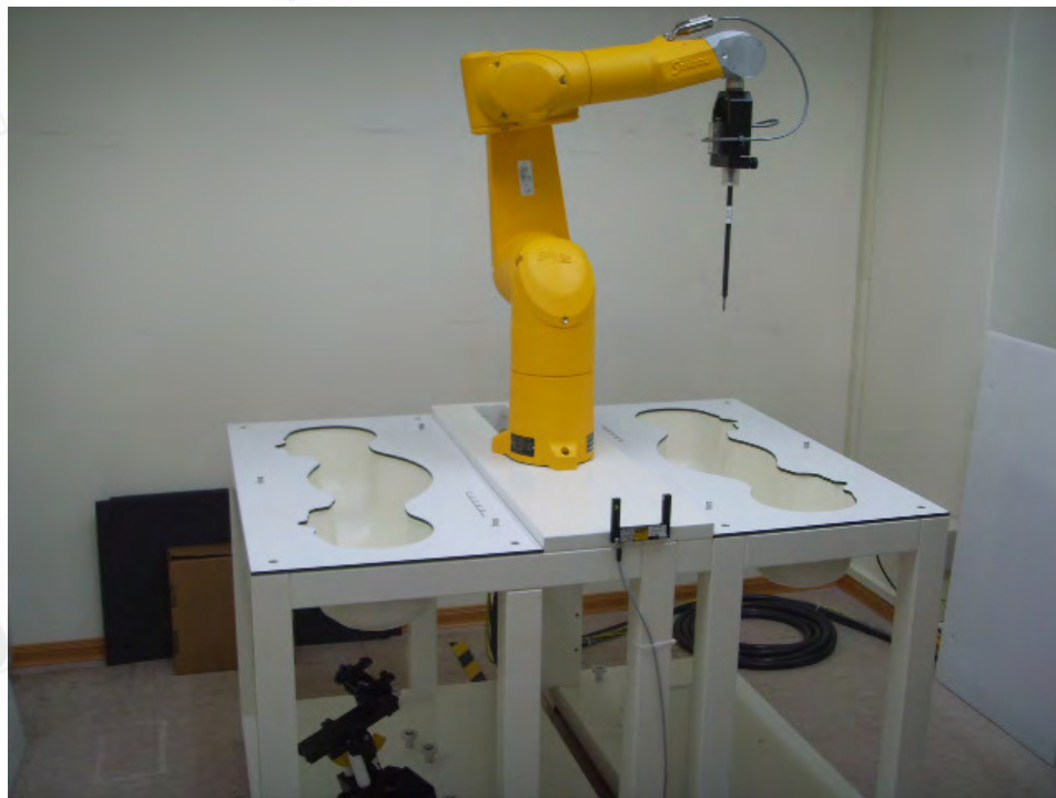
Fig.1 Photograph of the SAR measurement system
