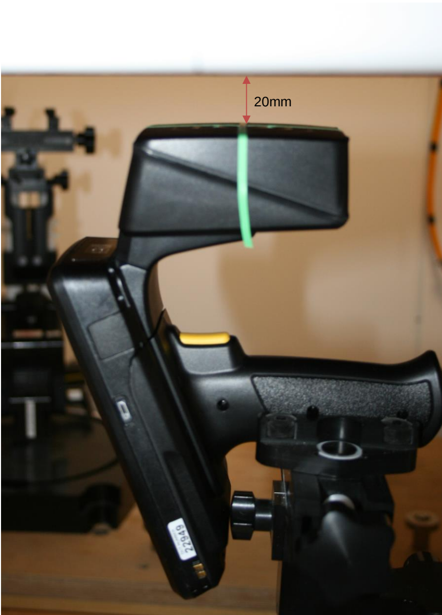
RFID reader in test position with front surface towards the phantom with 20mm separation distance.
