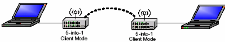
Figure 8: Client in Ad-Hoc Mode
