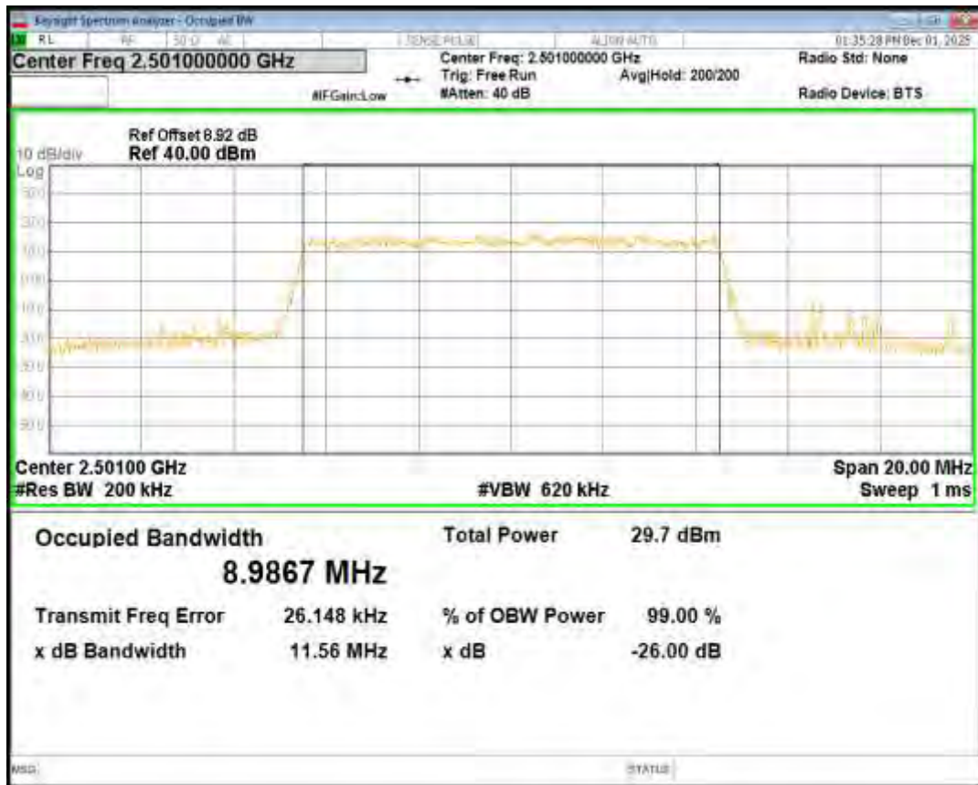
Band41 16QAM BW=10MHz Channel=40620 RB Size=50 Position=#0
