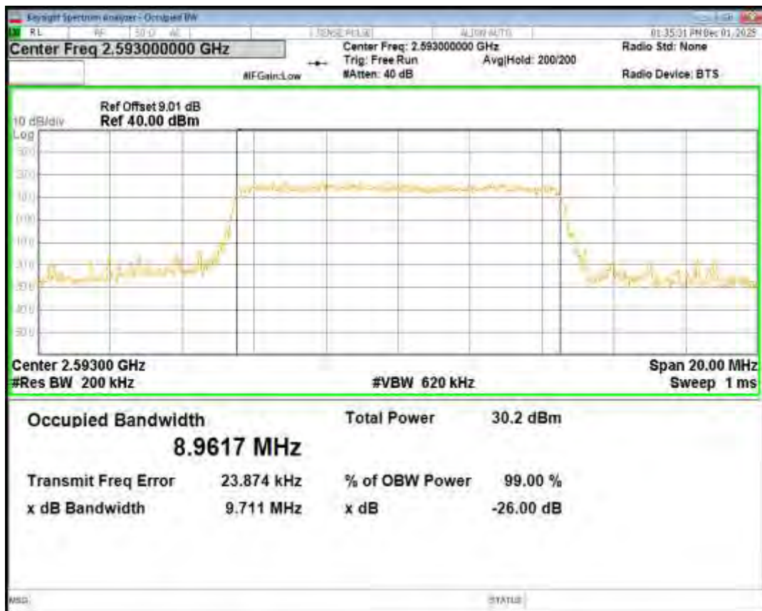
Band41 QPSK BW=15MHz Channel=40620 RB Size=75 Position=#0
