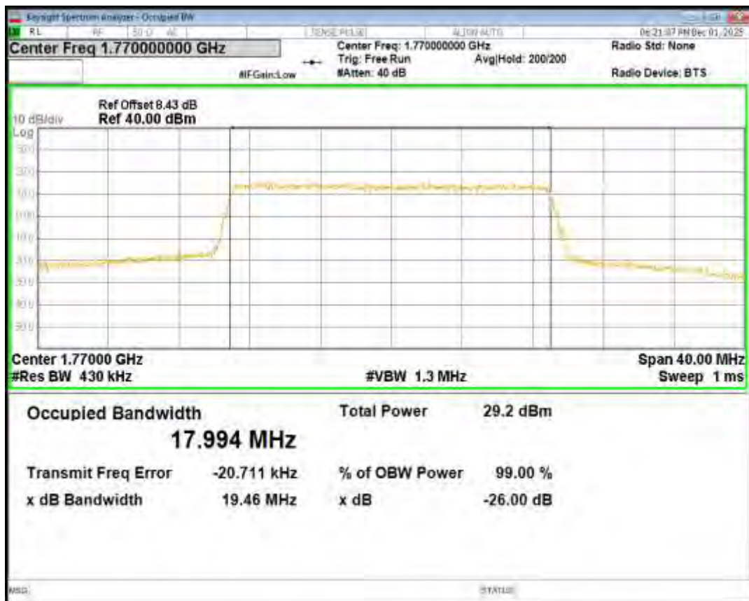
Band66 QPSK BW=3MHz Channel=131987 RB Size=15 Position=#0
