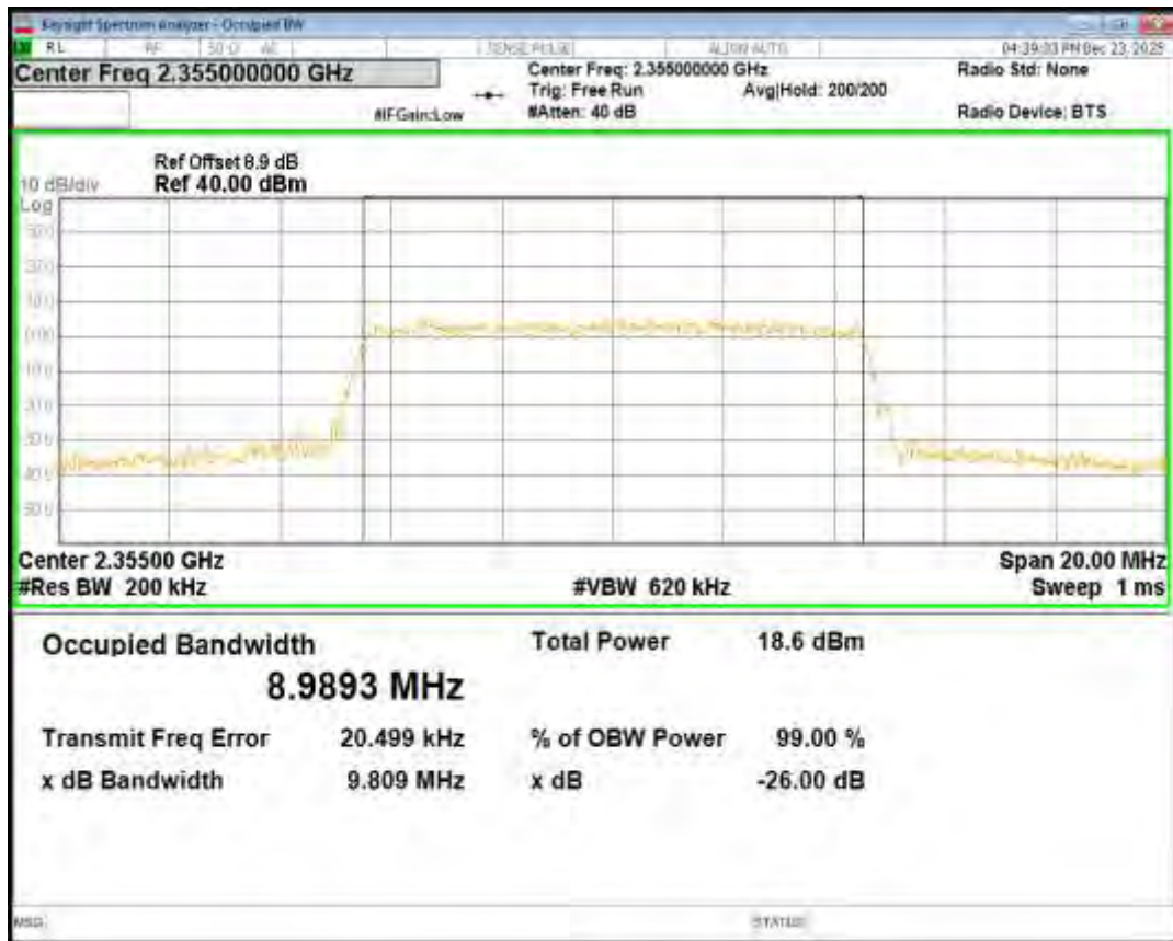
Band40(2350-2360) 16QAM BW=5MHz Channel=39175 RB Size=25 Position=#0
