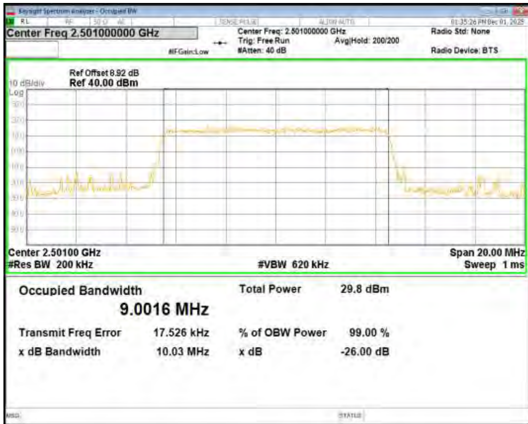
Band41 QPSK BW=10MHz Channel=40620 RB Size=50 Position=#0
