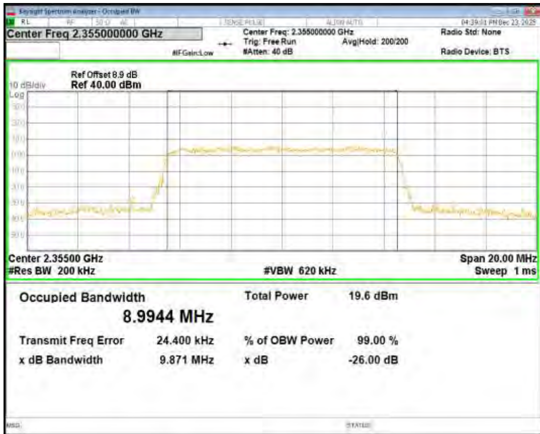
Band40(2350-2360) QPSK BW=5MHz Channel=39175 RB Size=25 Position=#0
