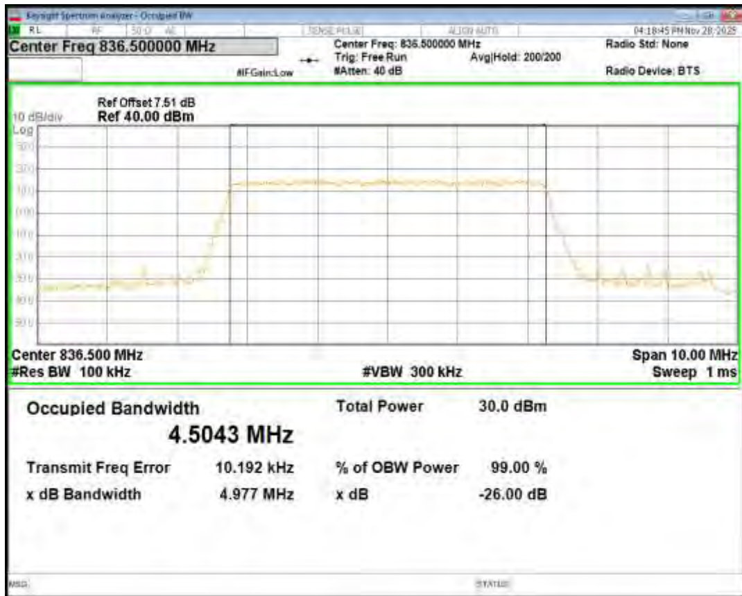
Band5 QPSK BW=5MHz Channel=20625 RB Size=25 Position=#0
