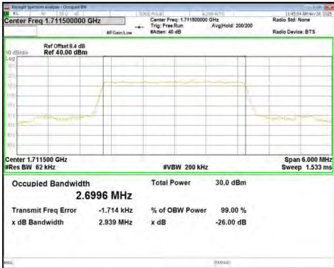
Band4 QPSK BW=3MHz Channel=20175 RB Size=15 Position=#0
