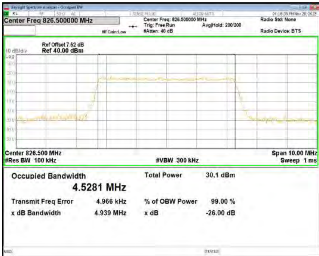
Band5 QPSK BW=5MHz Channel=20525 RB Size=25 Position=#0
