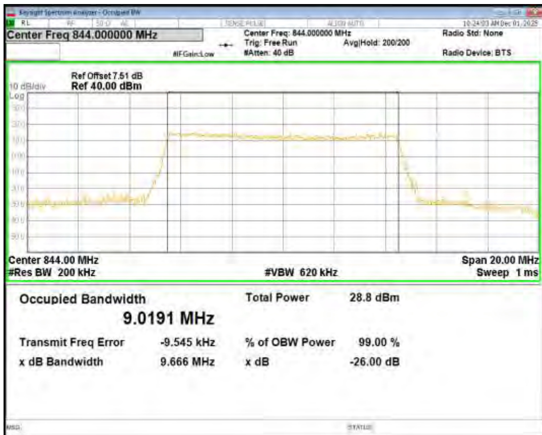
Band26(824-849) 16QAM BW=15MHz Channel=26865 RB Size=75 Position=#0
