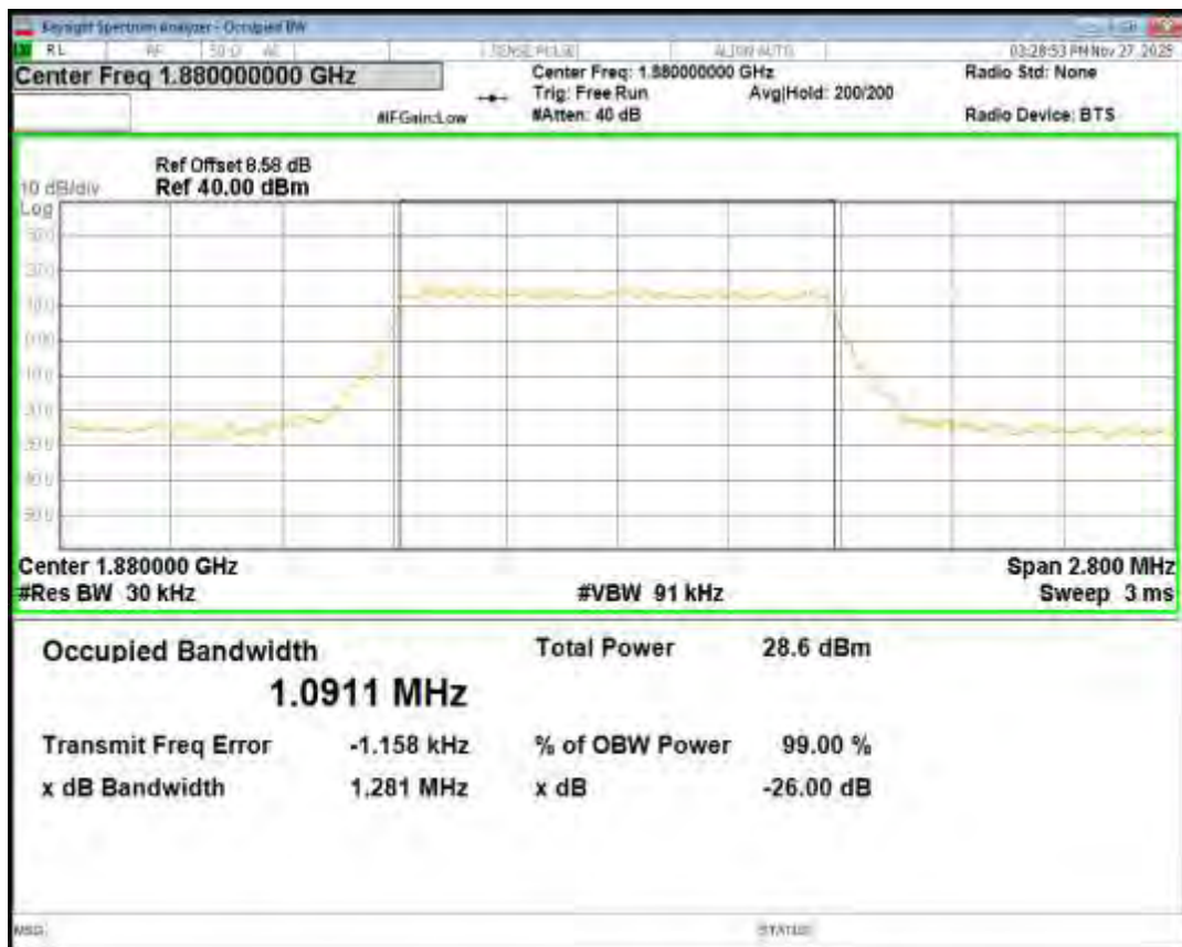
Band2 16QAM BW=1.4MHz Channel=19193 RB Size=6 Position=#0
