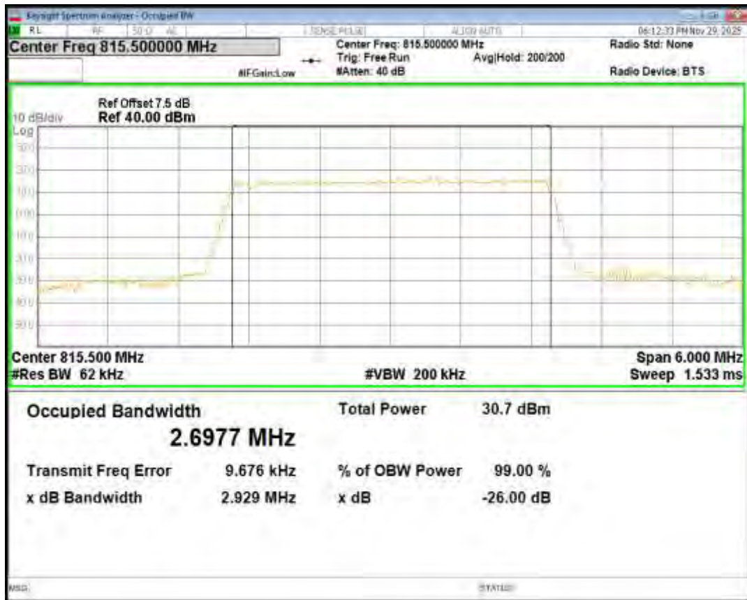
Band26(814-824) QPSK BW=3MHz Channel=26740 RB Size=15 Position=#0
