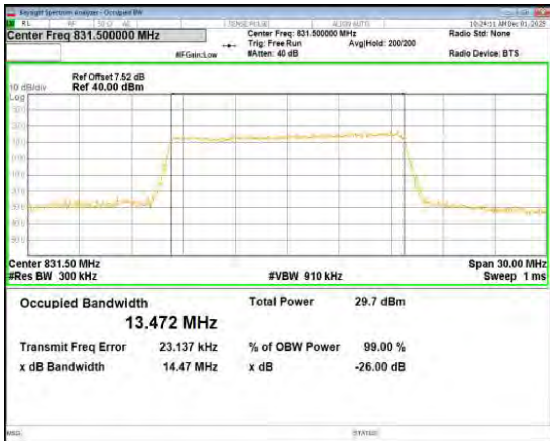
Band26(824-849) QPSK BW=15MHz Channel=26915 RB Size=75 Position=#0
