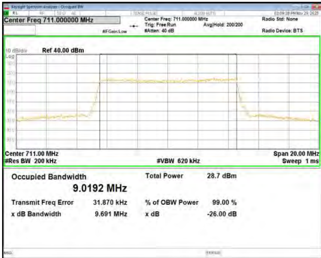
Band17 16QAM BW=5MHz Channel=23755 RB Size=25 Position=#0
