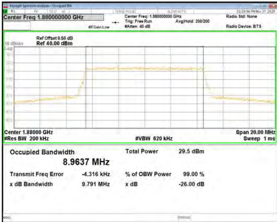
Band2 QPSK BW=20MHz Channel=18900 RB Size=100 Position=#0
