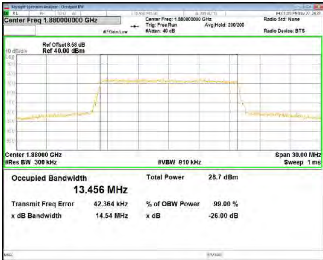
Band2 16QAM BW=5MHz Channel=18625 RB Size=25 Position=#0
