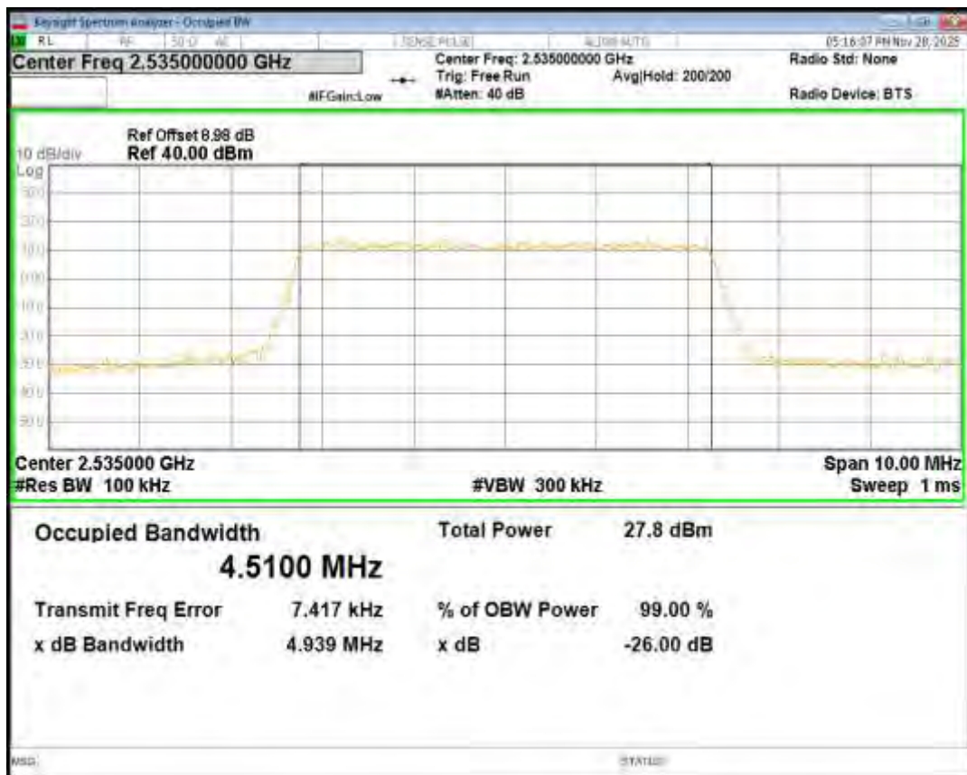
Band7 QPSK BW=10MHz Channel=20800 RB Size=50 Position=#0
