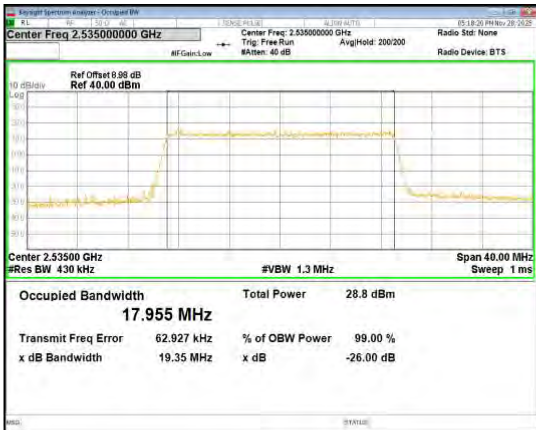
Band7 QPSK BW=20MHz Channel=21350 RB Size=100 Position=#0
