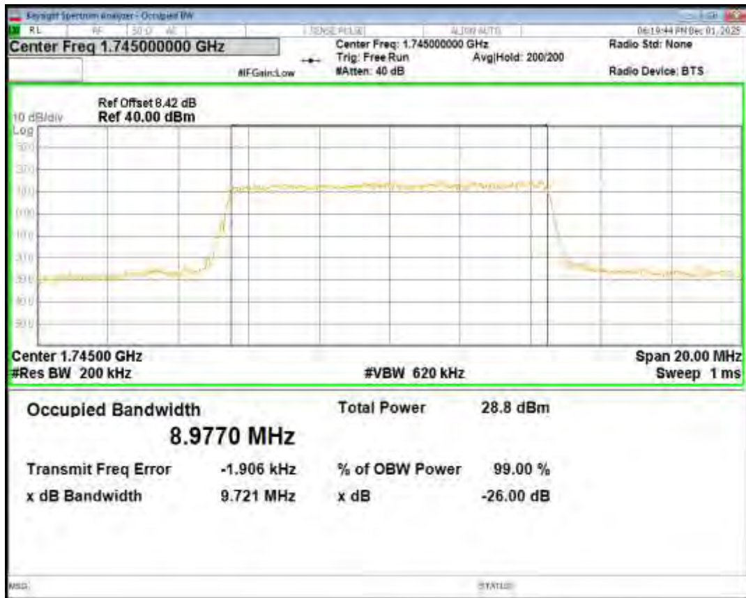
Band66 QPSK BW=15MHz Channel=132597 RB Size=75 Position=#0
