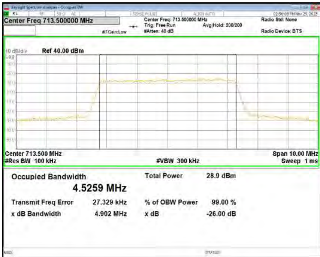
Band17 QPSK BW=10MHz Channel=23780 RB Size=50 Position=#0
