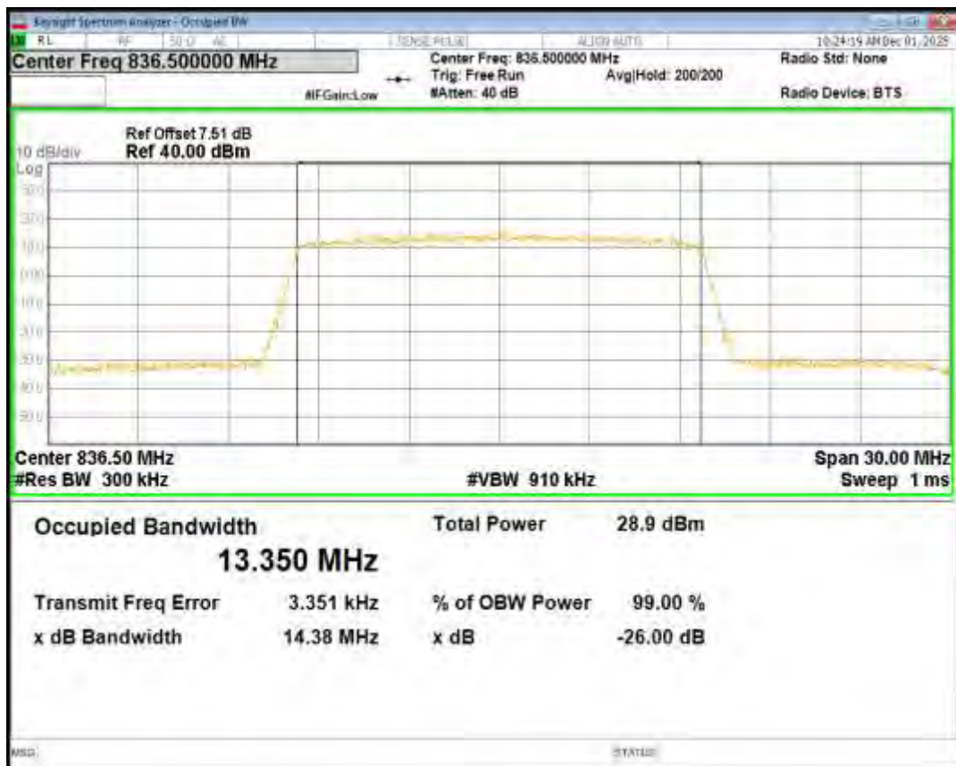
Band26(824-849) 16QAM BW=15MHz Channel=26965 RB Size=75 Position=#0
