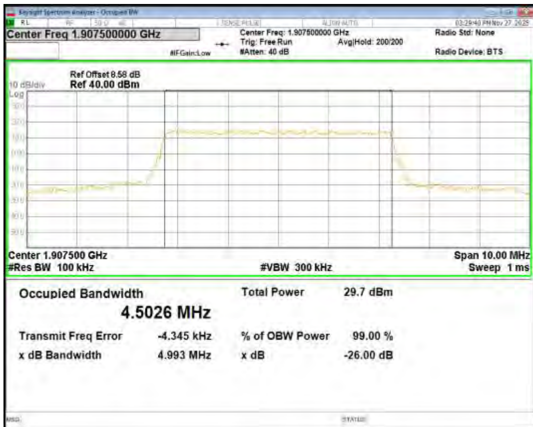
Band25 16QAM BW=1.4MHz Channel=26047 RB Size=6 Position=#0
