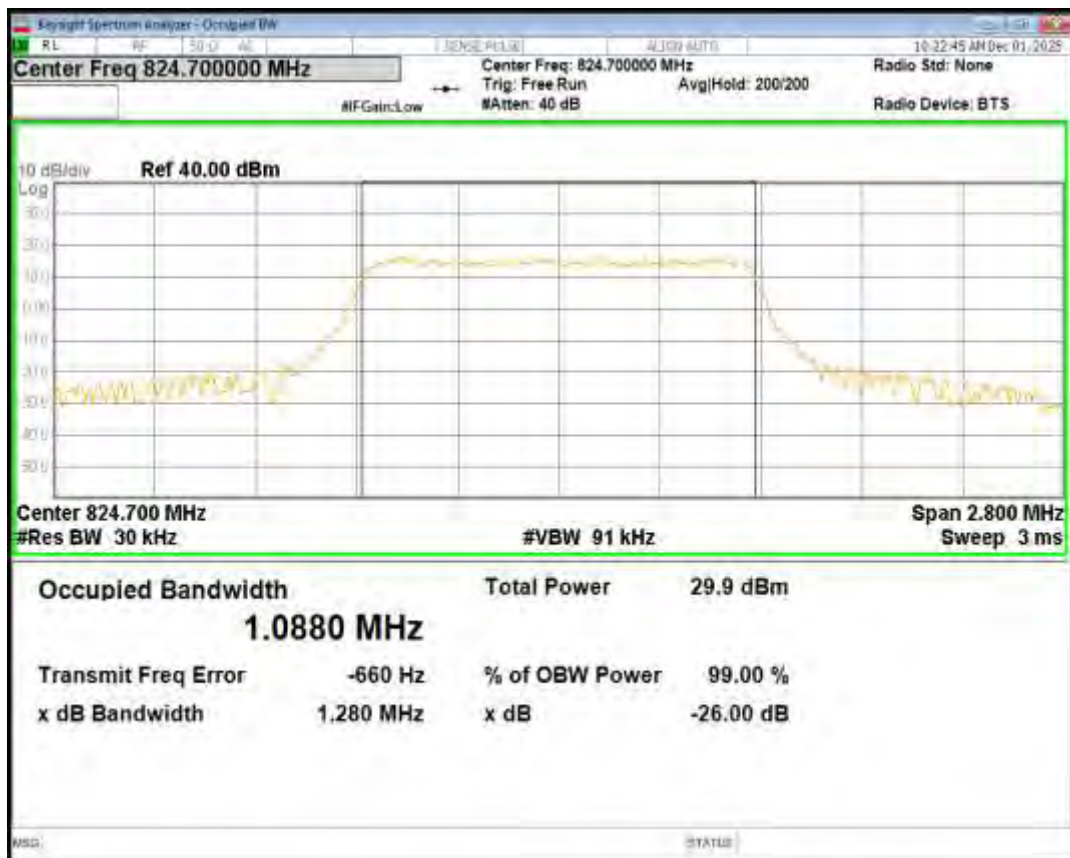
Band26(824-849) 16QAM BW=5MHz Channel=27015 RB Size=25 Position=#0
