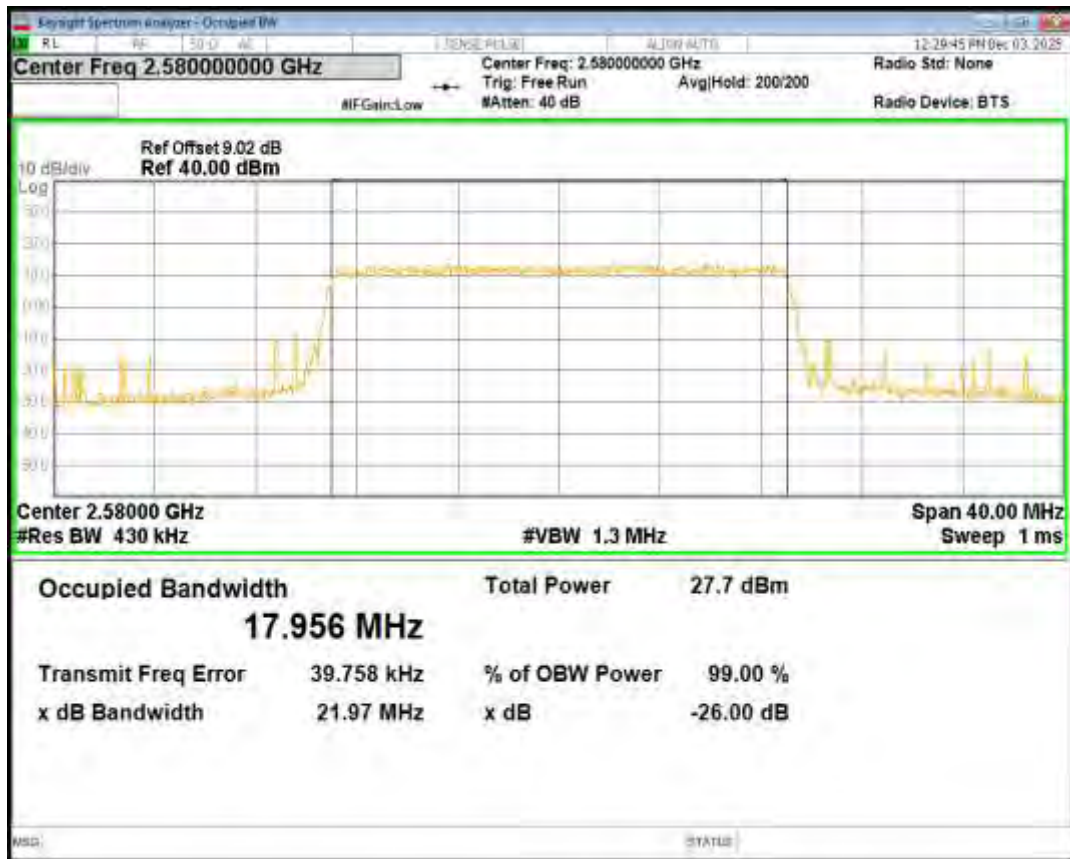
Band38 16QAM BW=20MHz Channel=38000 RB Size=100 Position=#0
