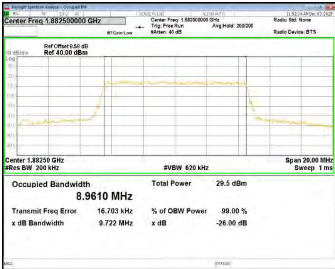
Band25 QPSK BW=10MHz Channel=26640 RB Size=50 Position=#0
