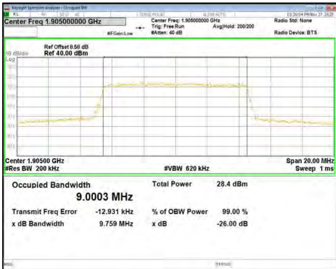
Band2 16QAM BW=15MHz Channel=18900 RB Size=75 Position=#0
