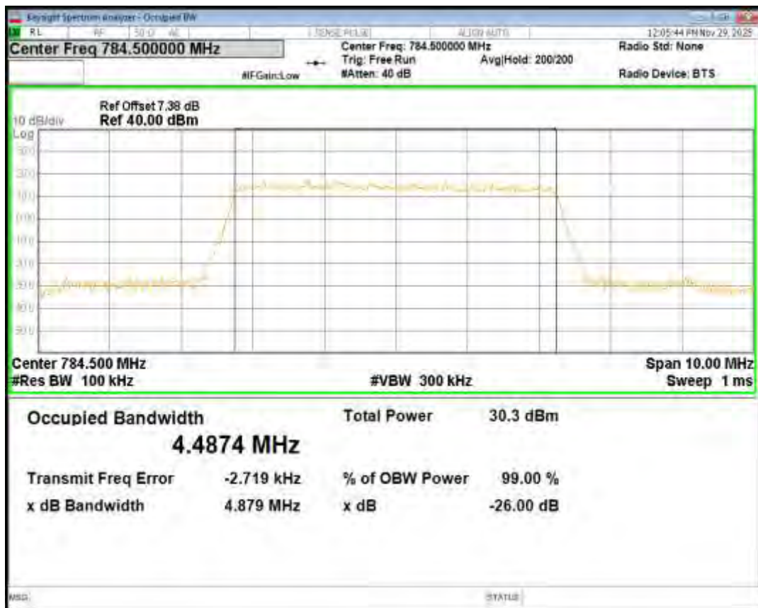
Band14 16QAM BW=10MHz Channel=23330 RB Size=50 Position=#0
