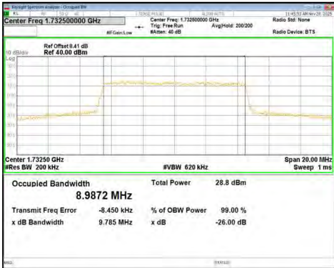
Band4 QPSK BW=20MHz Channel=20050 RB Size=100 Position=#0
