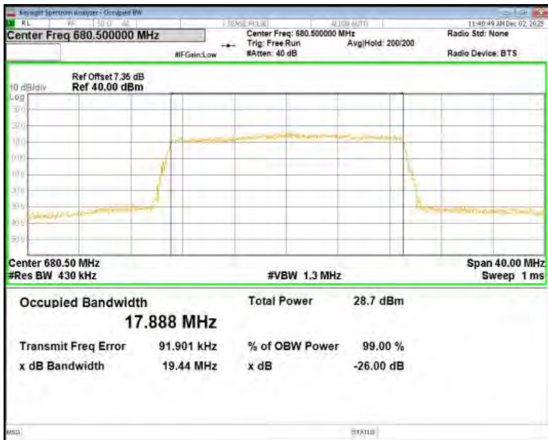
Band71 16QAM BW=20MHz Channel=133372 RB Size=100 Position=#0
