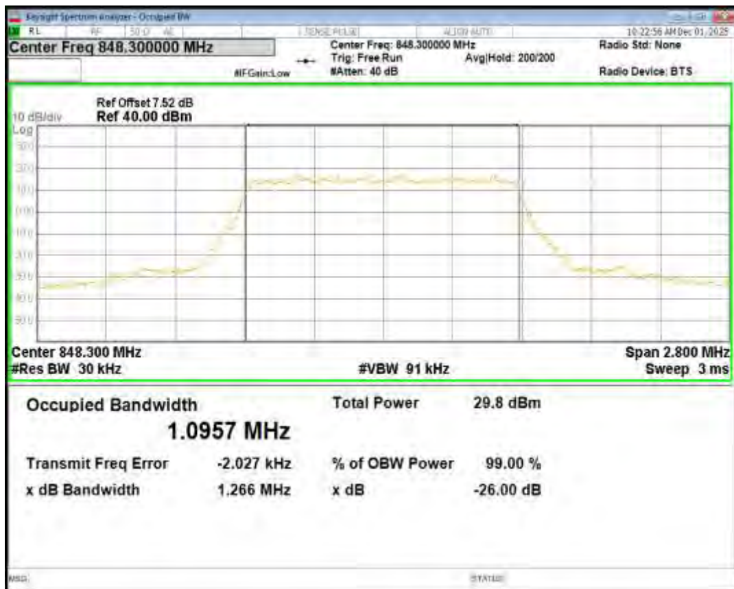
Band26(824-849) QPSK BW=10MHz Channel=26840 RB Size=50 Position=#0
