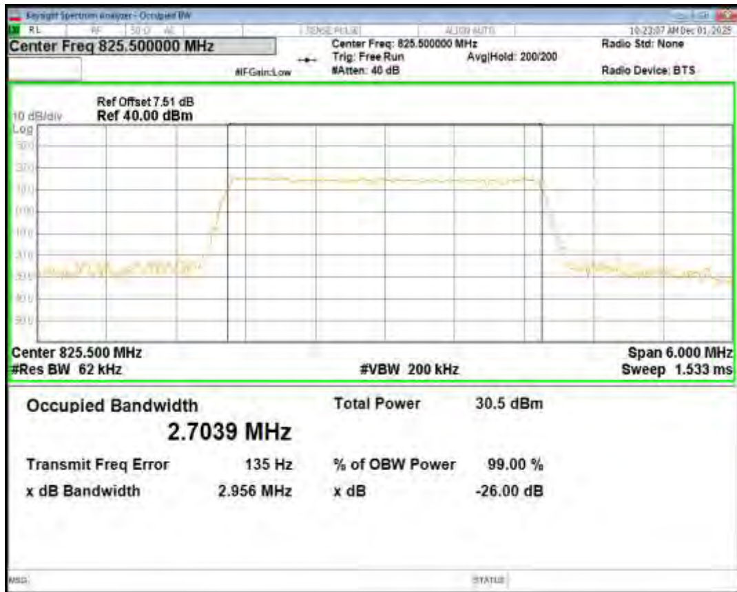
Band26(824-849) QPSK BW=3MHz Channel=26915 RB Size=15 Position=#0
