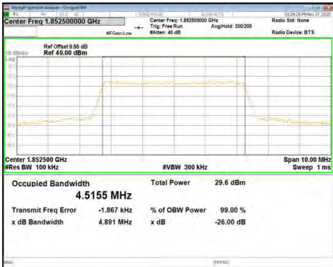
Band2 QPSK BW=5MHz Channel=18900 RB Size=25 Position=#0
