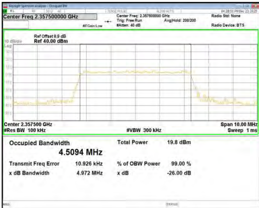
Band41 16QAM BW=10MHz Channel=39700 RB Size=50 Position=#0
