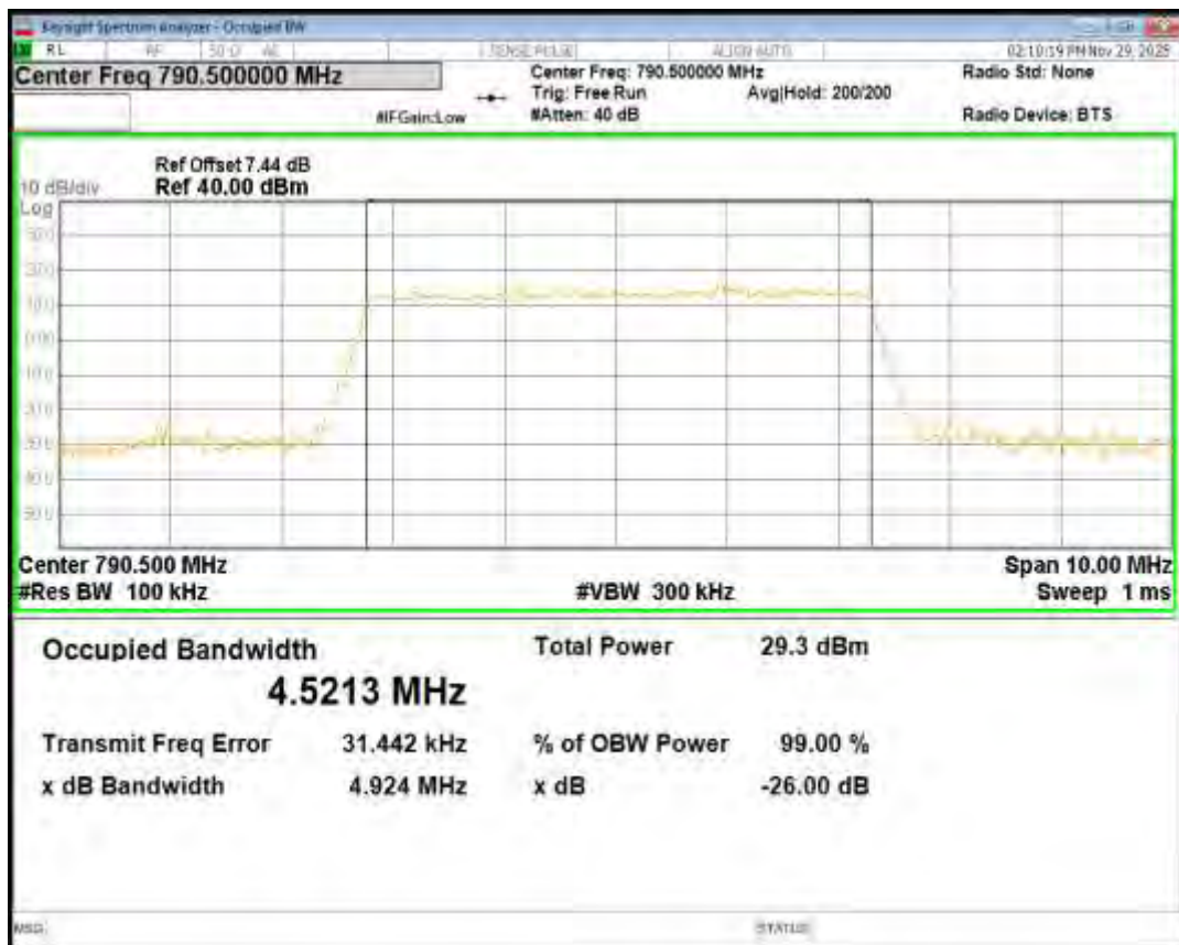
Band14 16QAM BW=5MHz Channel=23330 RB Size=25 Position=#0
