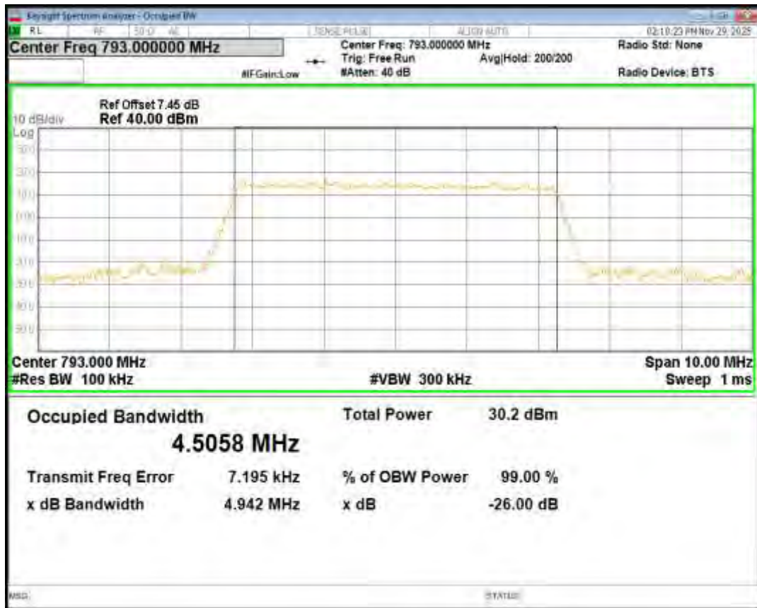
Band14 QPSK BW=5MHz Channel=23355 RB Size=25 Position=#0
