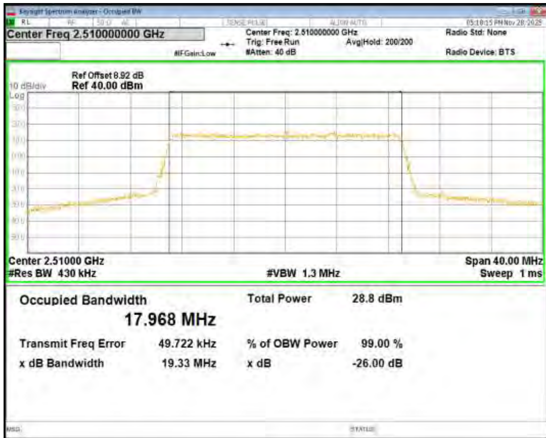
Band7 QPSK BW=20MHz Channel=21100 RB Size=100 Position=#0
