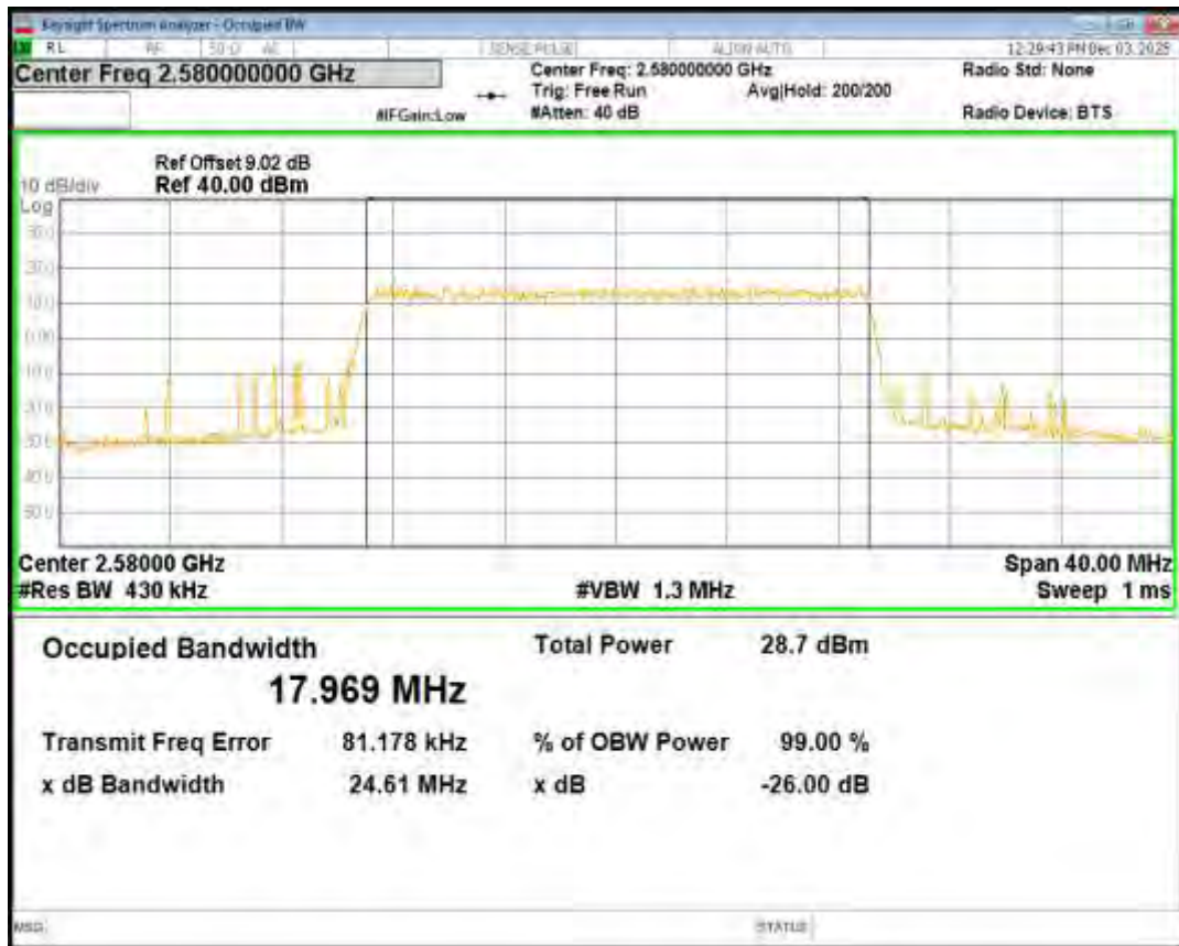
Band38 QPSK BW=20MHz Channel=38000 RB Size=100 Position=#0
