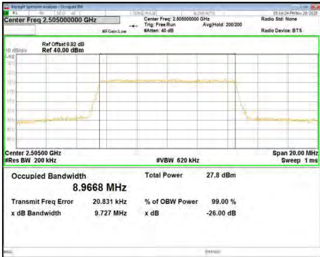
Band7 16QAM BW=10MHz Channel=21100 RB Size=50 Position=#0
