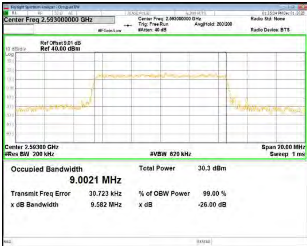
Band41 16QAM BW=10MHz Channel=41540 RB Size=50 Position=#0
