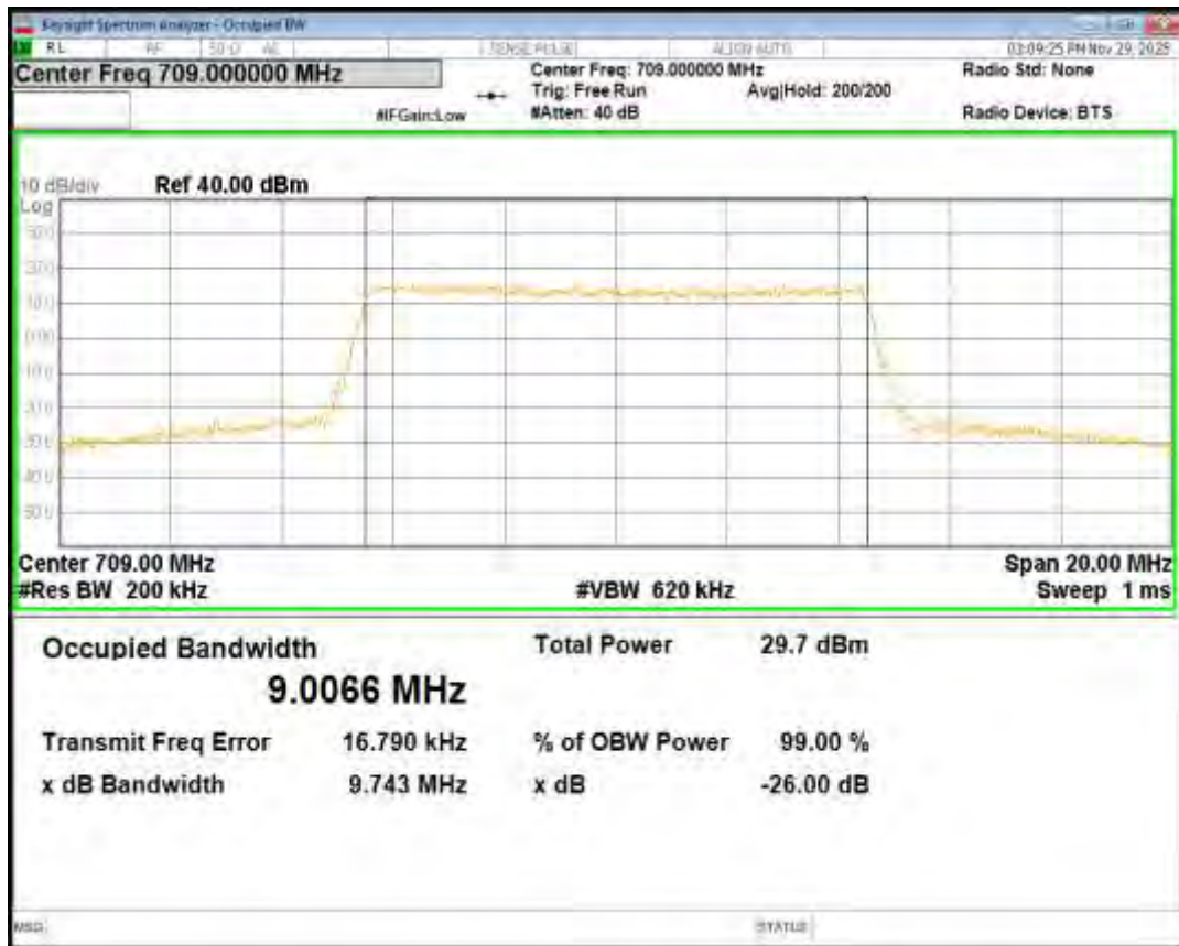
Band17 QPSK BW=10MHz Channel=23790 RB Size=50 Position=#0
