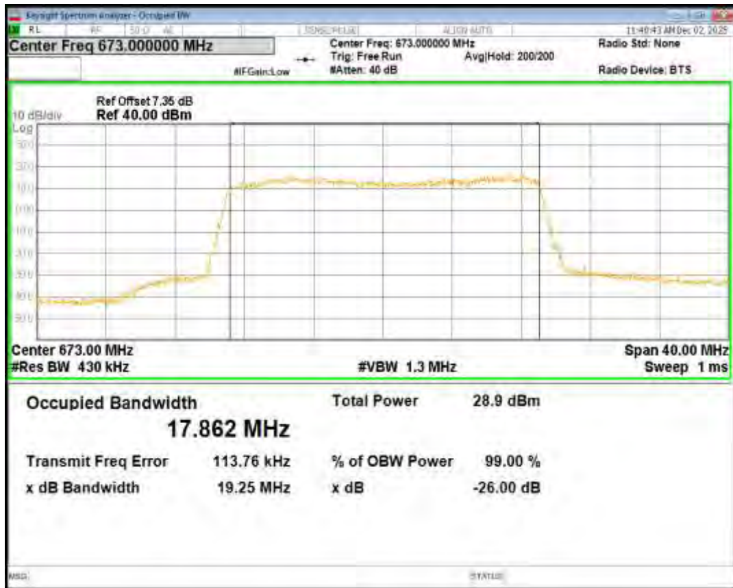
Band71 16QAM BW=20MHz Channel=133297 RB Size=100 Position=#0
