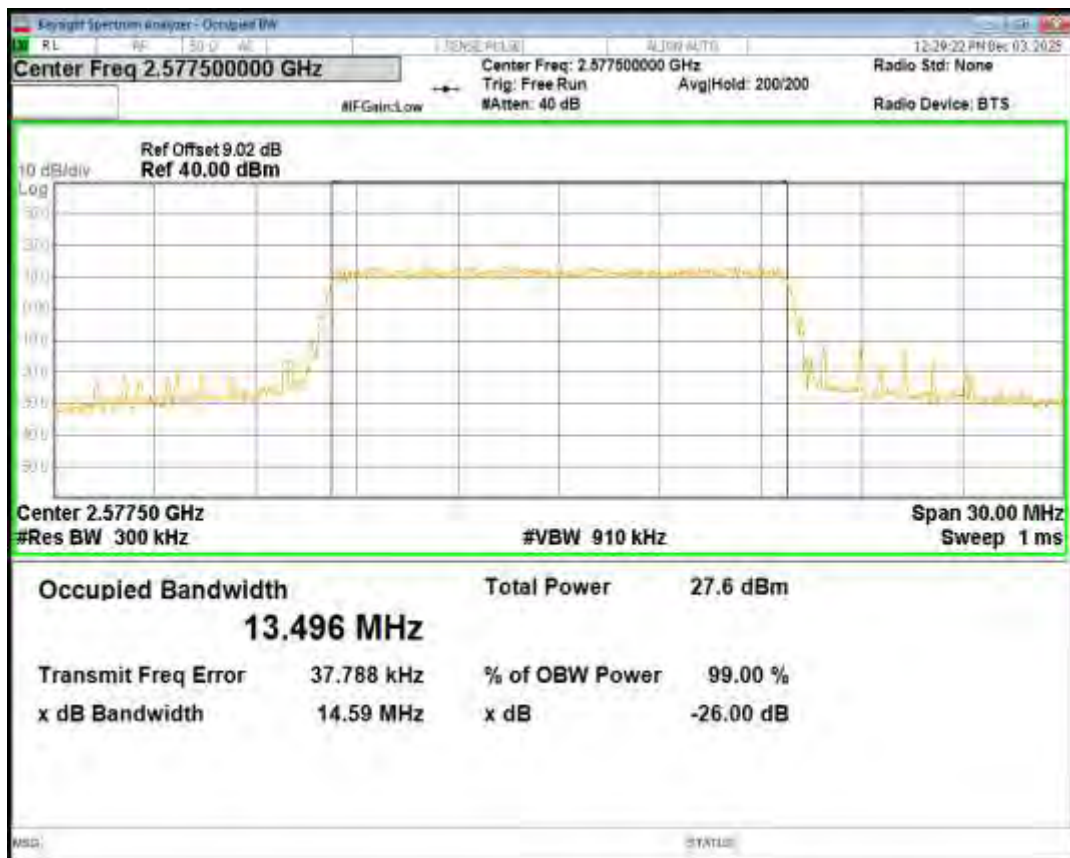
Band38 16QAM BW=15MHz Channel=38000 RB Size=75 Position=#0
