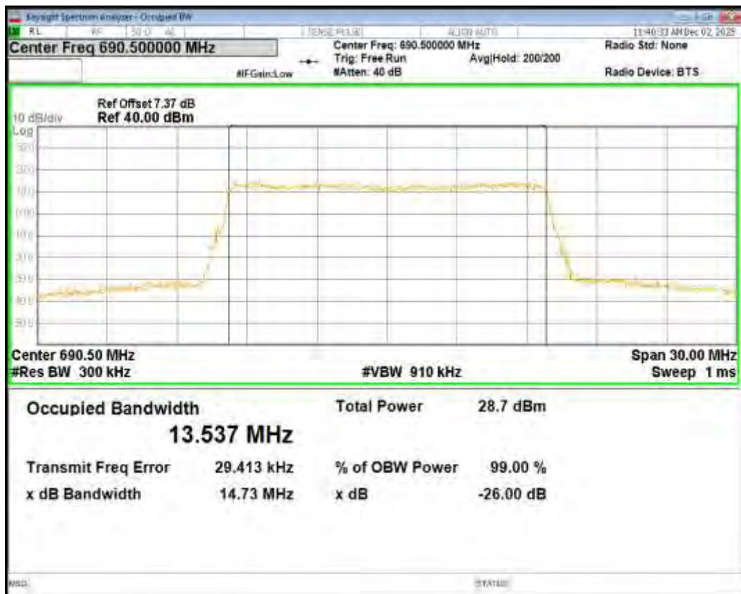
Band71 16QAM BW=20MHz Channel=133222 RB Size=100 Position=#0
