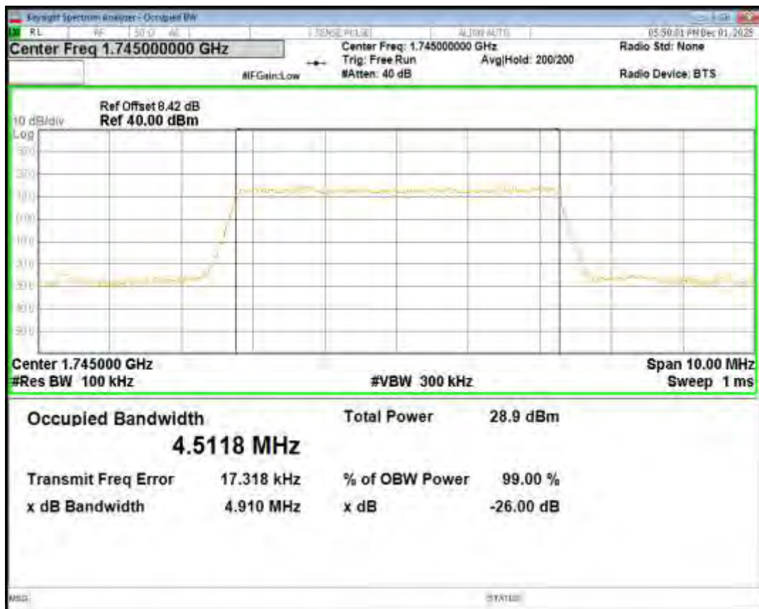
Band66 QPSK BW=3MHz Channel=132657 RB Size=15 Position=#0
