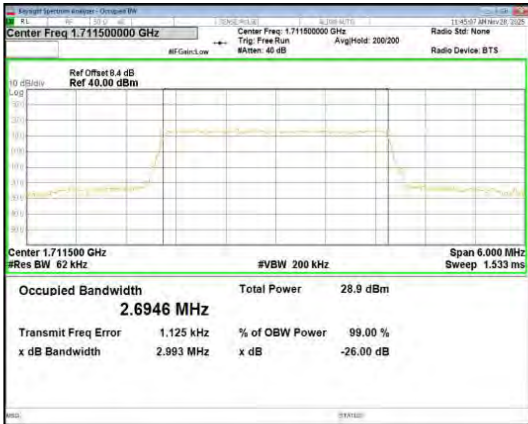
Band4 16QAM BW=5MHz Channel=20175 RB Size=25 Position=#0
