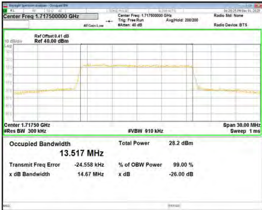
Band66 16QAM BW=15MHz Channel=132322 RB Size=75 Position=#0
