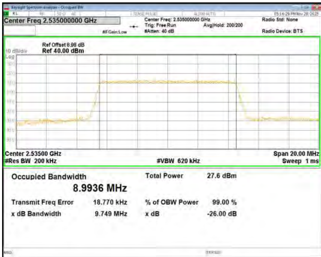
Band7 16QAM BW=10MHz Channel=21400 RB Size=50 Position=#0
