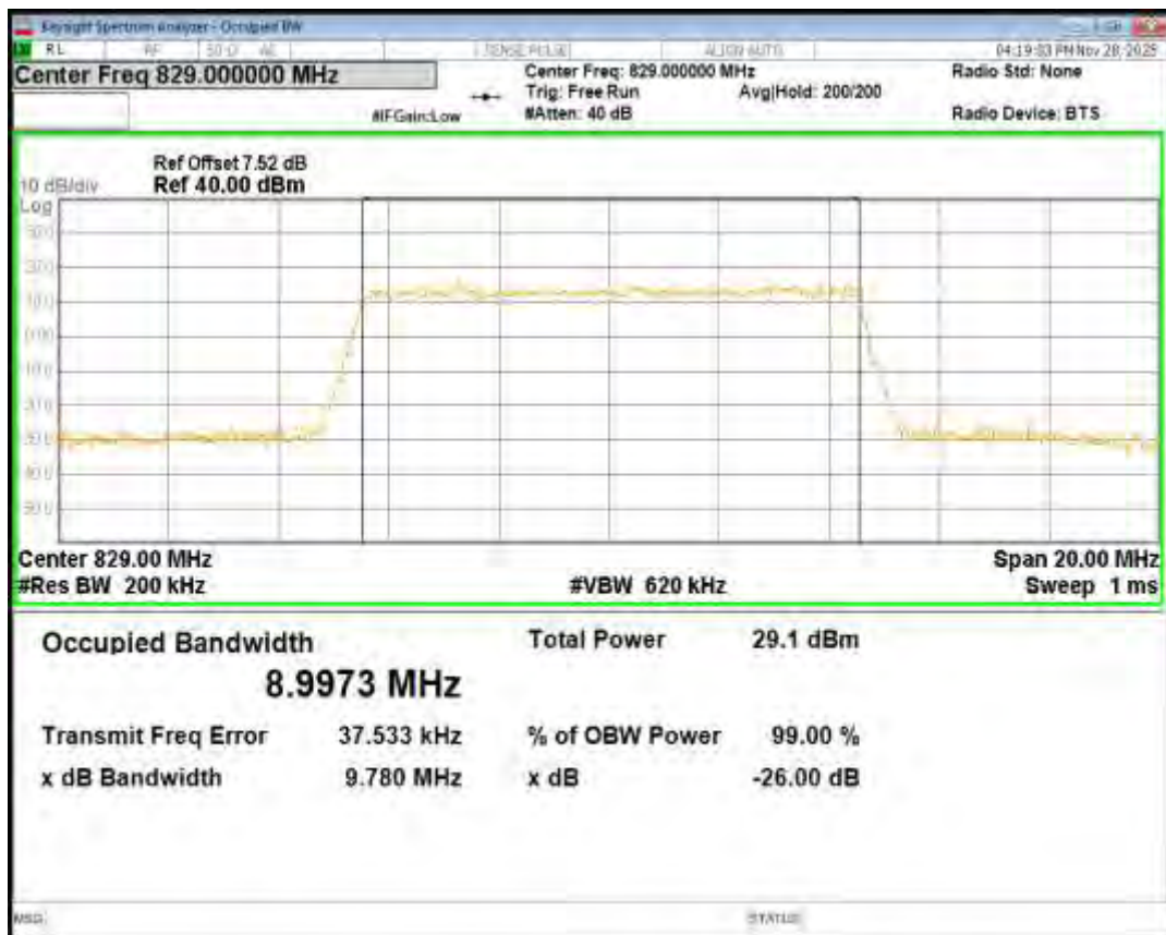
Band5 16QAM BW=10MHz Channel=20525 RB Size=50 Position=#0
