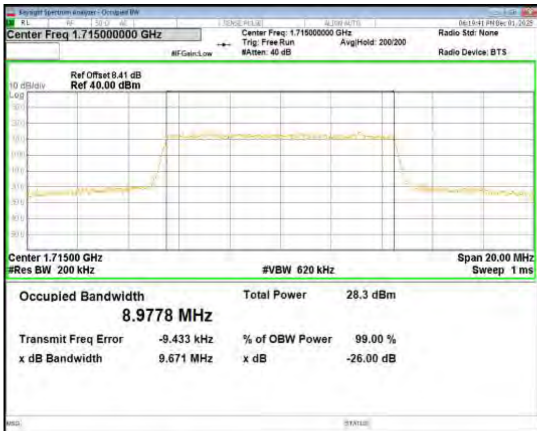
Band66 16QAM BW=10MHz Channel=132322 RB Size=50 Position=#0
