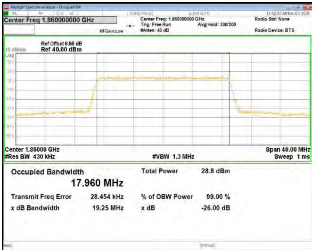
Band25 16QAM BW=10MHz Channel=26640 RB Size=50 Position=#0
