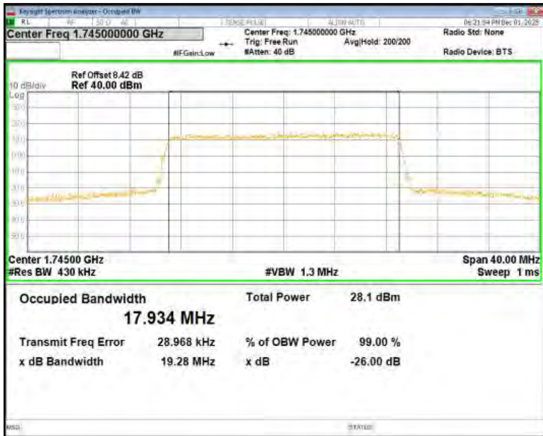
Band66 16QAM BW=20MHz Channel=132572 RB Size=100 Position=#0
