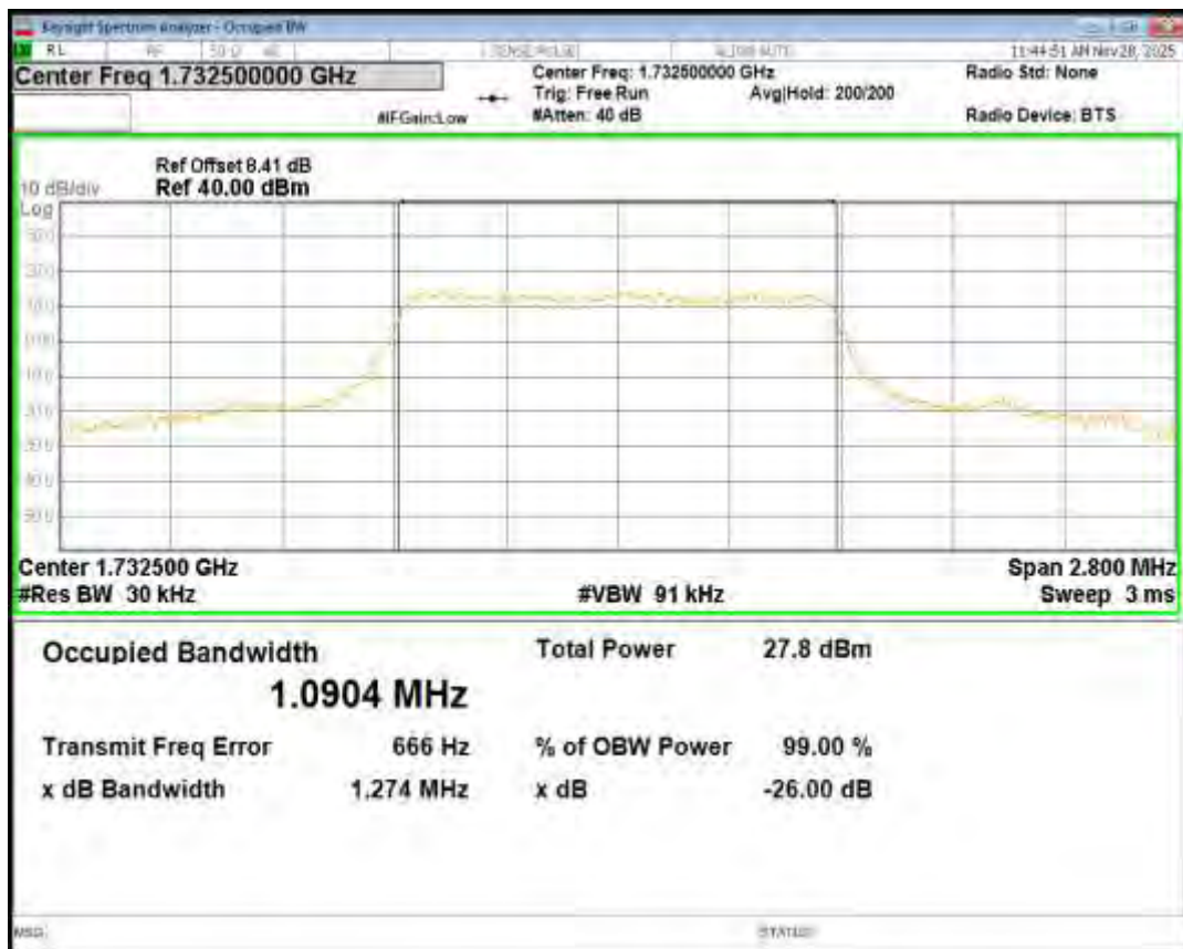
Band4 16QAM BW=1.4MHz Channel=20393 RB Size=6 Position=#0
