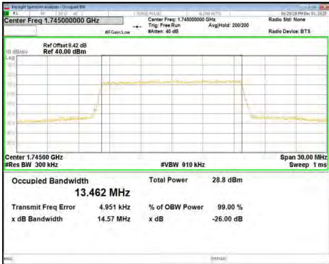
Band66 QPSK BW=20MHz Channel=132072 RB Size=100 Position=#0
