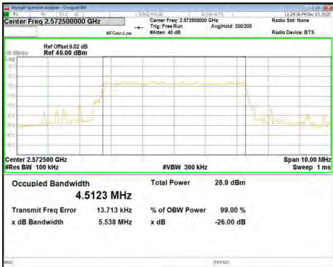
Band38 QPSK BW=5MHz Channel=38000 RB Size=25 Position=#0
