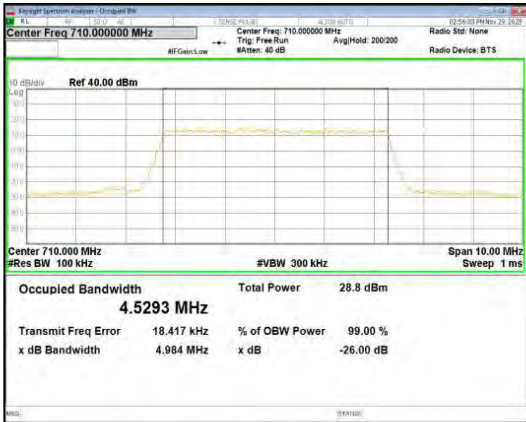
Band17 16QAM BW=5MHz Channel=23825 RB Size=25 Position=#0
