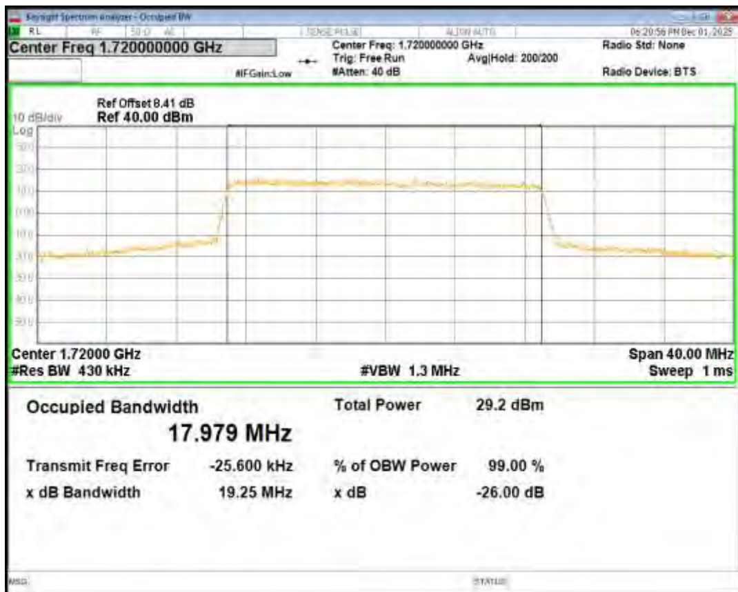
Band66 QPSK BW=20MHz Channel=132322 RB Size=100 Position=#0
