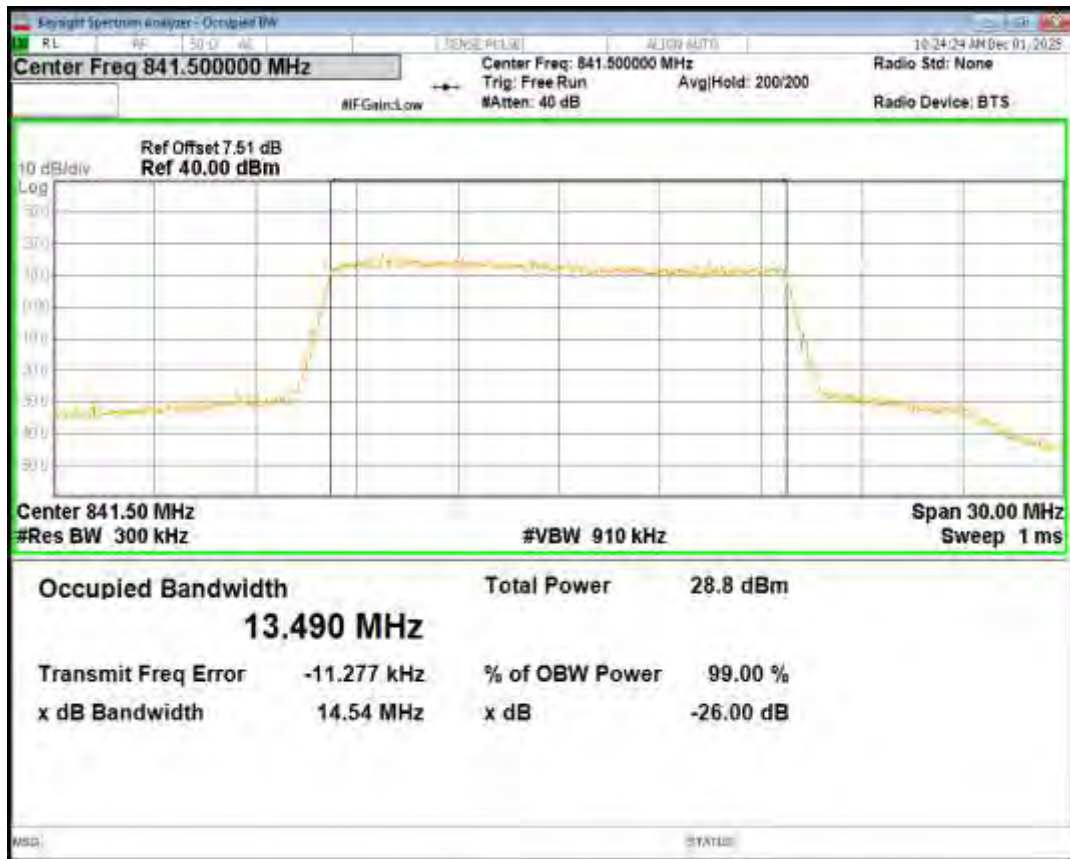
Band26(824-849) 16QAM BW=3MHz Channel=26805 RB Size=15 Position=#0
