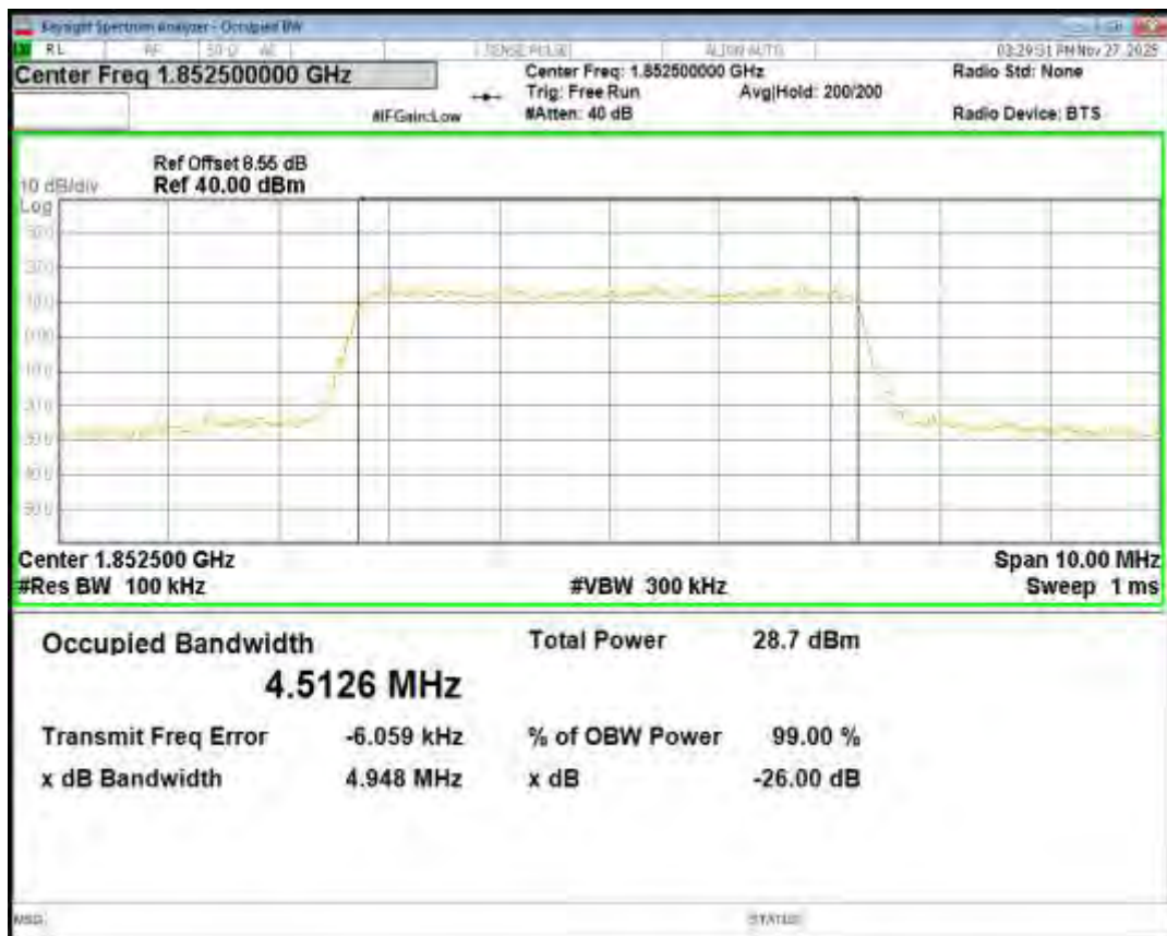
Band2 16QAM BW=20MHz Channel=19100 RB Size=100 Position=#0
