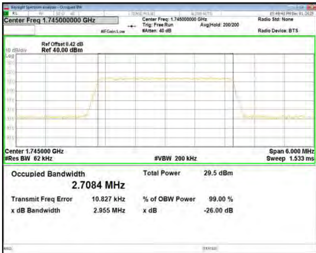
Band66 QPSK BW=5MHz Channel=131997 RB Size=25 Position=#0
