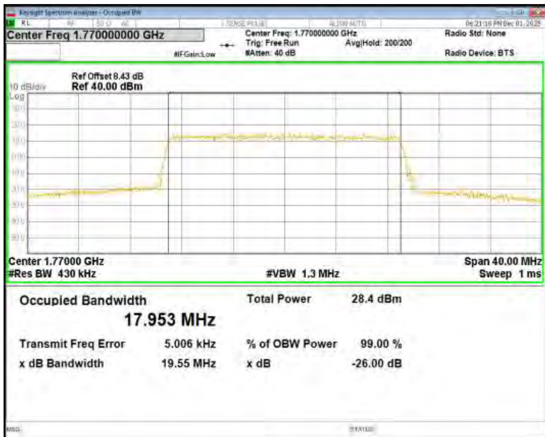
Band66 16QAM BW=3MHz Channel=131987 RB Size=15 Position=#0
