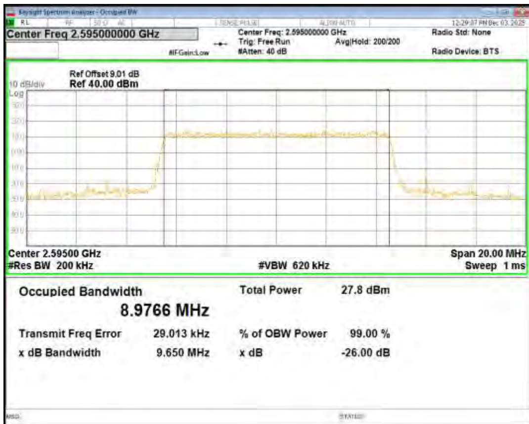
Band38 16QAM BW=10MHz Channel=38200 RB Size=50 Position=#0
