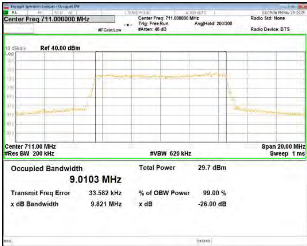
Band17 QPSK BW=5MHz Channel=23755 RB Size=25 Position=#0
