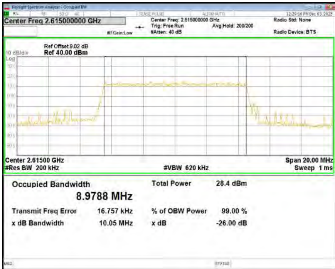
Band38 QPSK BW=15MHz Channel=37825 RB Size=75 Position=#0
