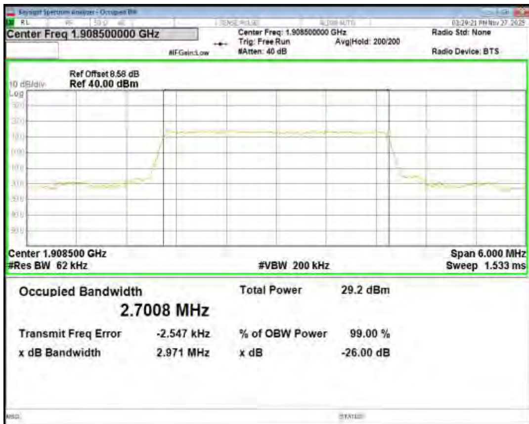
Band2 16QAM BW=5MHz Channel=18900 RB Size=25 Position=#0
