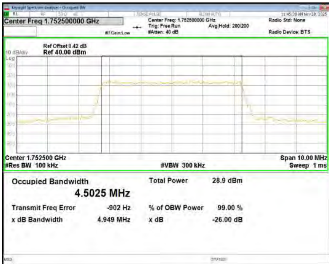
Band40(2305-2315) 16QAM BW=10MHz Channel=38750 RB Size=50 Position=#0
