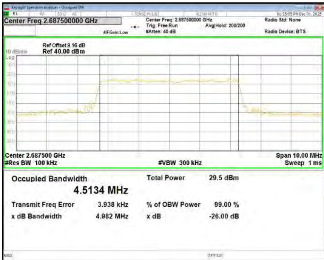
Band41 QPSK BW=10MHz Channel=39700 RB Size=50 Position=#0
