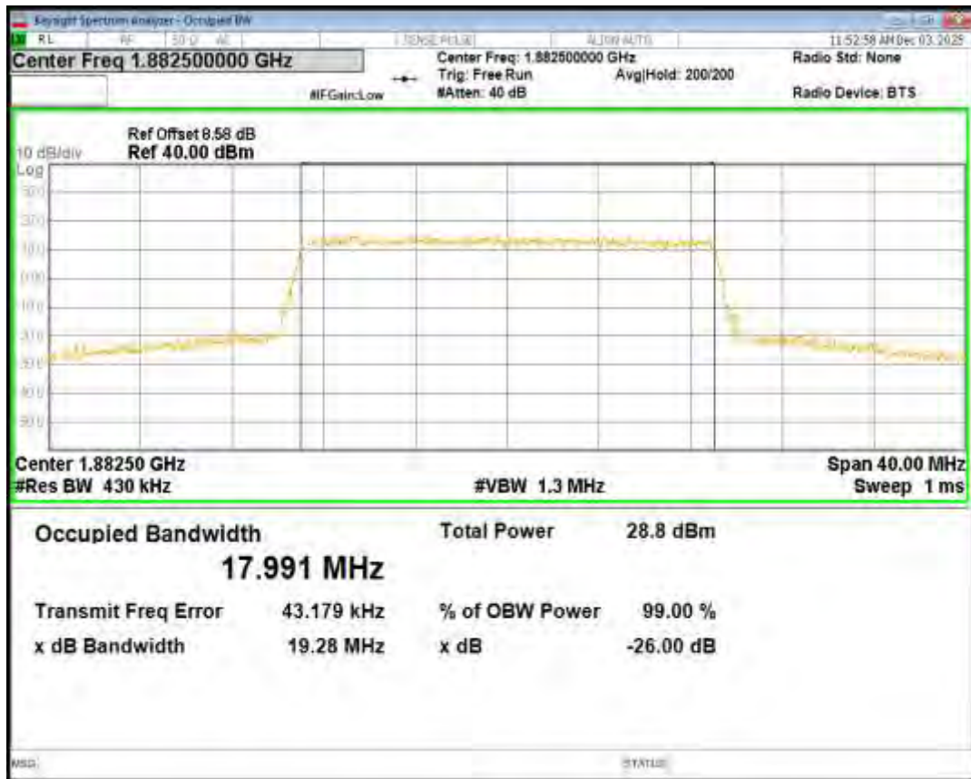
Band25 16QAM BW=20MHz Channel=26590 RB Size=100 Position=#0
