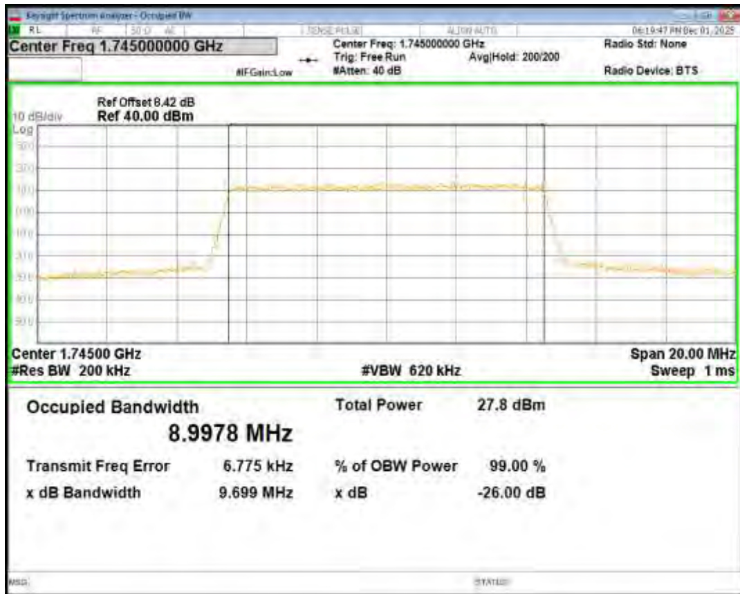
Band66 16QAM BW=10MHz Channel=132622 RB Size=50 Position=#0
