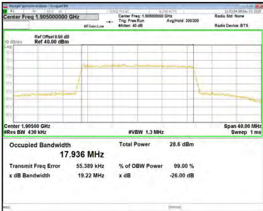
Band25 16QAM BW=3MHz Channel=26055 RB Size=15 Position=#0
