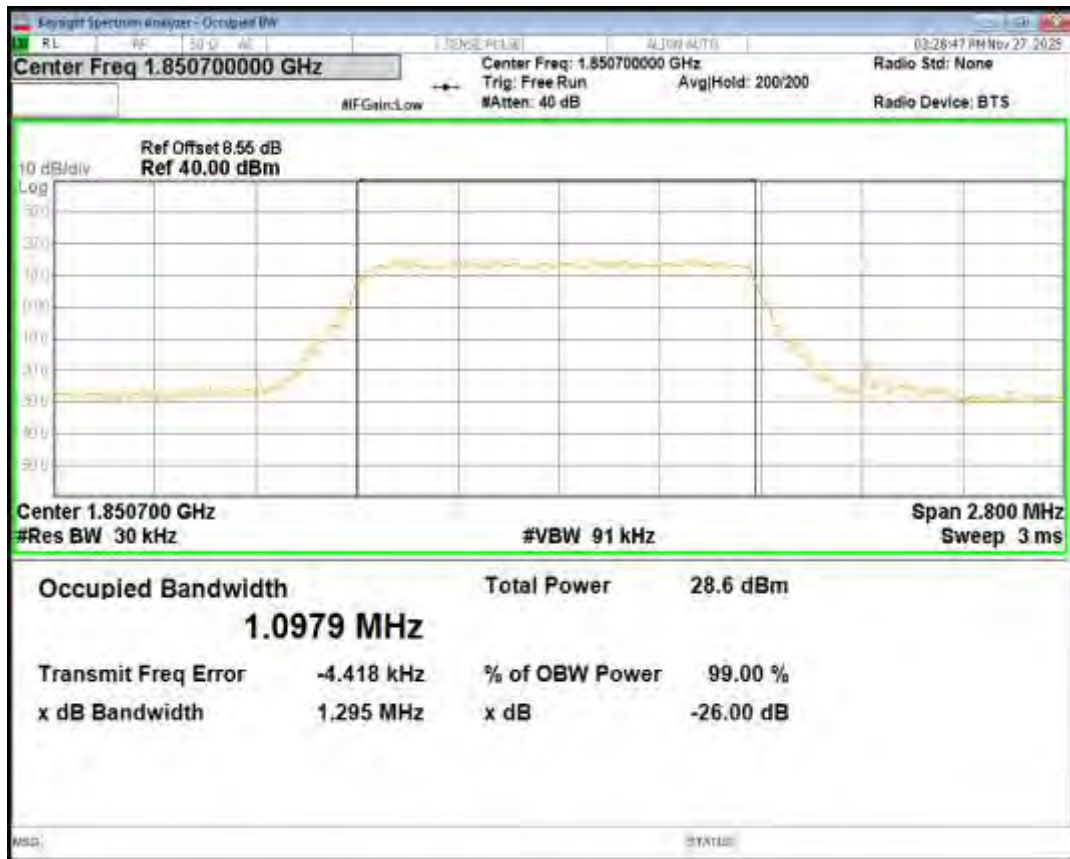
Band2 16QAM BW=1.4MHz Channel=18900 RB Size=6 Position=#0
