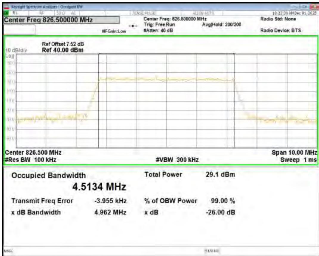
Band26(824-849) QPSK BW=1.4MHz Channel=27033 RB Size=6 Position=#0
