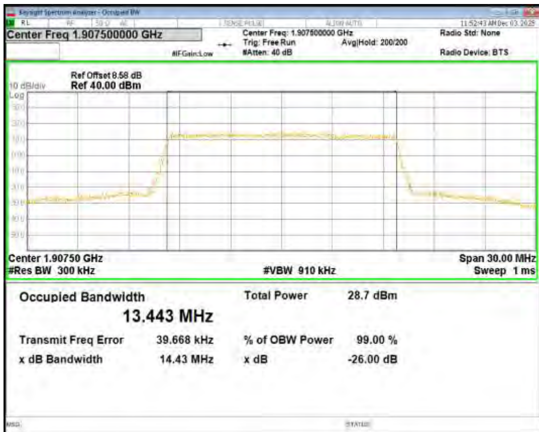
Band25 16QAM BW=15MHz Channel=26365 RB Size=75 Position=#0
