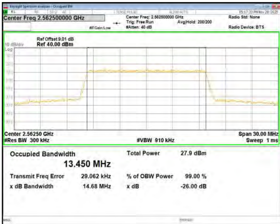
Band7 16QAM BW=20MHz Channel=20850 RB Size=100 Position=#0
