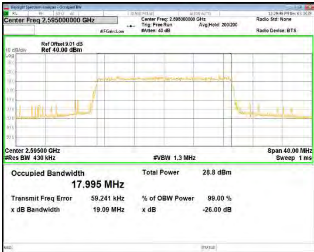
Band38 QPSK BW=20MHz Channel=38150 RB Size=100 Position=#0
