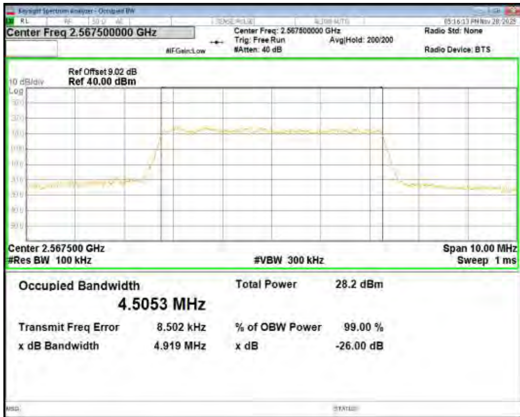
Band7 16QAM BW=5MHz Channel=21100 RB Size=25 Position=#0
