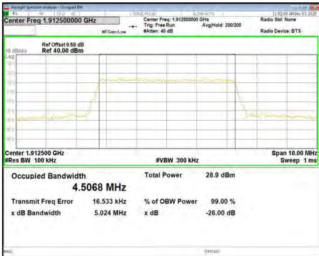
Band25 16QAM BW=5MHz Channel=26365 RB Size=25 Position=#0
