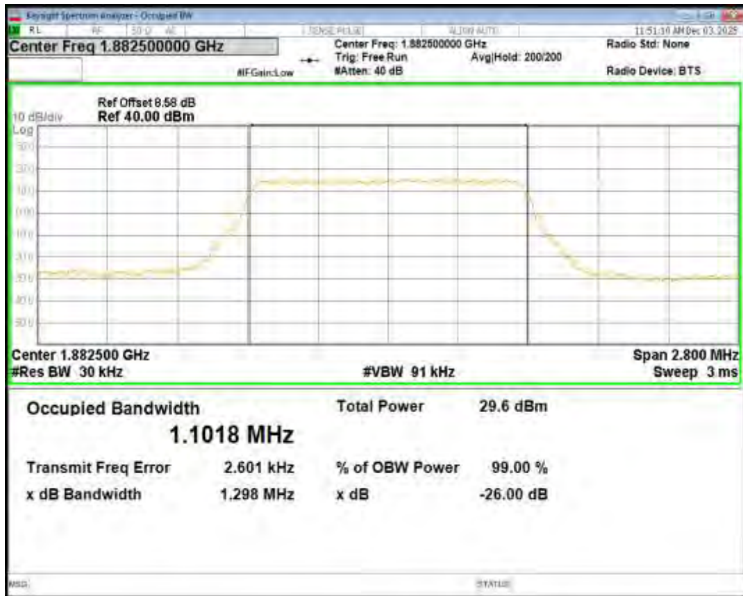
Band25 16QAM BW=5MHz Channel=26665 RB Size=25 Position=#0
