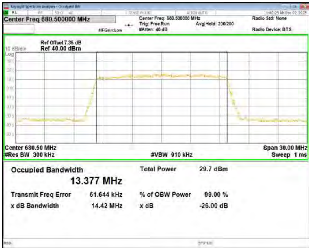
Band71 QPSK BW=15MHz Channel=133397 RB Size=75 Position=#0
