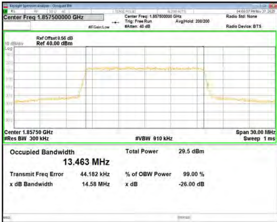
Band2 QPSK BW=10MHz Channel=19150 RB Size=50 Position=#0
