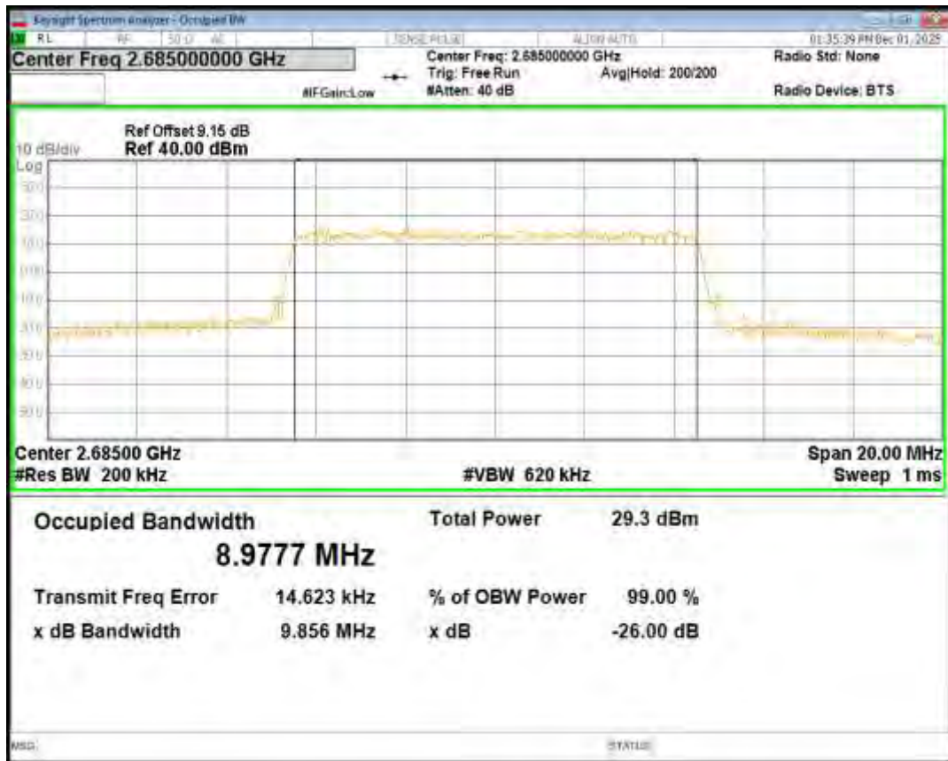
Band41 16QAM BW=15MHz Channel=39725 RB Size=75 Position=#0
