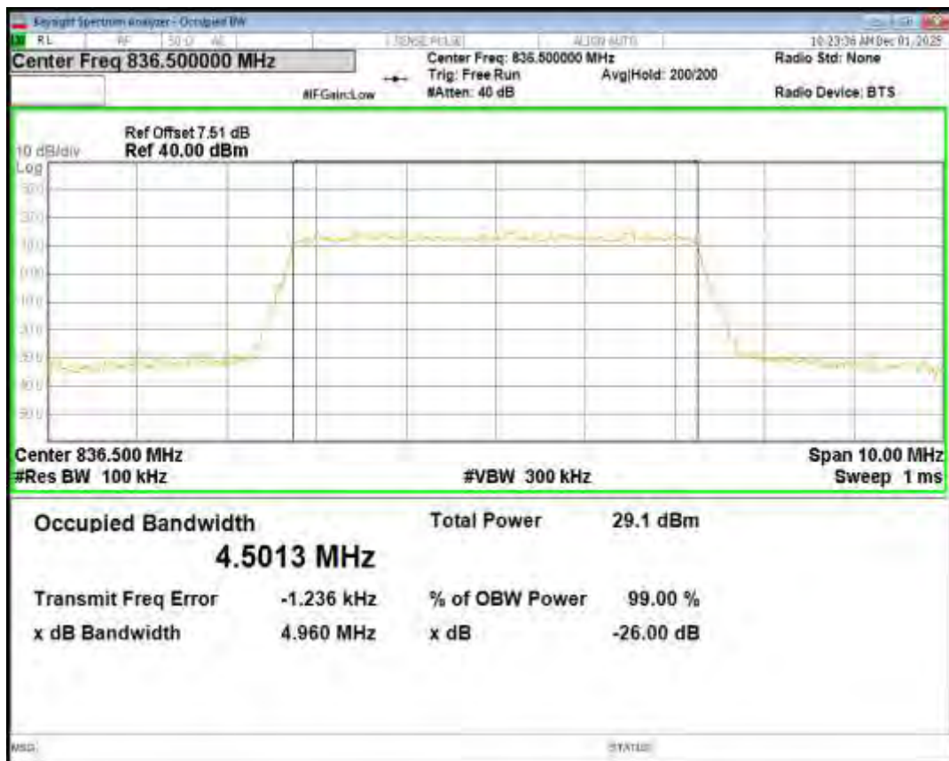
Band26(824-849) 16QAM BW=5MHz Channel=26815 RB Size=25 Position=#0
