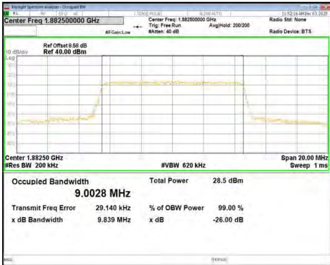
Band25 16QAM BW=15MHz Channel=26615 RB Size=75 Position=#0
