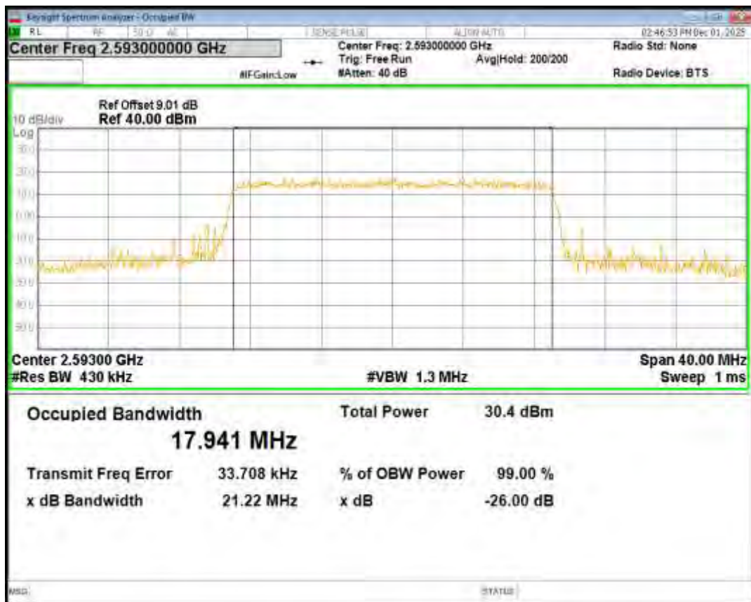
Band41 16QAM BW=20MHz Channel=41490 RB Size=100 Position=#0
