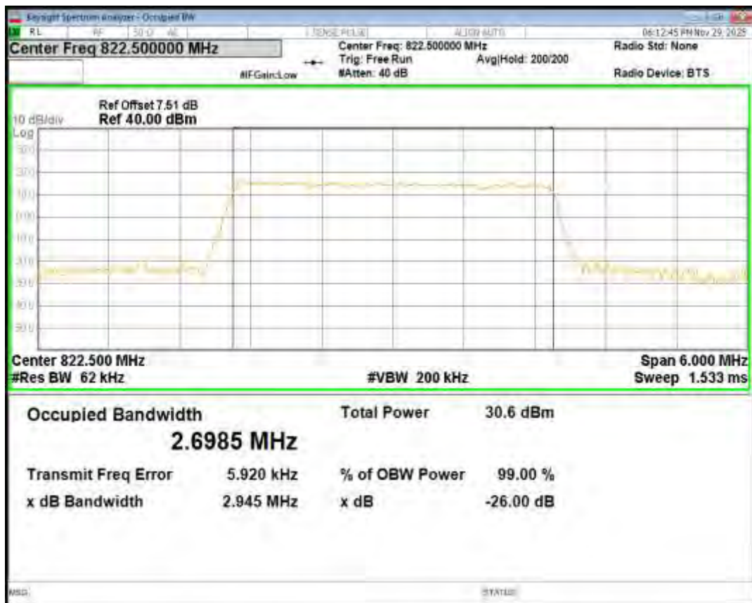
Band26(814-824) QPSK BW=5MHz Channel=26715 RB Size=25 Position=#0
