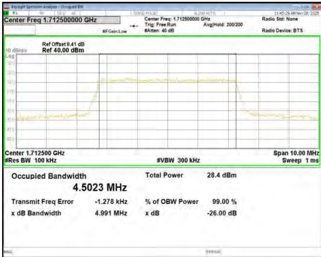
Band4 16QAM BW=5MHz Channel=20375 RB Size=25 Position=#0
