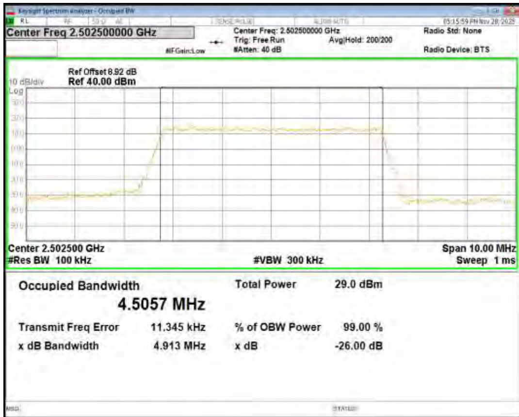
Band7 QPSK BW=5MHz Channel=21425 RB Size=25 Position=#0
