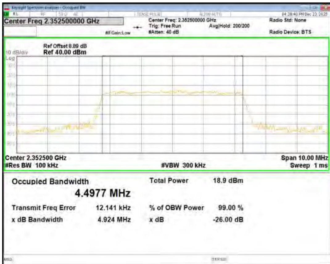
Band40(2350-2360) 16QAM BW=5MHz Channel=39200 RB Size=25 Position=#0
