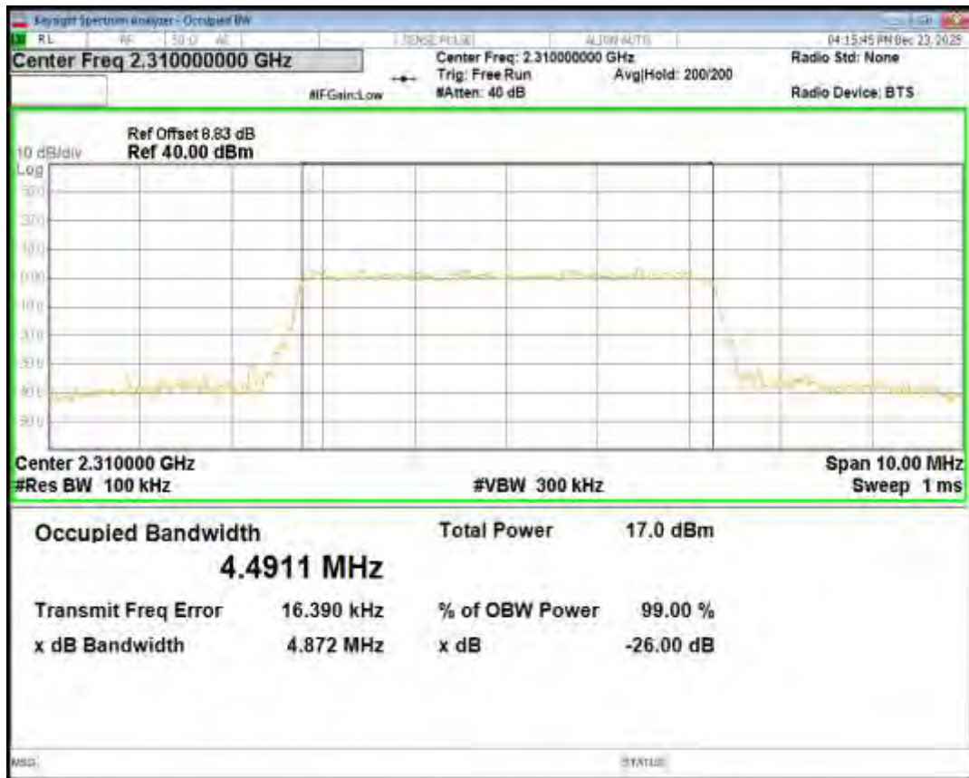
Band40(2305-2315) QPSK BW=5MHz Channel=38775 RB Size=25 Position=#0
