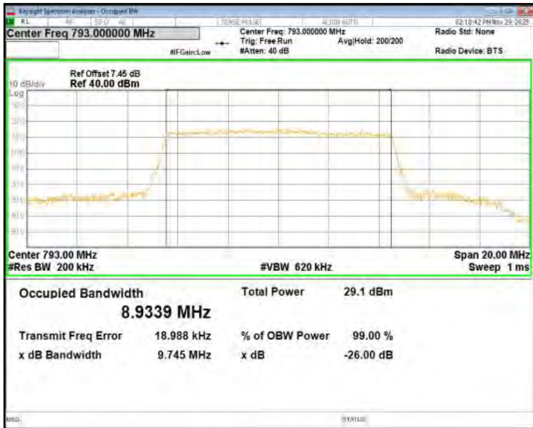
Band14 16QAM BW=5MHz Channel=23305 RB Size=25 Position=#0
