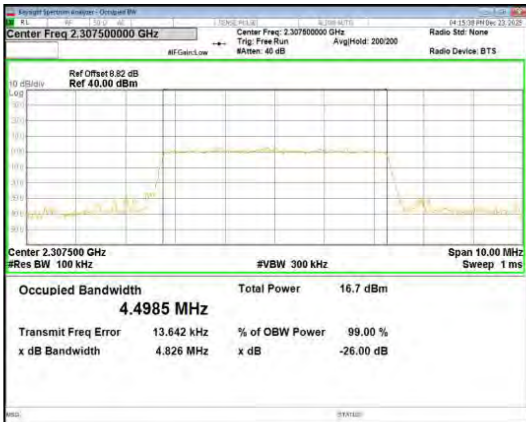
Band40(2305-2315) QPSK BW=5MHz Channel=38750 RB Size=25 Position=#0
