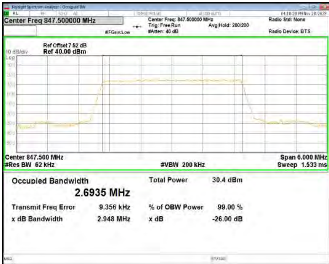
Band5 QPSK BW=5MHz Channel=20425 RB Size=25 Position=#0
