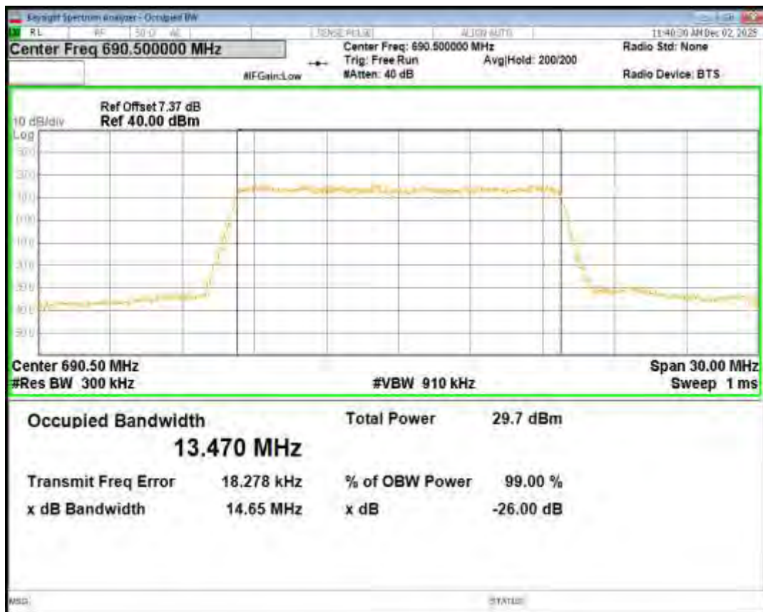
Band71 QPSK BW=20MHz Channel=133222 RB Size=100 Position=#0
