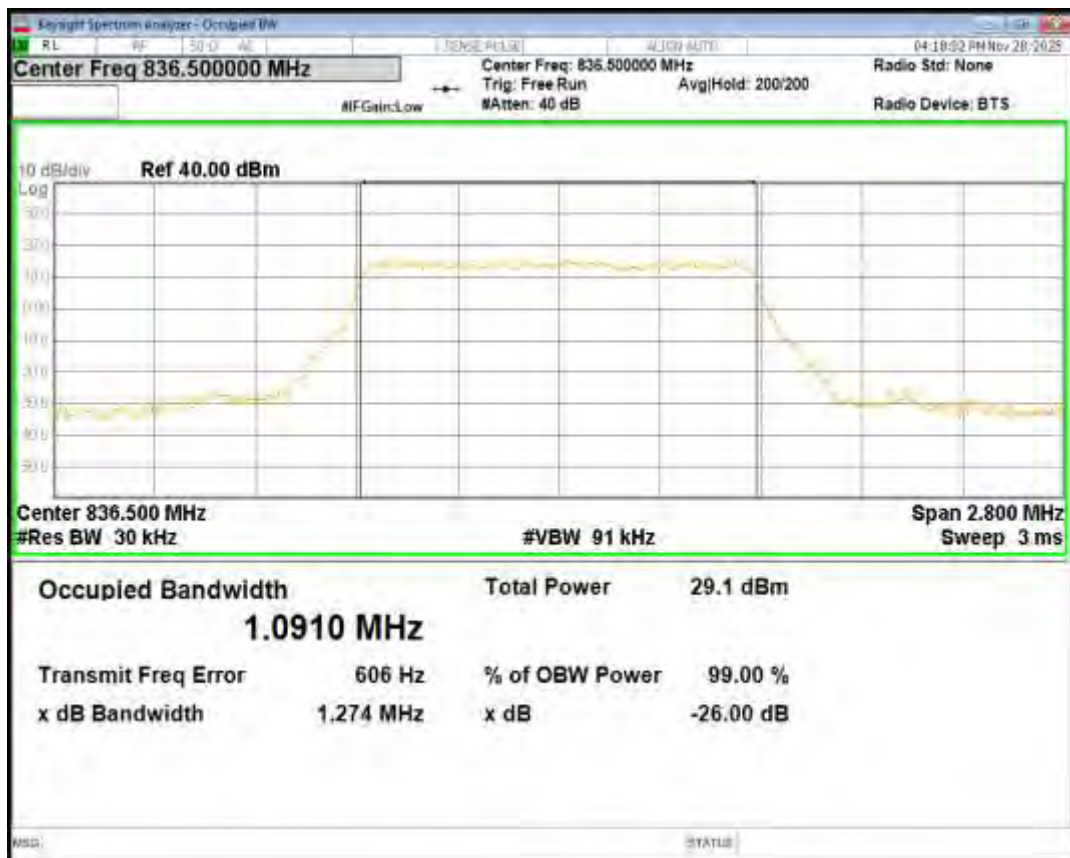
Band5 16QAM BW=1.4MHz Channel=20643 RB Size=6 Position=#0
