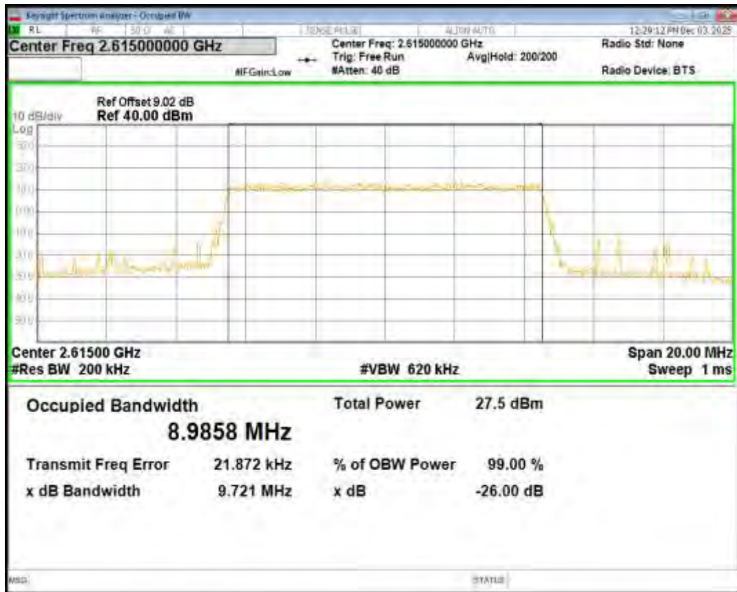
Band38 16QAM BW=15MHz Channel=37825 RB Size=75 Position=#0
