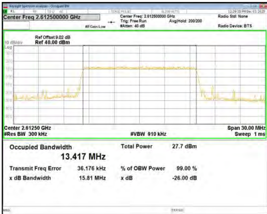
Band38 16QAM BW=20MHz Channel=37850 RB Size=100 Position=#0
