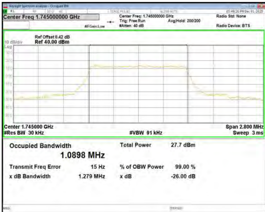
Band66 16QAM BW=1.4MHz Channel=132665 RB Size=6 Position=#0
