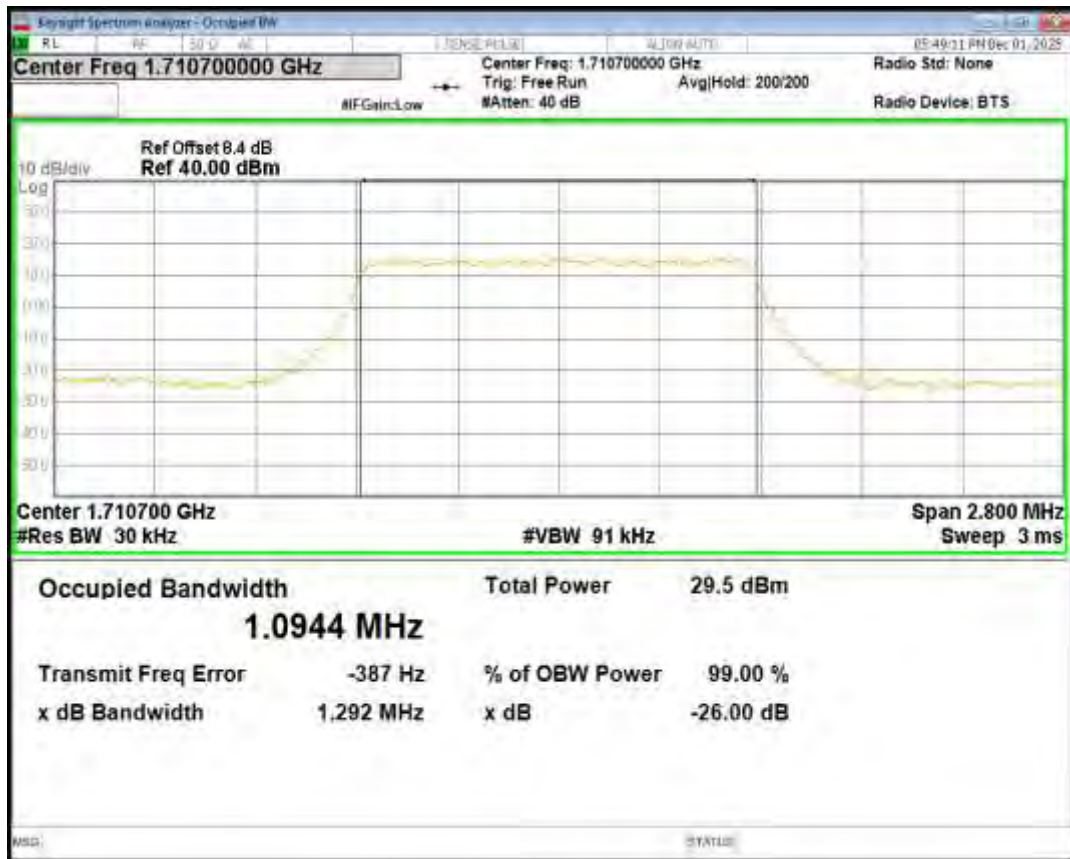
Band66 QPSK BW=1.4MHz Channel=132322 RB Size=6 Position=#0
