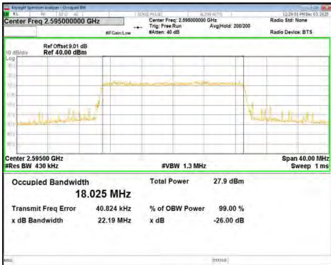
Band38 16QAM BW=20MHz Channel=38150 RB Size=100 Position=#0
