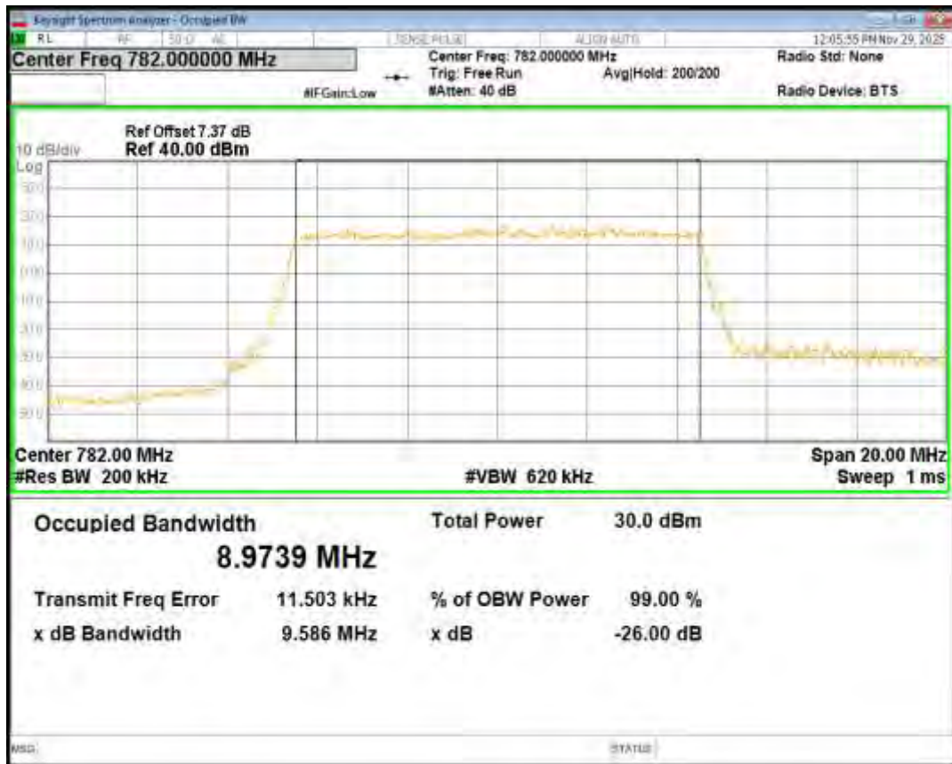
Band13 QPSK BW=5MHz Channel=23205 RB Size=25 Position=#0
