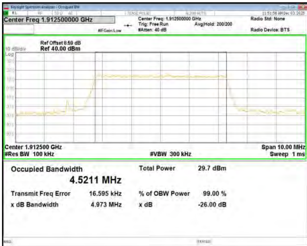
Band26(814-824) 16QAM BW=1.4MHz Channel=26697 RB Size=6 Position=#0
