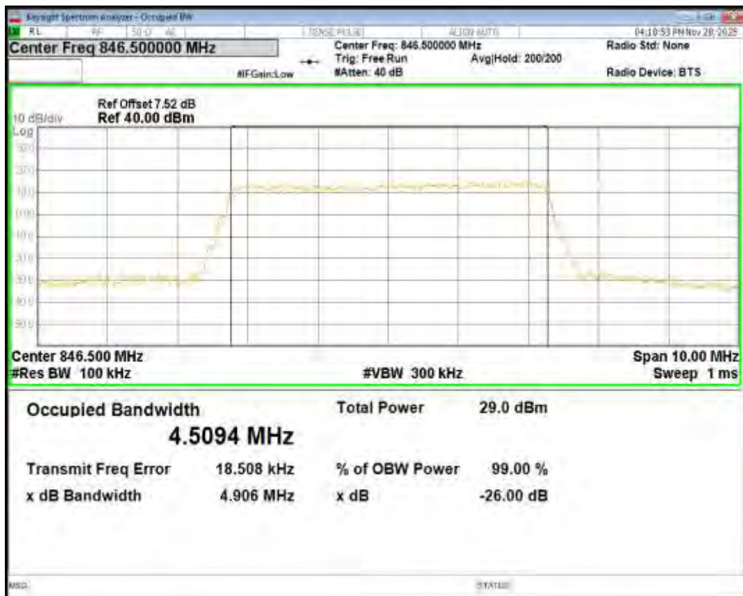
Band5 16QAM BW=3MHz Channel=20635 RB Size=15 Position=#0
