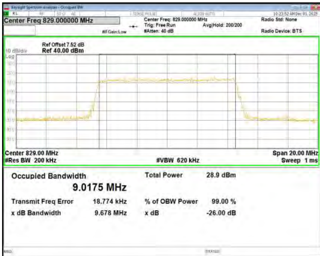
Band26(824-849) 16QAM BW=10MHz Channel=26915 RB Size=50 Position=#0
