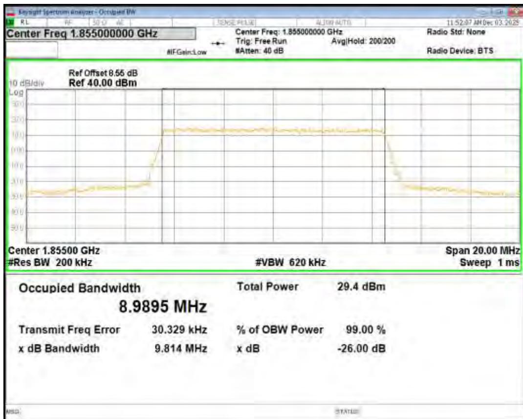
Band25 QPSK BW=1.4MHz Channel=26365 RB Size=6 Position=#0
