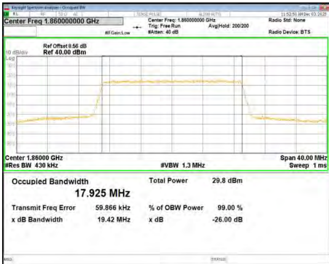
Band25 QPSK BW=20MHz Channel=26365 RB Size=100 Position=#0
