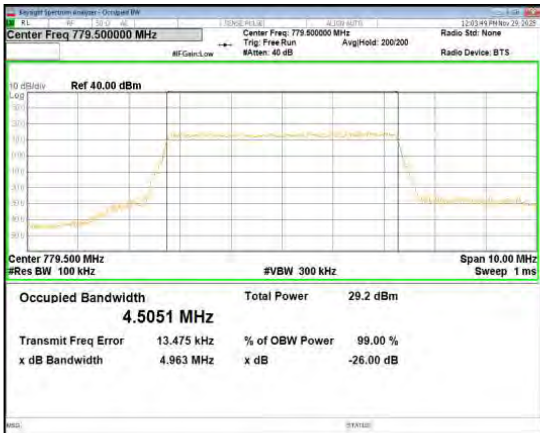
Band13 16QAM BW=5MHz Channel=23230 RB Size=25 Position=#0
