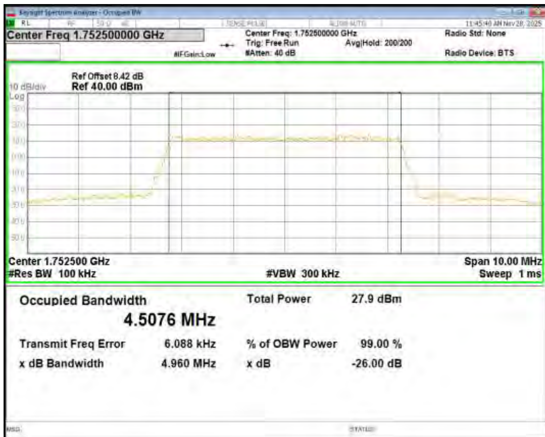
Band4 16QAM BW=3MHz Channel=20175 RB Size=15 Position=#0
