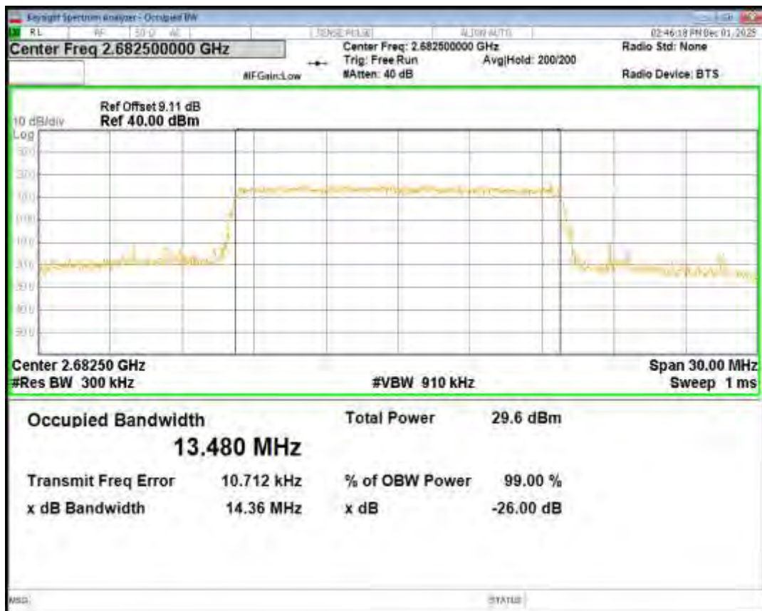
Band41 16QAM BW=20MHz Channel=39750 RB Size=100 Position=#0
