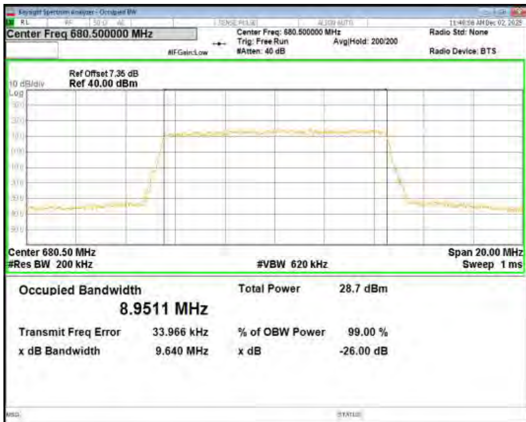
Band71 16QAM BW=10MHz Channel=133422 RB Size=50 Position=#0
