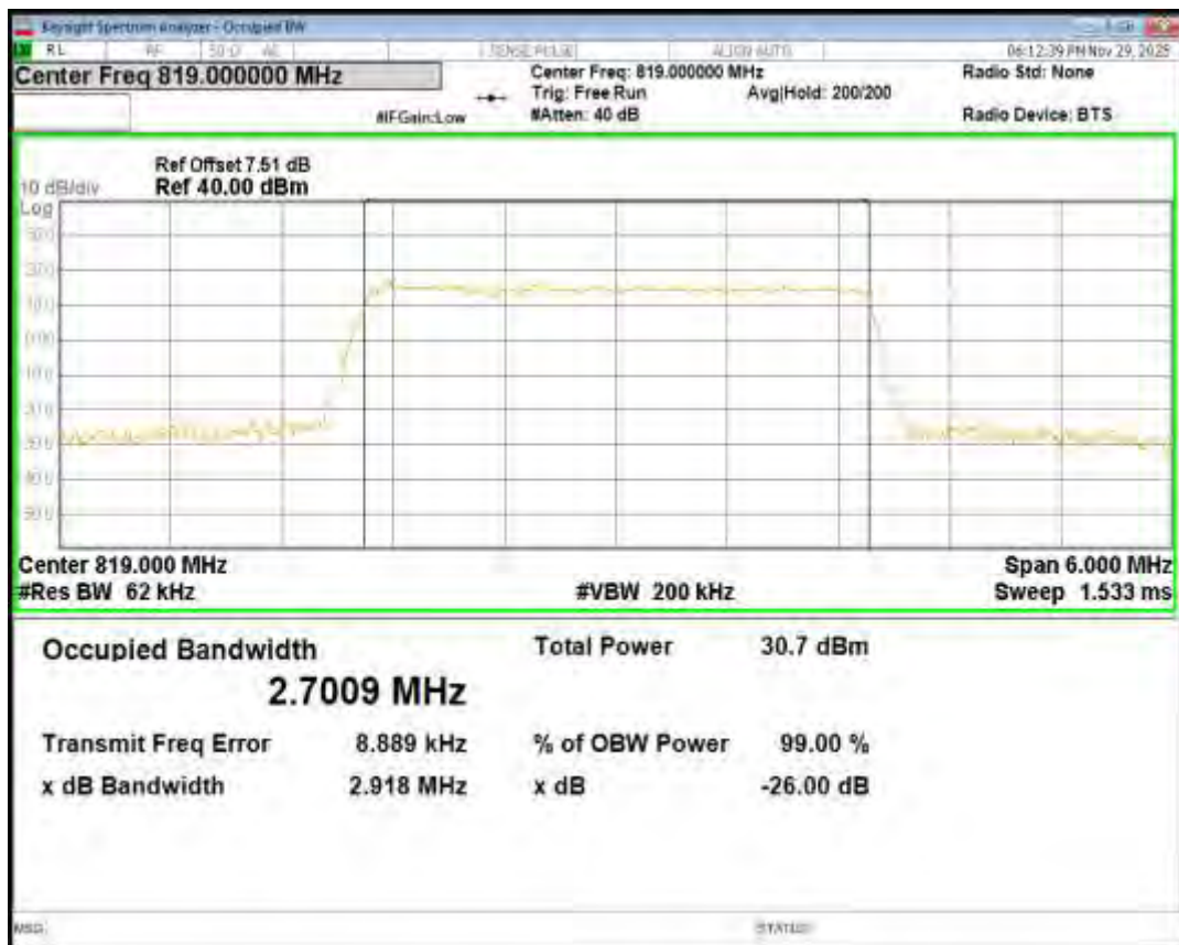
Band26(814-824) QPSK BW=5MHz Channel=26740 RB Size=25 Position=#0
