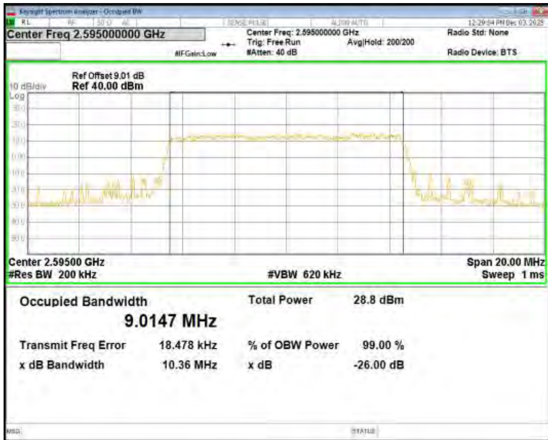
Band38 QPSK BW=10MHz Channel=37800 RB Size=50 Position=#0
