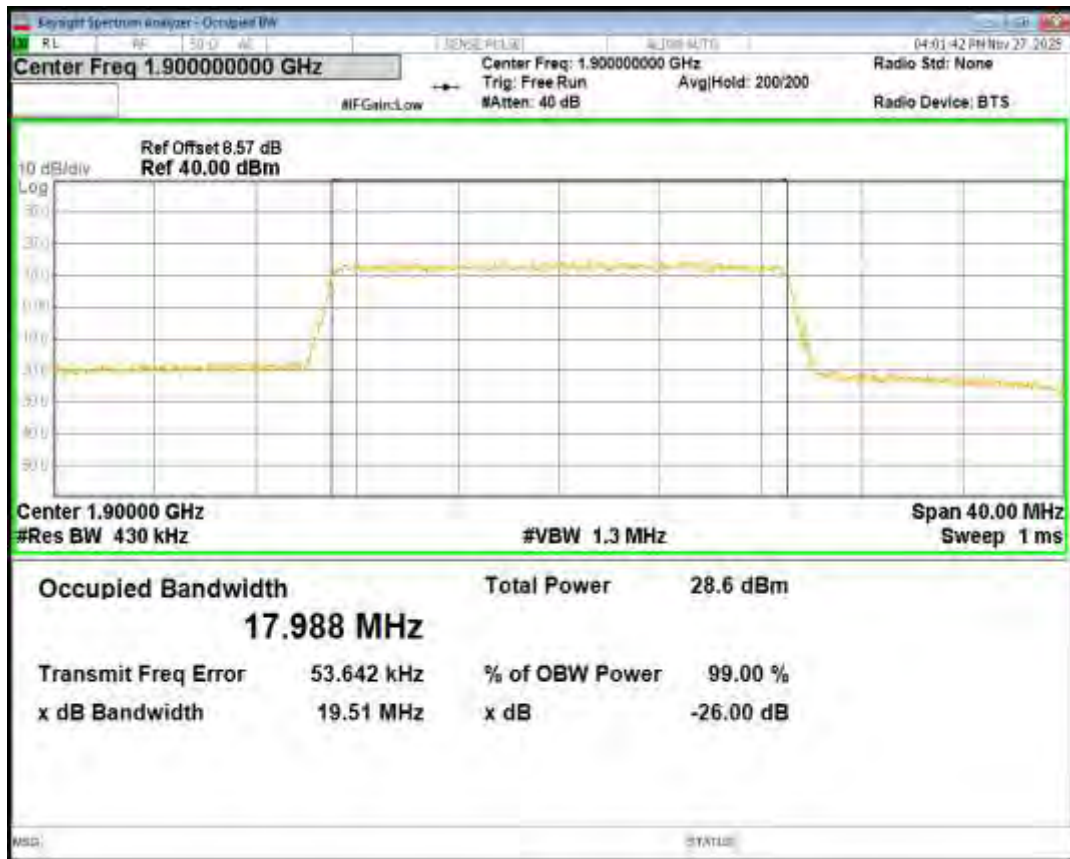
Band2 16QAM BW=3MHz Channel=18615 RB Size=15 Position=#0
