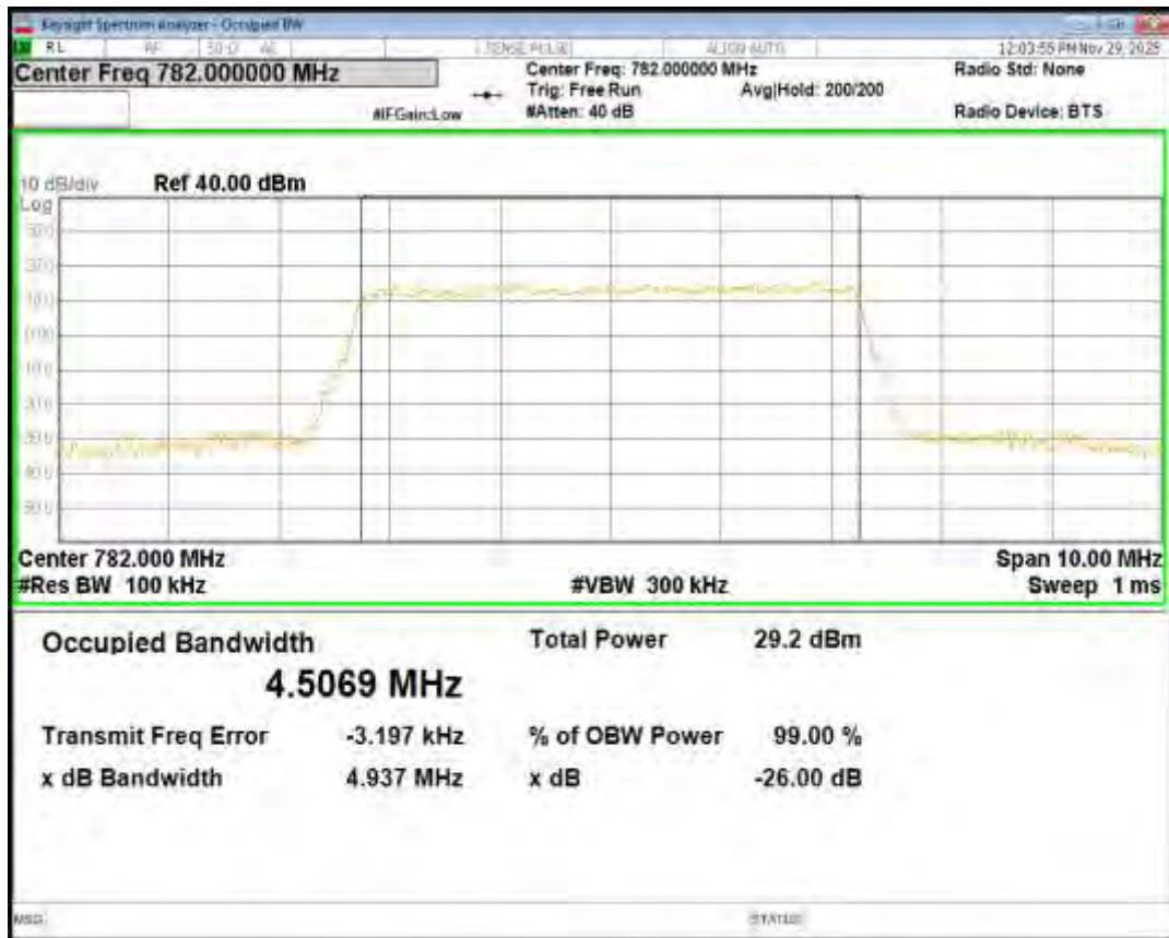
Band13 16QAM BW=5MHz Channel=23255 RB Size=25 Position=#0
