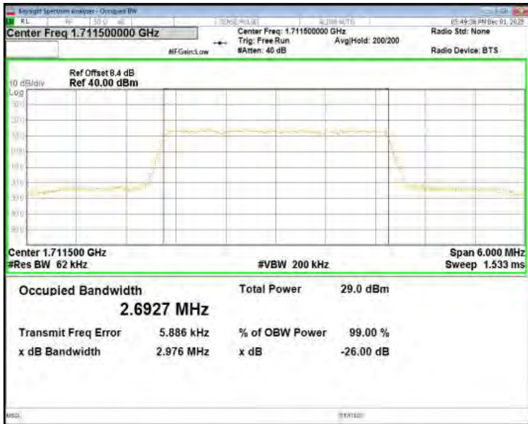
Band66 16QAM BW=3MHz Channel=132322 RB Size=15 Position=#0
