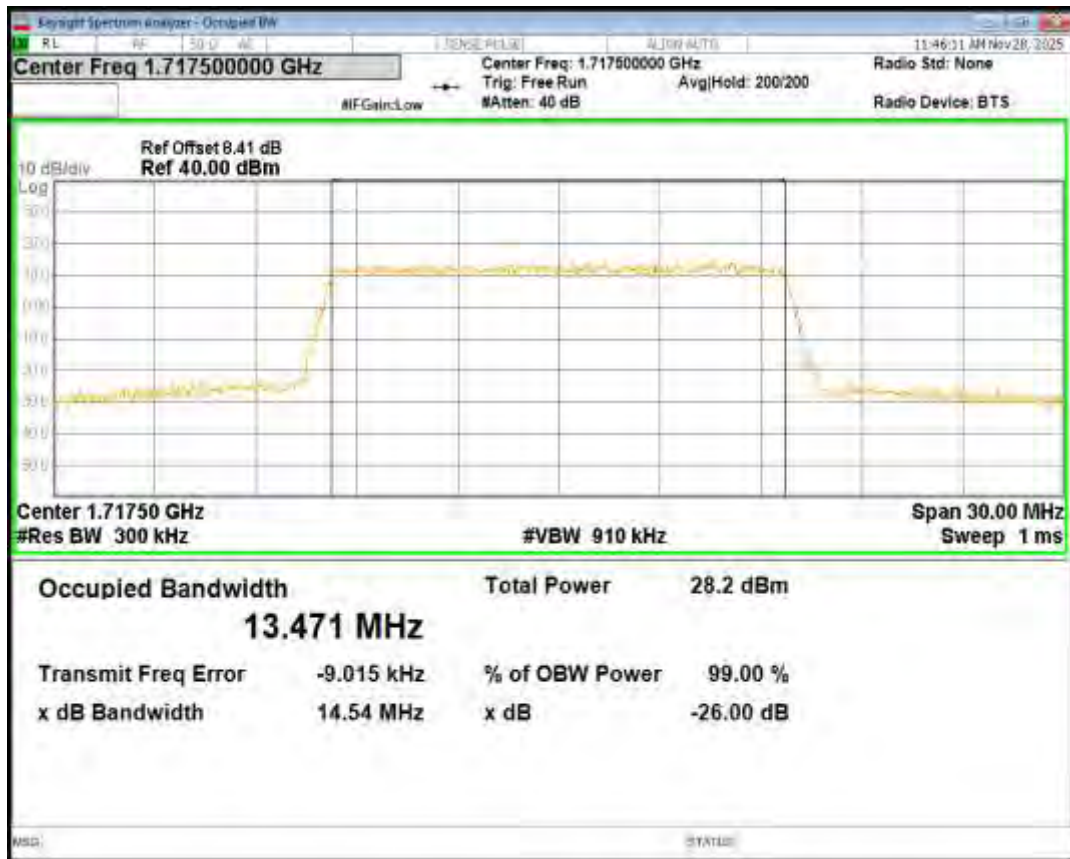
Band4 16QAM BW=15MHz Channel=20175 RB Size=75 Position=#0
