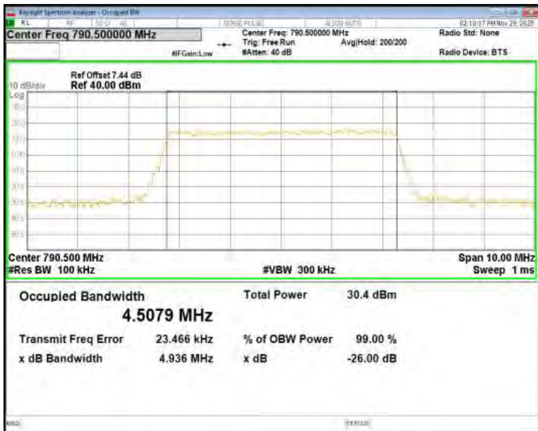
Band14 QPSK BW=5MHz Channel=23330 RB Size=25 Position=#0
