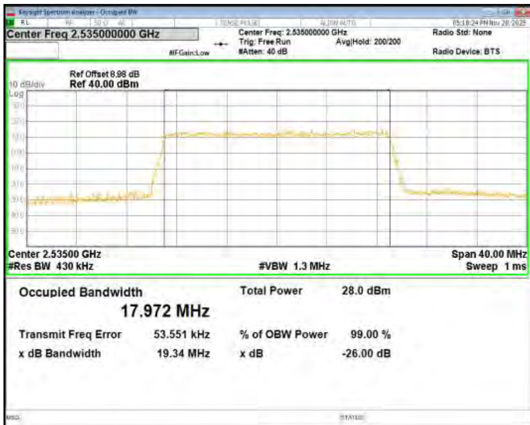
Band7 16QAM BW=20MHz Channel=21350 RB Size=100 Position=#0
