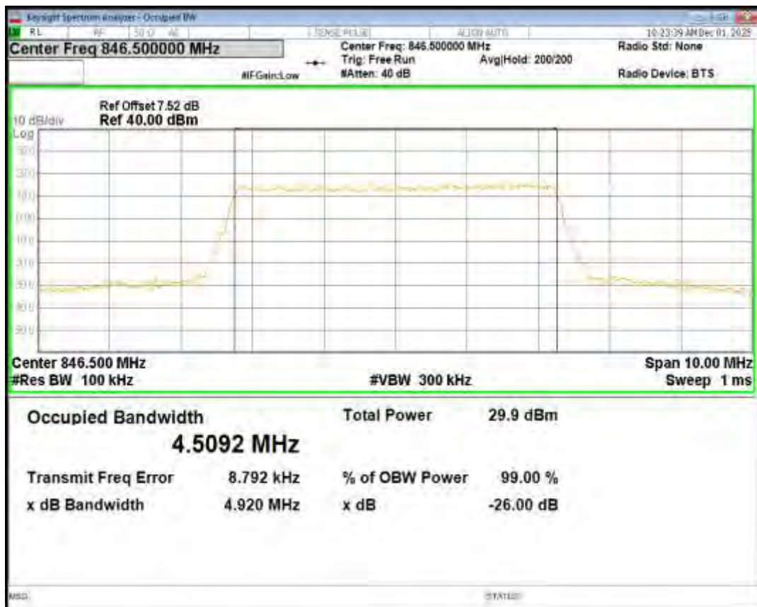
Band38 16QAM BW=10MHz Channel=37800 RB Size=50 Position=#0
