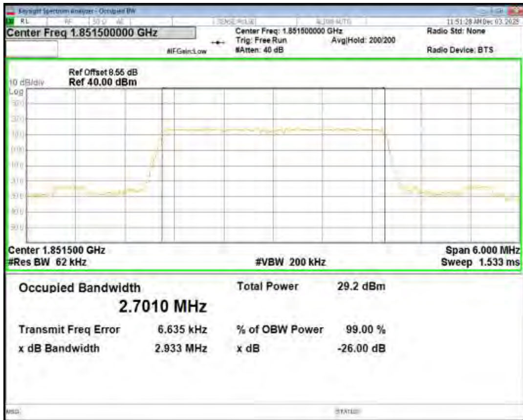
Band25 16QAM BW=3MHz Channel=26365 RB Size=15 Position=#0
