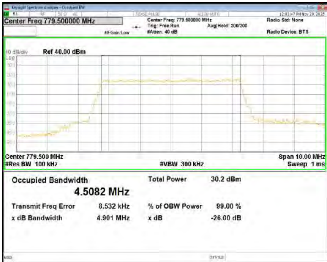
Band13 QPSK BW=5MHz Channel=23230 RB Size=25 Position=#0
