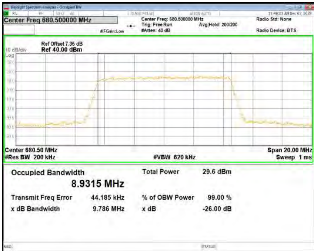
Band71 16QAM BW=5MHz Channel=133447 RB Size=25 Position=#0
