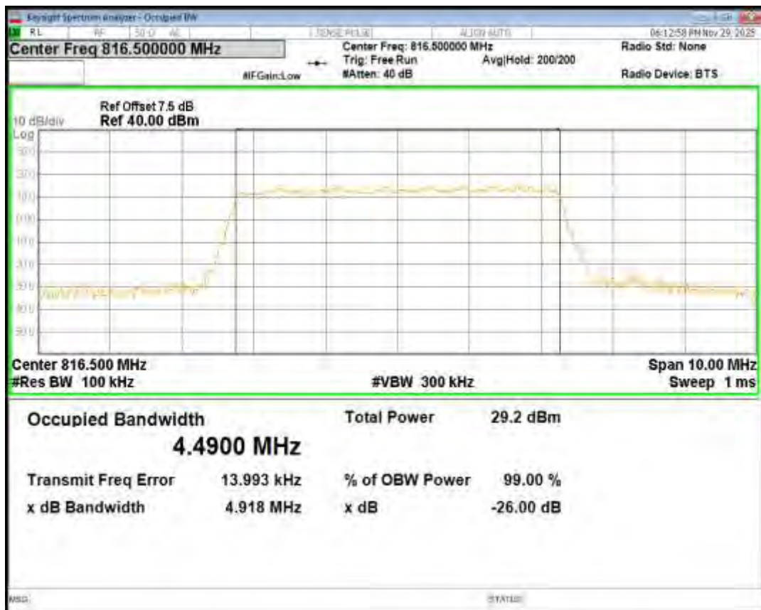
Band26(814-824) 16QAM BW=5MHz Channel=26765 RB Size=25 Position=#0
