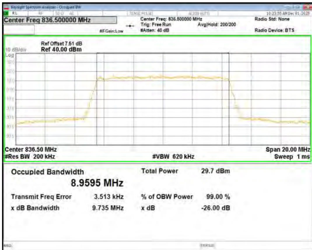
Band26(824-849) QPSK BW=10MHz Channel=26990 RB Size=50 Position=#0
