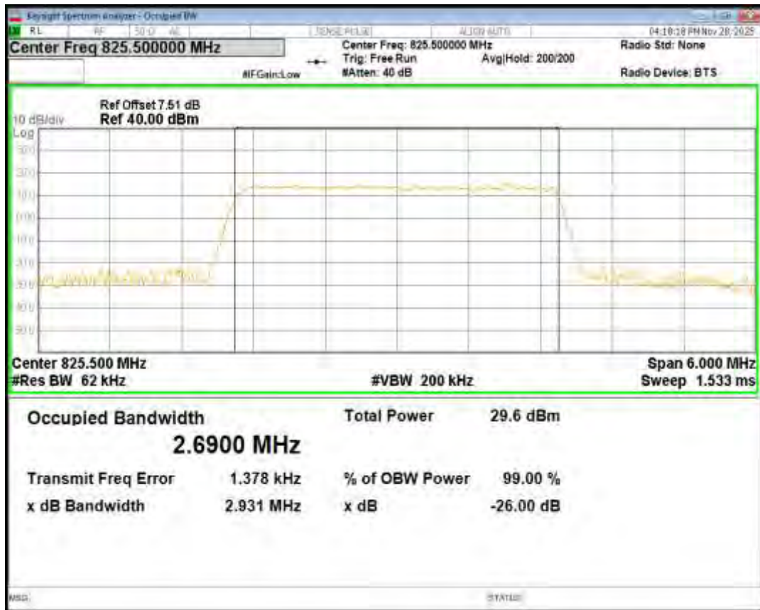
Band5 16QAM BW=3MHz Channel=20525 RB Size=15 Position=#0
