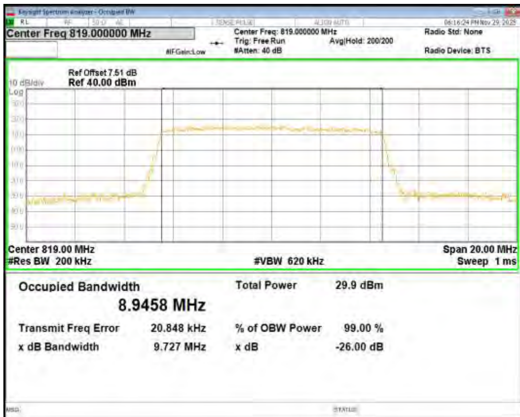
Band26(814-824) QPSK BW=3MHz Channel=26705 RB Size=15 Position=#0
