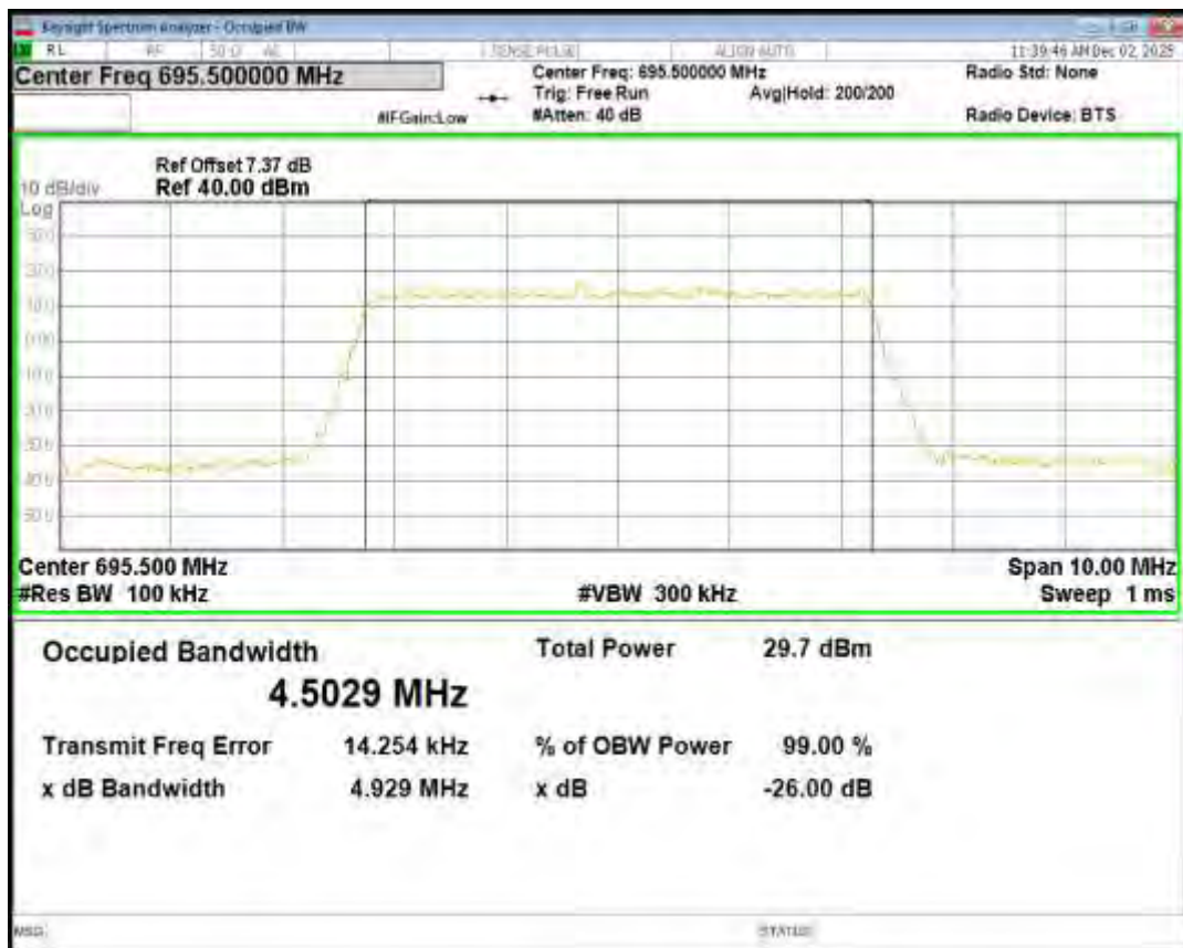
Band71 QPSK BW=5MHz Channel=133447 RB Size=25 Position=#0
