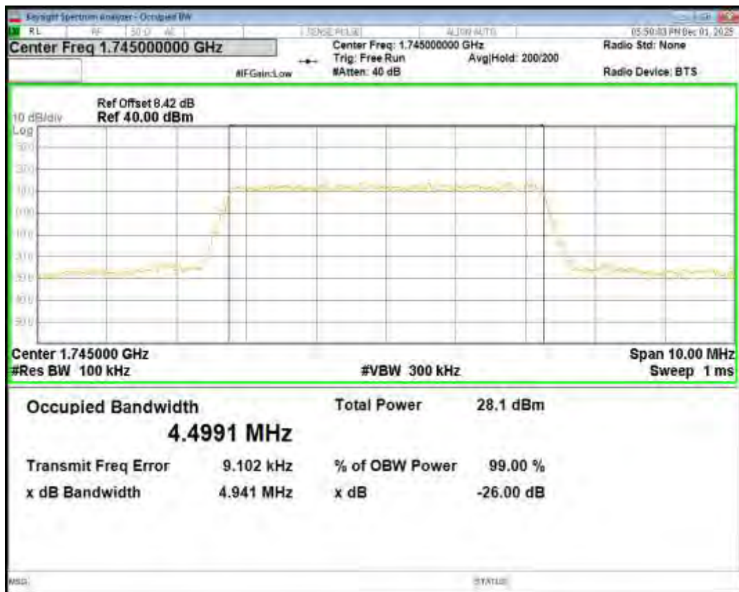
Band66 16QAM BW=5MHz Channel=132647 RB Size=25 Position=#0
