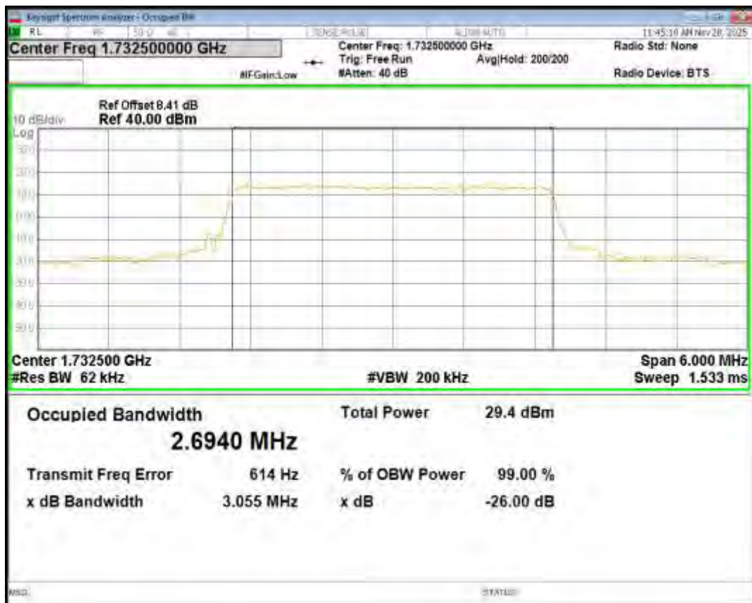
Band4 QPSK BW=3MHz Channel=20385 RB Size=15 Position=#0
