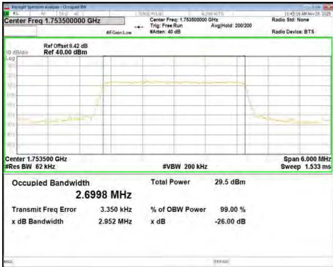
Band4 QPSK BW=5MHz Channel=19975 RB Size=25 Position=#0
