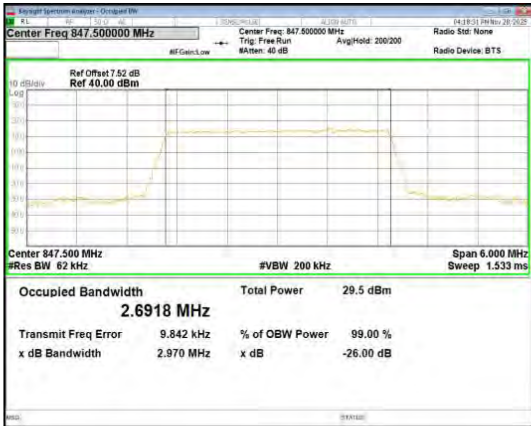
Band5 16QAM BW=5MHz Channel=20425 RB Size=25 Position=#0
