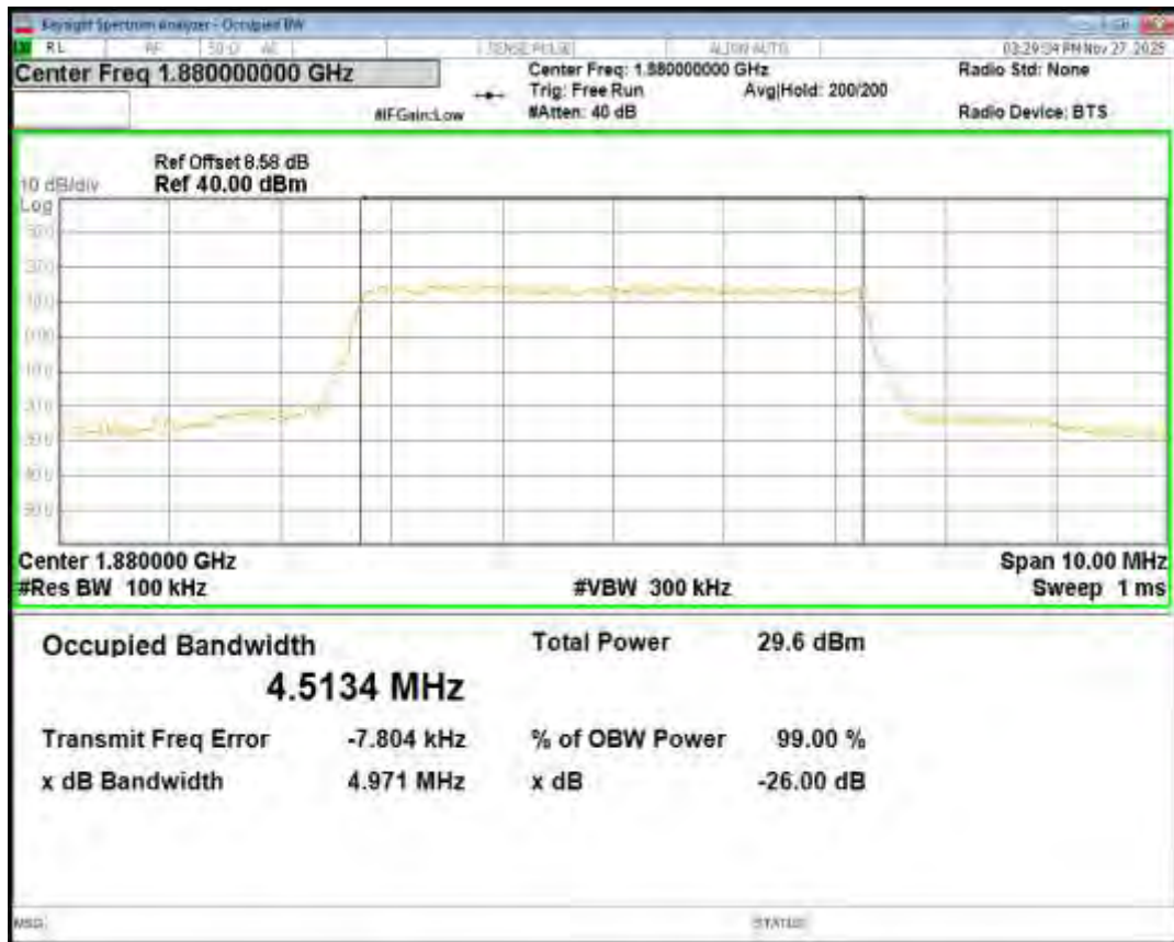
Band2 QPSK BW=5MHz Channel=19175 RB Size=25 Position=#0
