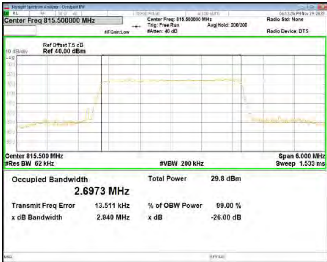
Band26(814-824) 16QAM BW=3MHz Channel=26775 RB Size=15 Position=#0
