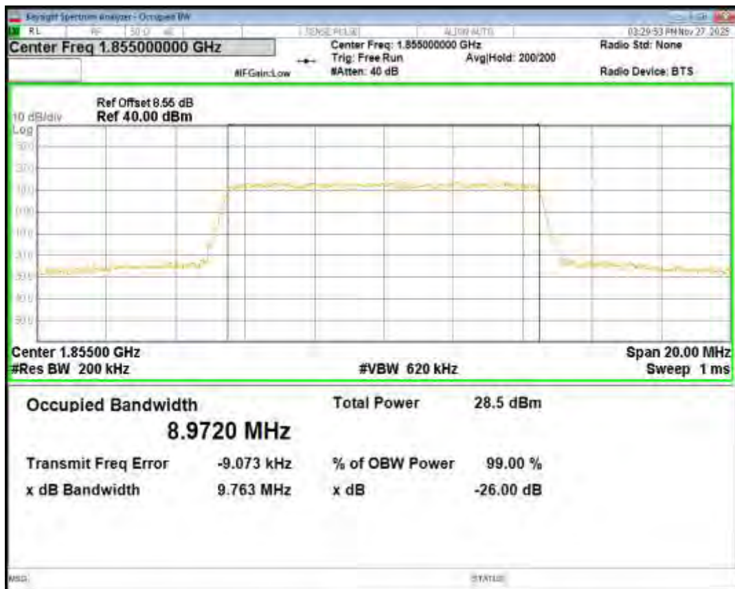
Band2 16QAM BW=10MHz Channel=18900 RB Size=50 Position=#0
