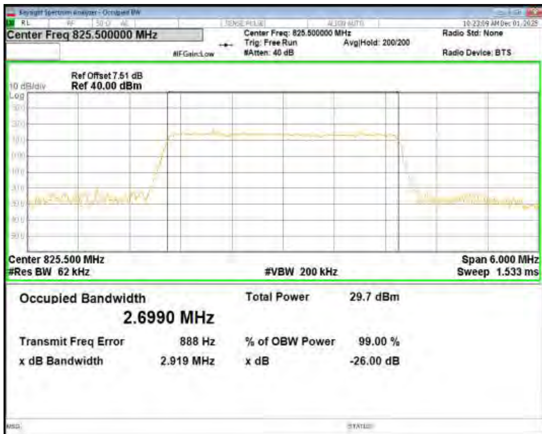
Band26(824-849) 16QAM BW=3MHz Channel=26915 RB Size=15 Position=#0
