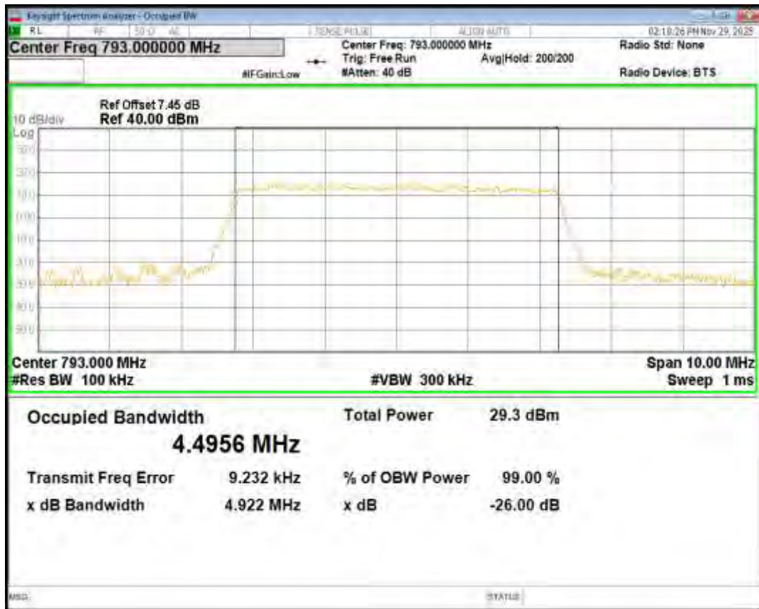
Band14 16QAM BW=5MHz Channel=23355 RB Size=25 Position=#0
