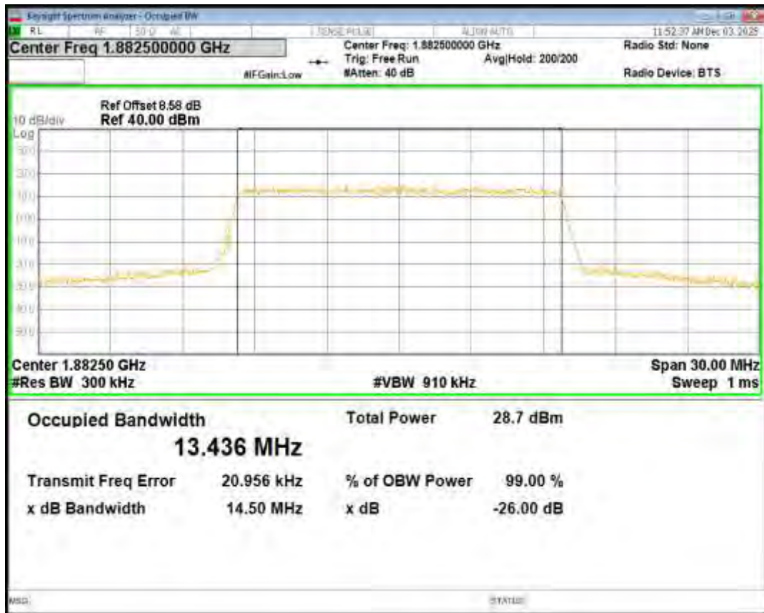
Band25 16QAM BW=20MHz Channel=26140 RB Size=100 Position=#0
