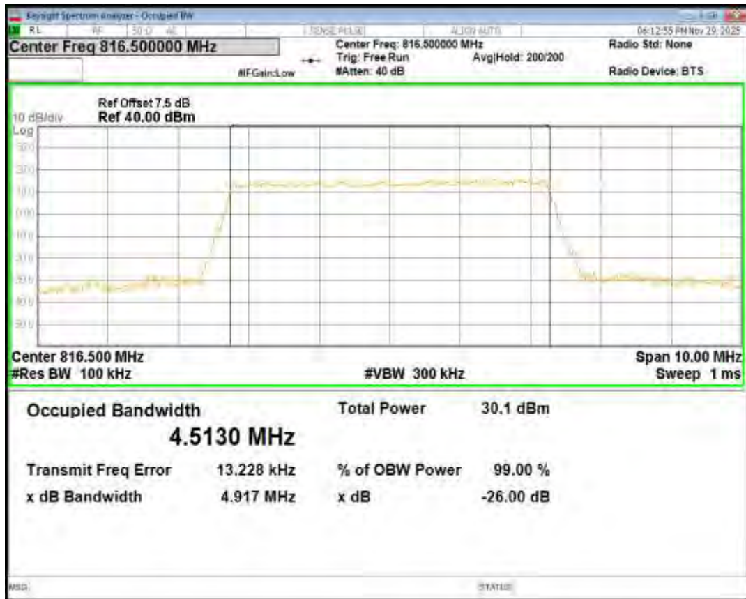
Band26(814-824) QPSK BW=5MHz Channel=26765 RB Size=25 Position=#0
