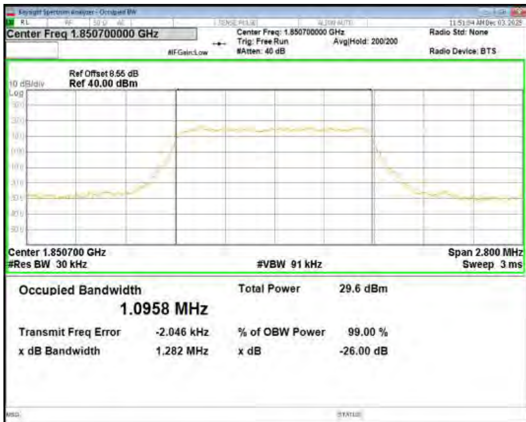
Band25 QPSK BW=10MHz Channel=26365 RB Size=50 Position=#0
