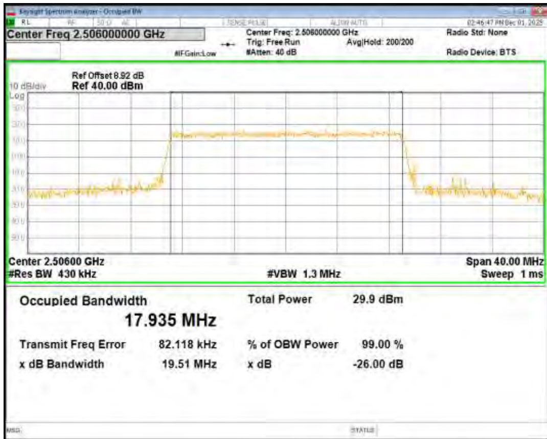
Band41 16QAM BW=20MHz Channel=40620 RB Size=100 Position=#0
