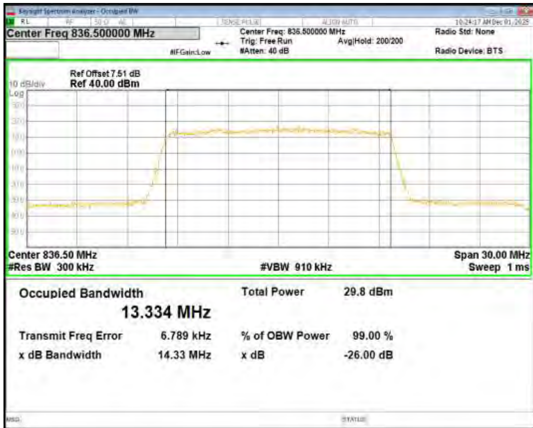
Band26(824-849) QPSK BW=15MHz Channel=26965 RB Size=75 Position=#0
