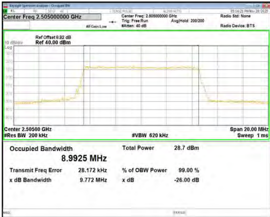
Band7 QPSK BW=10MHz Channel=21100 RB Size=50 Position=#0
