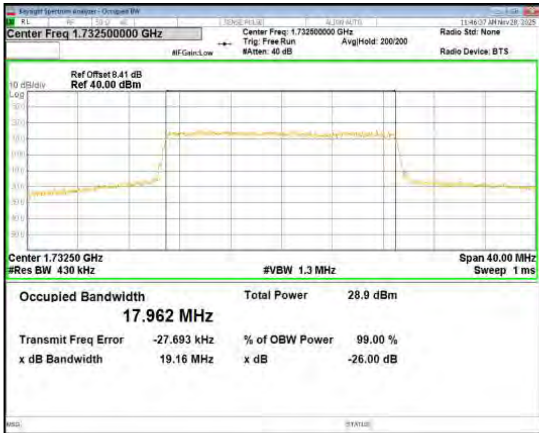
Band4 QPSK BW=20MHz Channel=20300 RB Size=100 Position=#0
