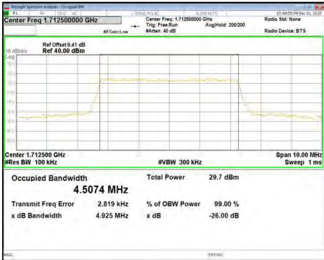
Band66 QPSK BW=5MHz Channel=132322 RB Size=25 Position=#0
