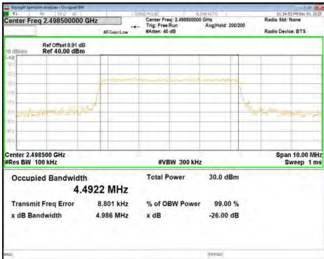
Band41 16QAM BW=5MHz Channel=40620 RB Size=25 Position=#0
