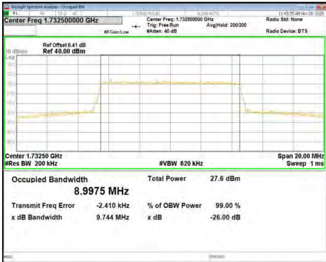
Band4 16QAM BW=10MHz Channel=20350 RB Size=50 Position=#0
