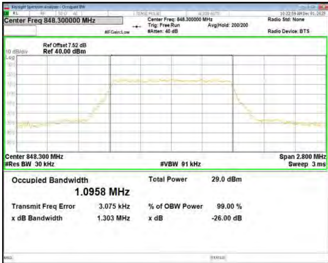
Band26(824-849) 16QAM BW=10MHz Channel=26840 RB Size=50 Position=#0
