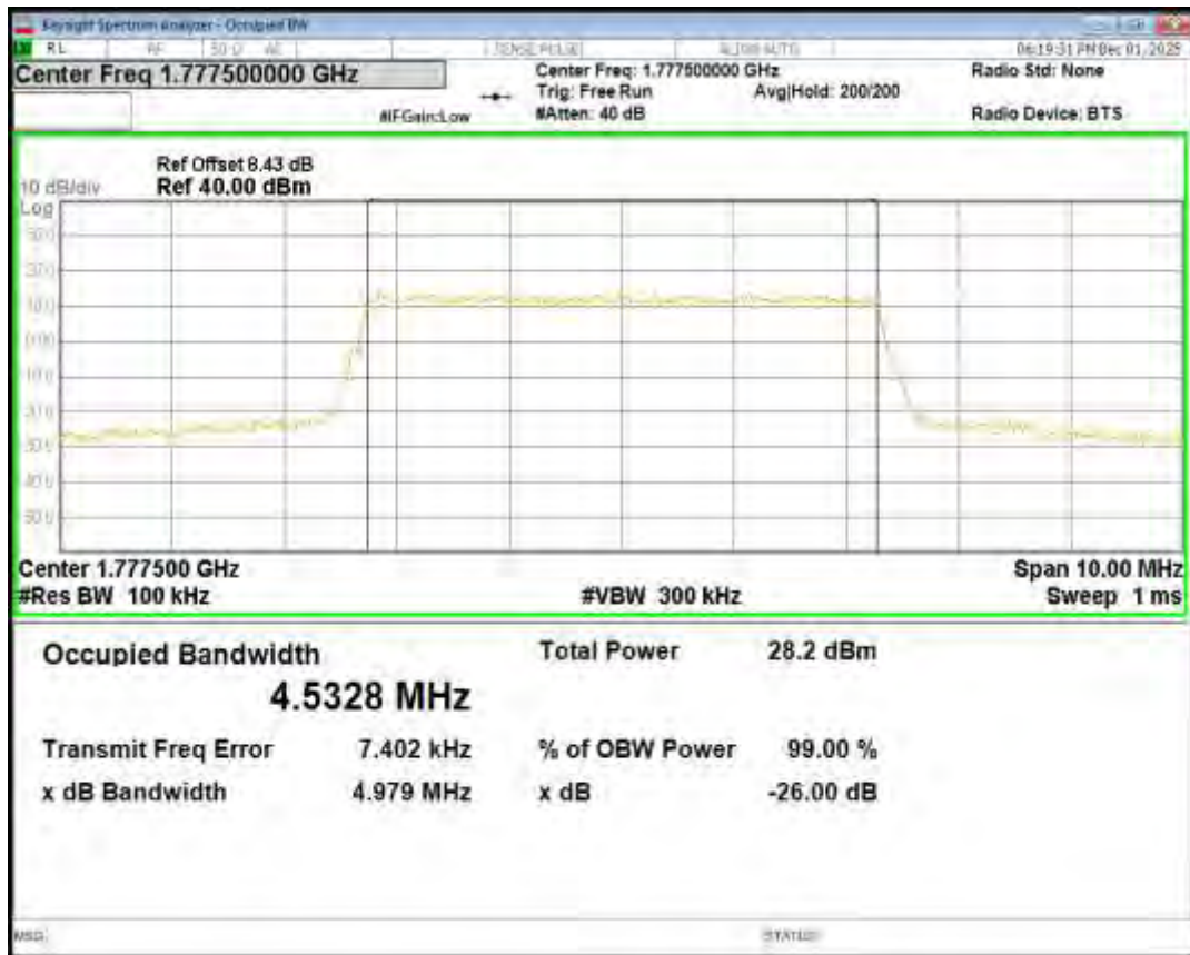
Band66 16QAM BW=5MHz Channel=131997 RB Size=25 Position=#0
