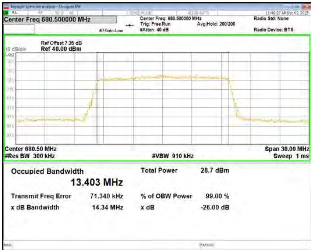
Band71 16QAM BW=15MHz Channel=133397 RB Size=75 Position=#0
