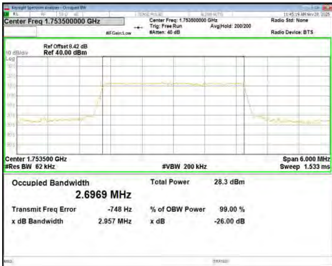
Band4 QPSK BW=1.4MHz Channel=19957 RB Size=6 Position=#0
