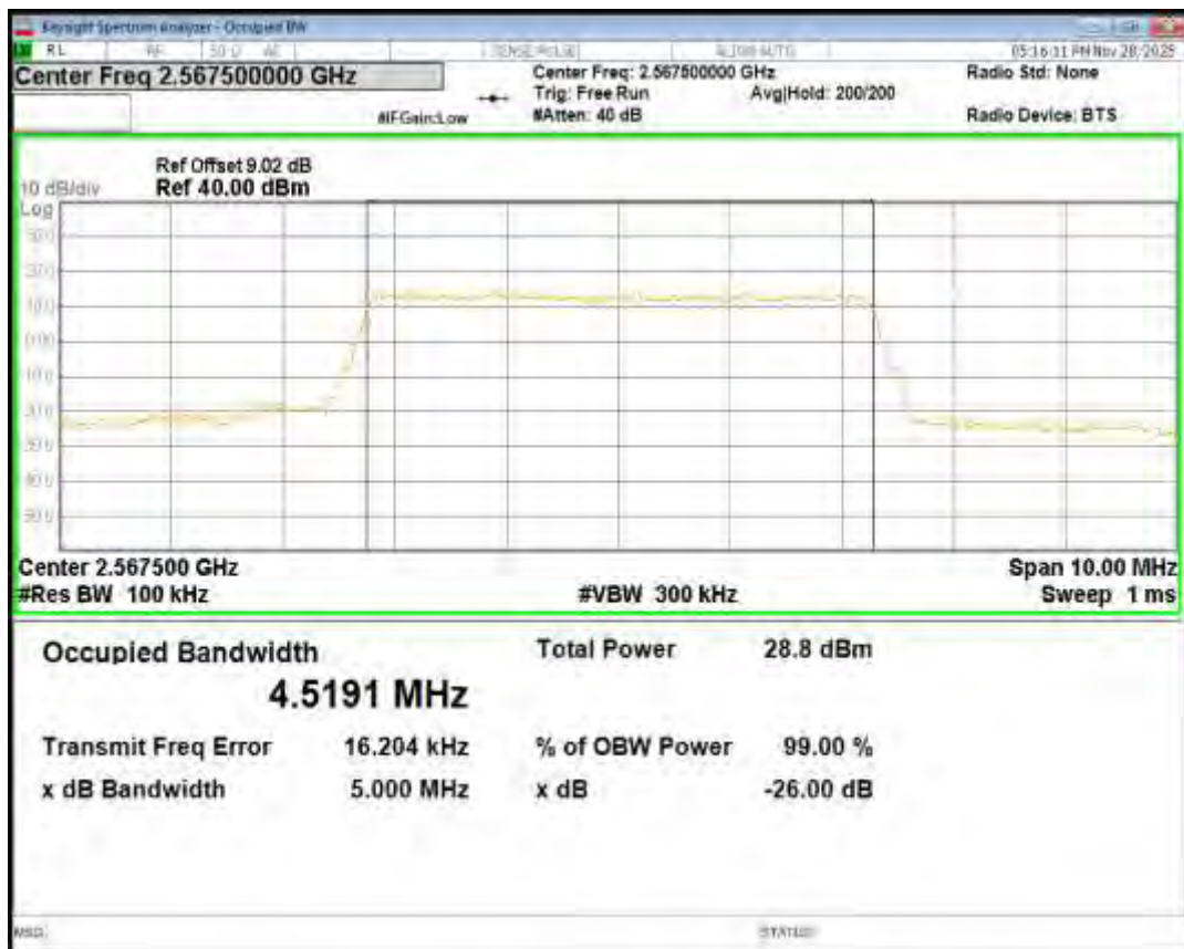
Band71 16QAM BW=10MHz Channel=133172 RB Size=50 Position=#0
