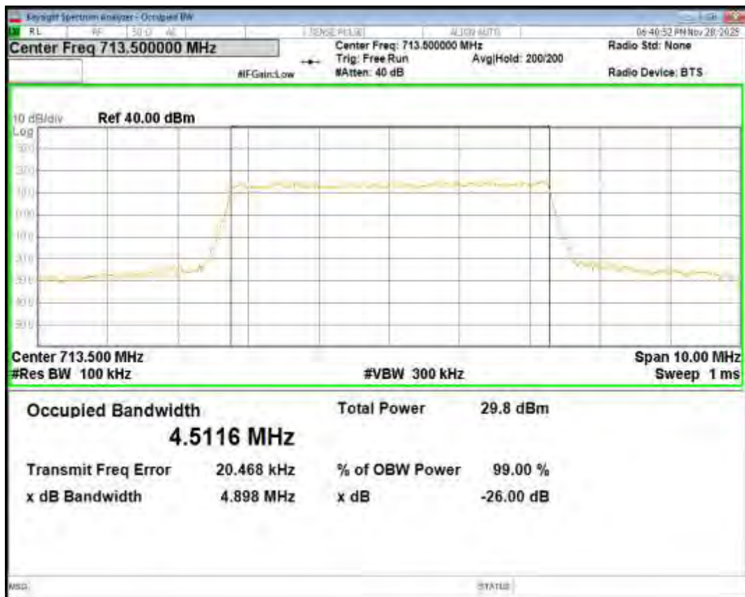
Band13 16QAM BW=10MHz Channel=23230 RB Size=50 Position=#0
