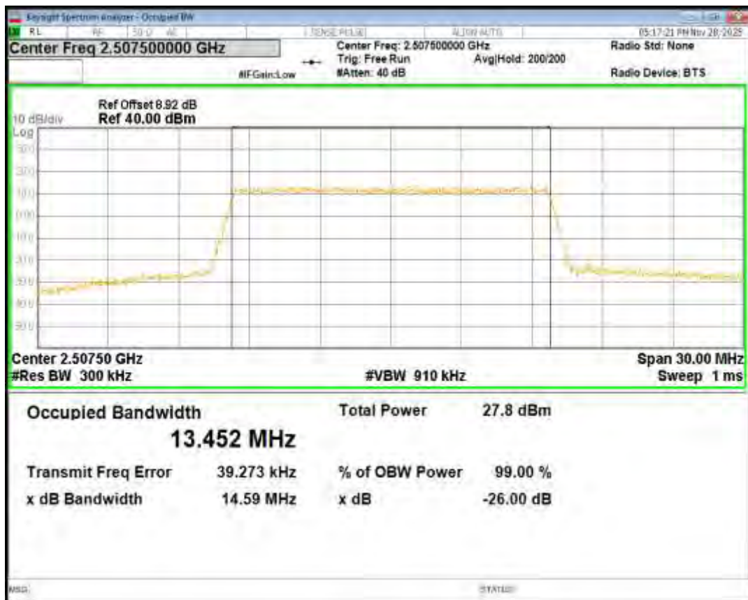
Band7 16QAM BW=15MHz Channel=21100 RB Size=75 Position=#0
