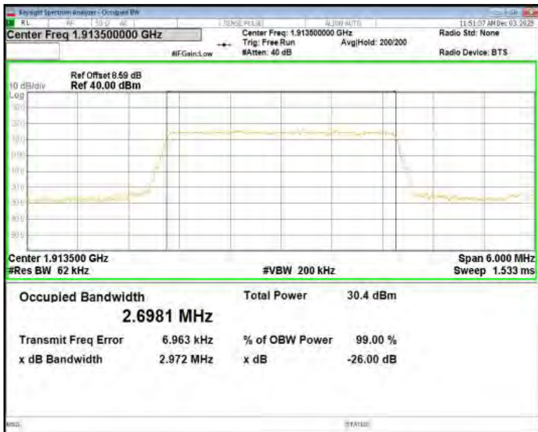
Band25 QPSK BW=5MHz Channel=26065 RB Size=25 Position=#0
