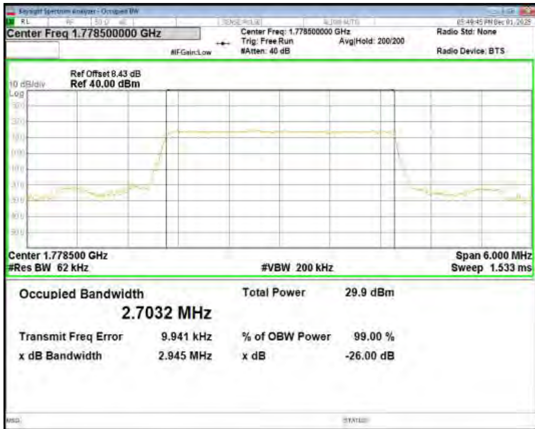
Band66 QPSK BW=5MHz Channel=132647 RB Size=25 Position=#0
