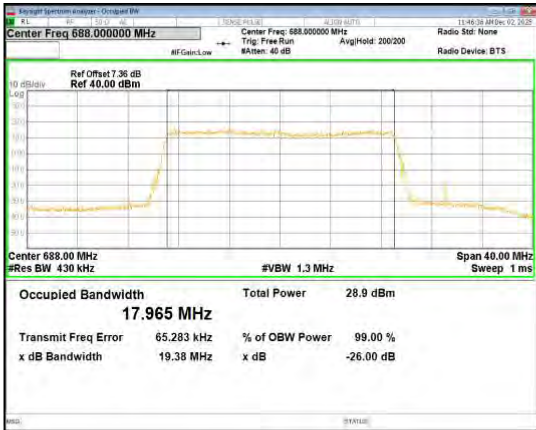
Band71 16QAM BW=5MHz Channel=133147 RB Size=25 Position=#0
