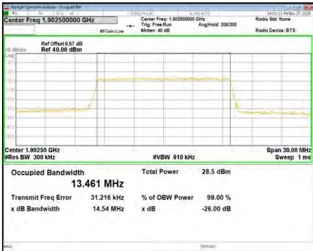
Band2 16QAM BW=15MHz Channel=18675 RB Size=75 Position=#0
