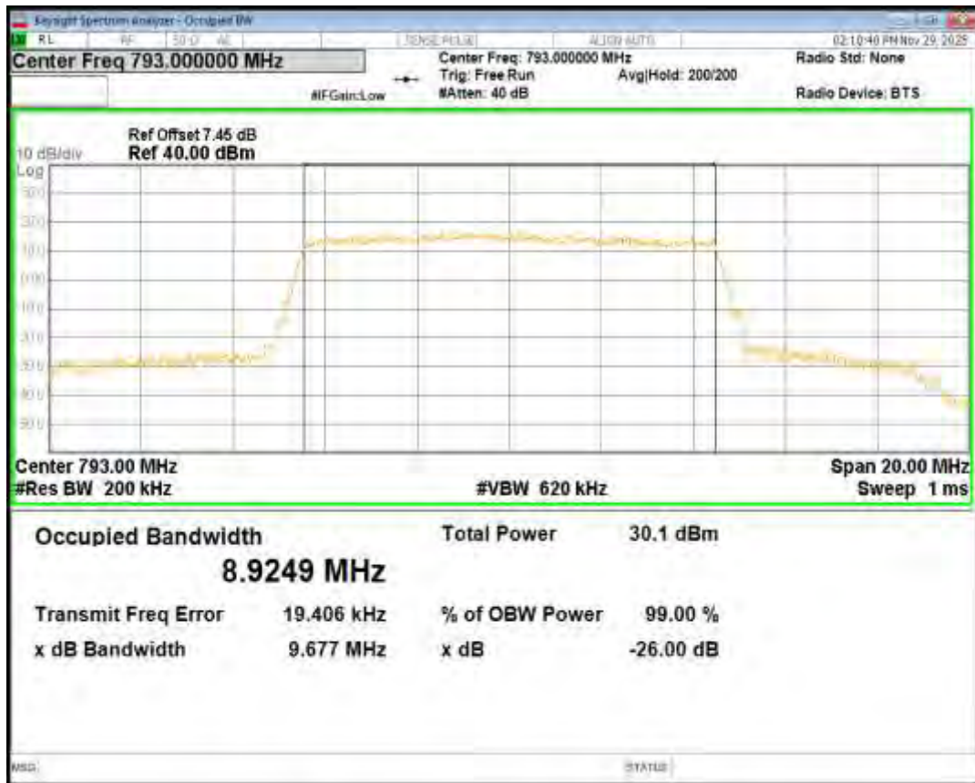
Band14 QPSK BW=5MHz Channel=23305 RB Size=25 Position=#0
