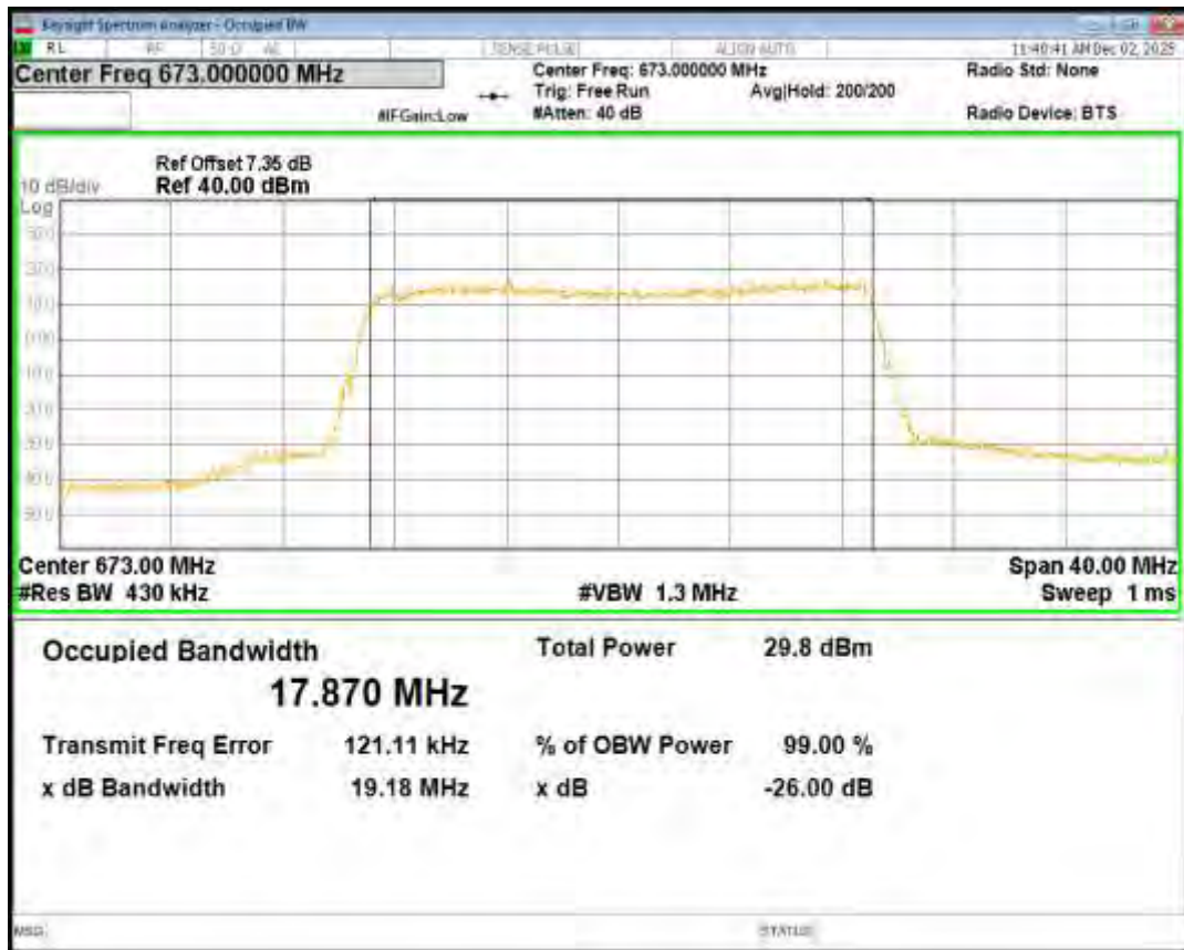
Band71 QPSK BW=20MHz Channel=133297 RB Size=100 Position=#0
