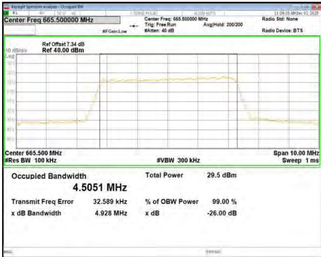
Band71 QPSK BW=5MHz Channel=133447 RB Size=25 Position=#0
