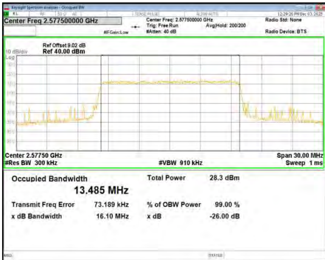
Band38 QPSK BW=15MHz Channel=38000 RB Size=75 Position=#0
