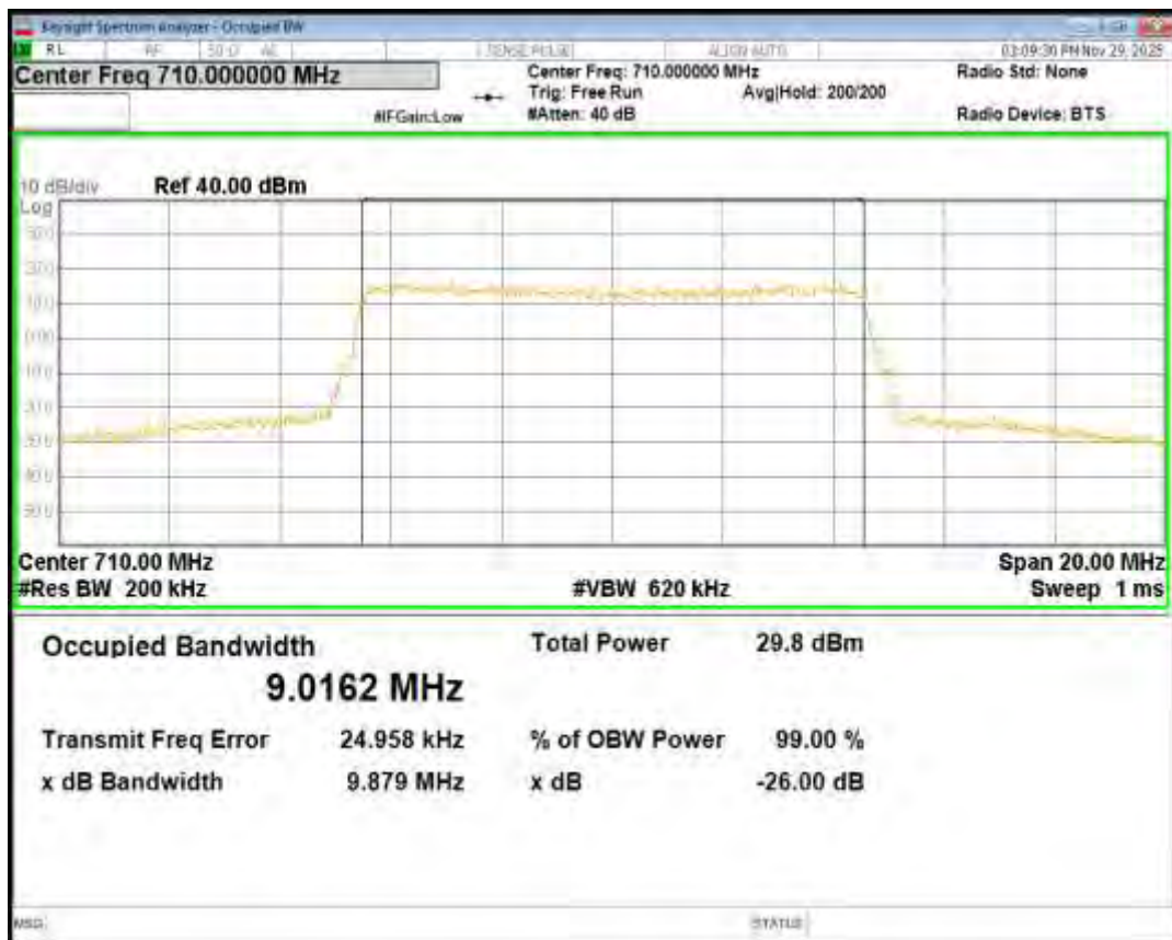
Band17 QPSK BW=10MHz Channel=23800 RB Size=50 Position=#0
