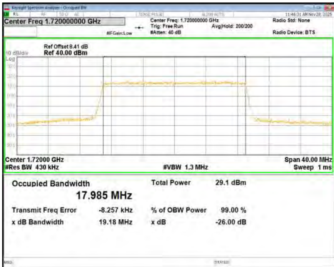
Band4 QPSK BW=15MHz Channel=20325 RB Size=75 Position=#0
