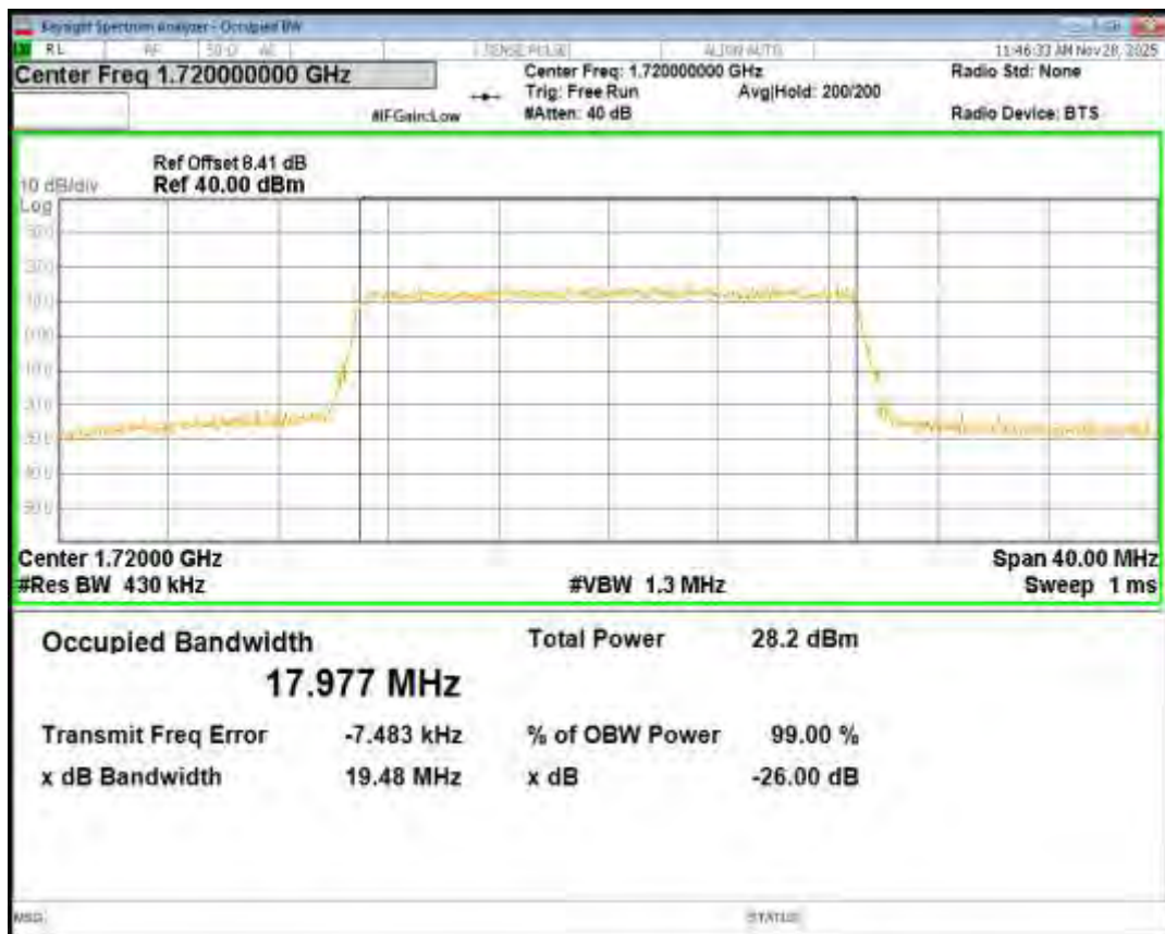
Band4 16QAM BW=20MHz Channel=20175 RB Size=100 Position=#0
