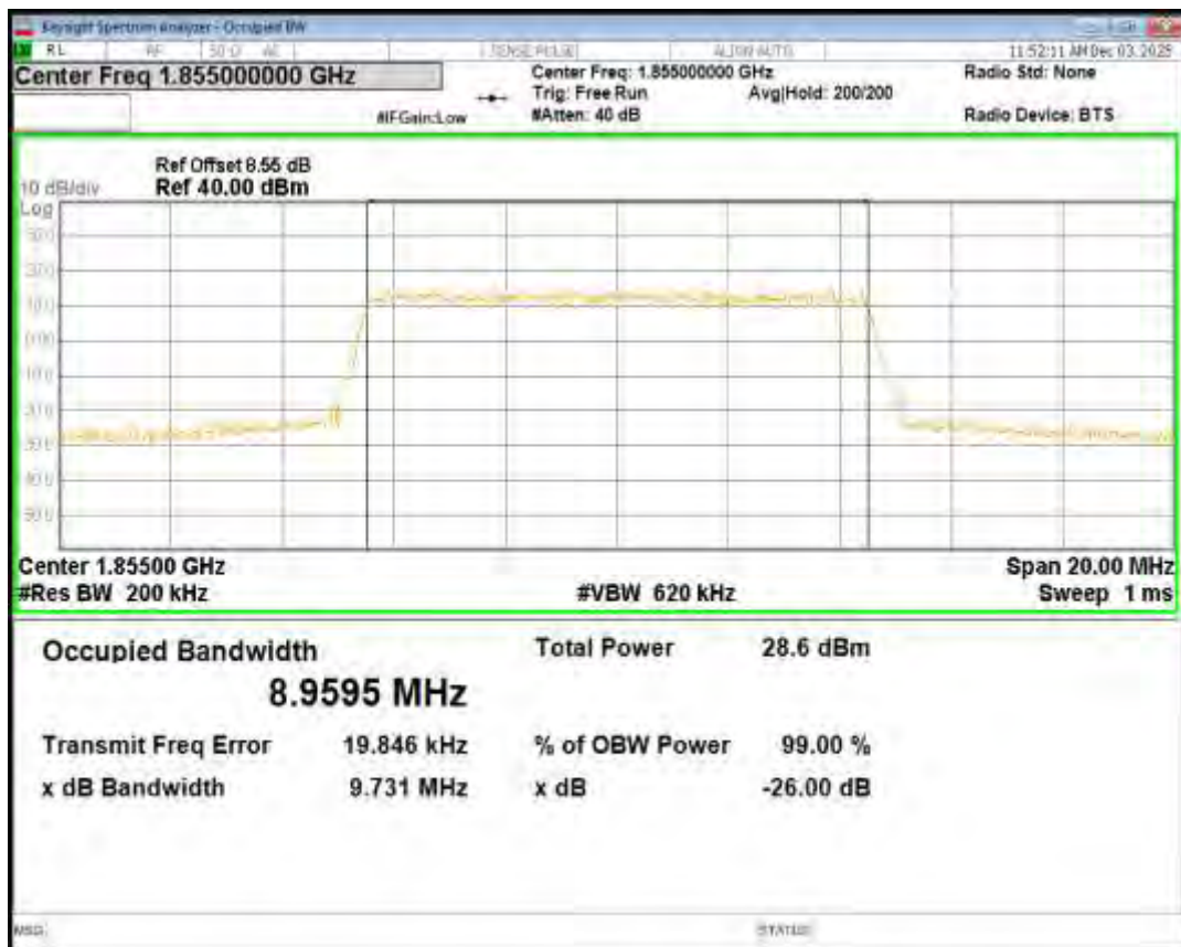
Band25 16QAM BW=10MHz Channel=26365 RB Size=50 Position=#0
