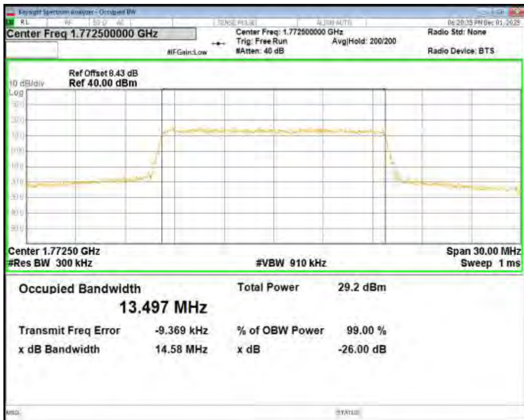
Band66 QPSK BW=10MHz Channel=132622 RB Size=50 Position=#0
