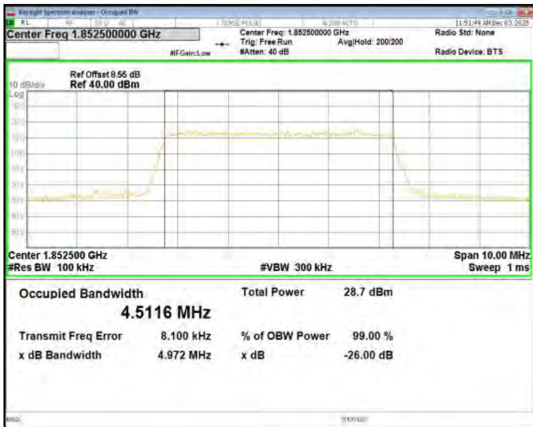
Band25 QPSK BW=1.4MHz Channel=26683 RB Size=6 Position=#0
