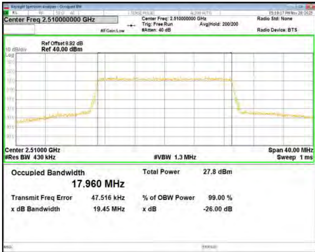
Band7 16QAM BW=20MHz Channel=21100 RB Size=100 Position=#0
