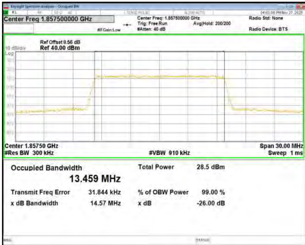
Band2 16QAM BW=10MHz Channel=19150 RB Size=50 Position=#0
