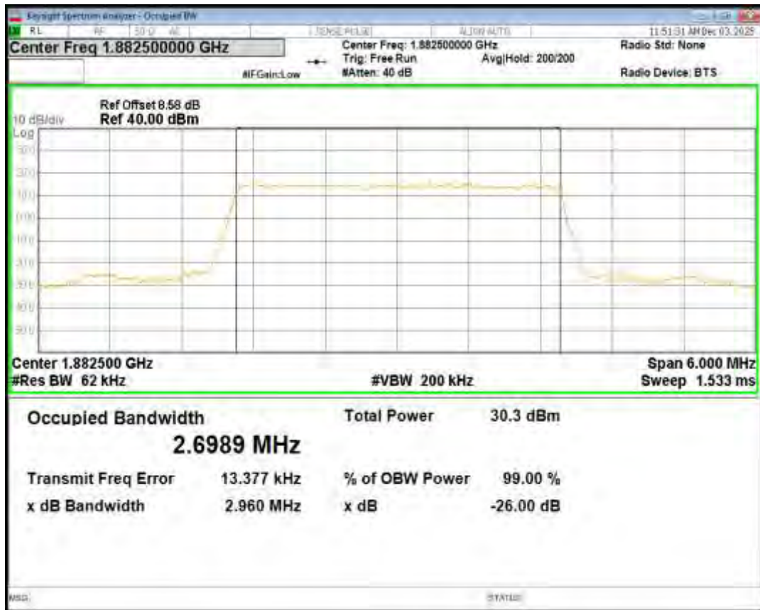
Band25 QPSK BW=3MHz Channel=26675 RB Size=15 Position=#0
