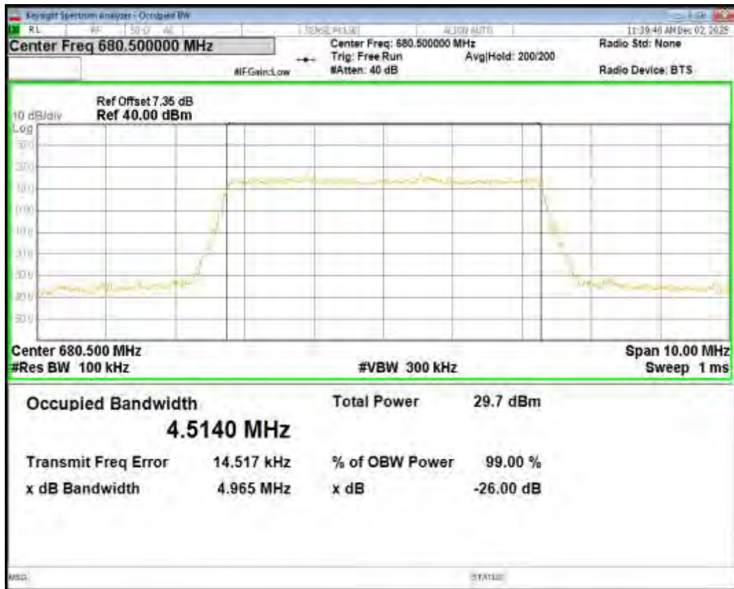
Band71 QPSK BW=20MHz Channel=133372 RB Size=100 Position=#0
