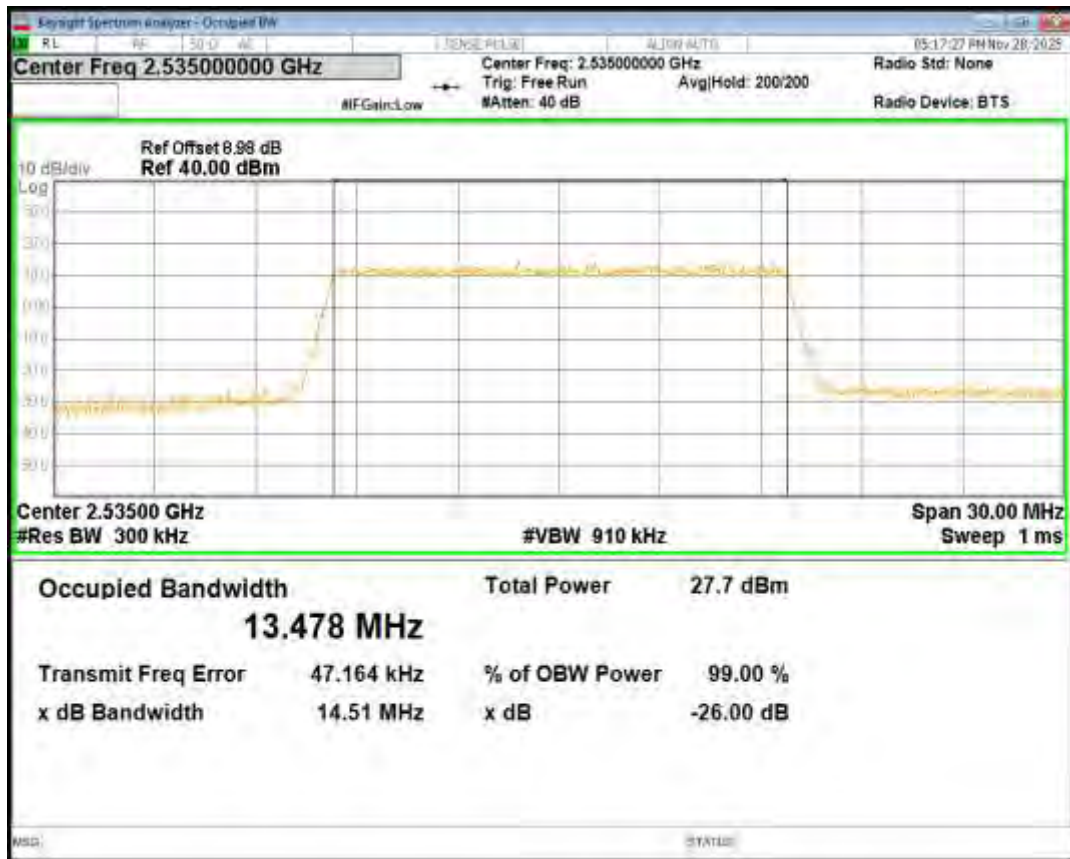
Band7 16QAM BW=15MHz Channel=21375 RB Size=75 Position=#0
