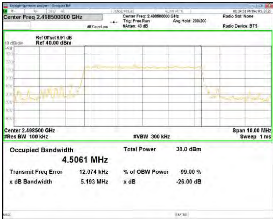
Band41 QPSK BW=5MHz Channel=41565 RB Size=25 Position=#0
