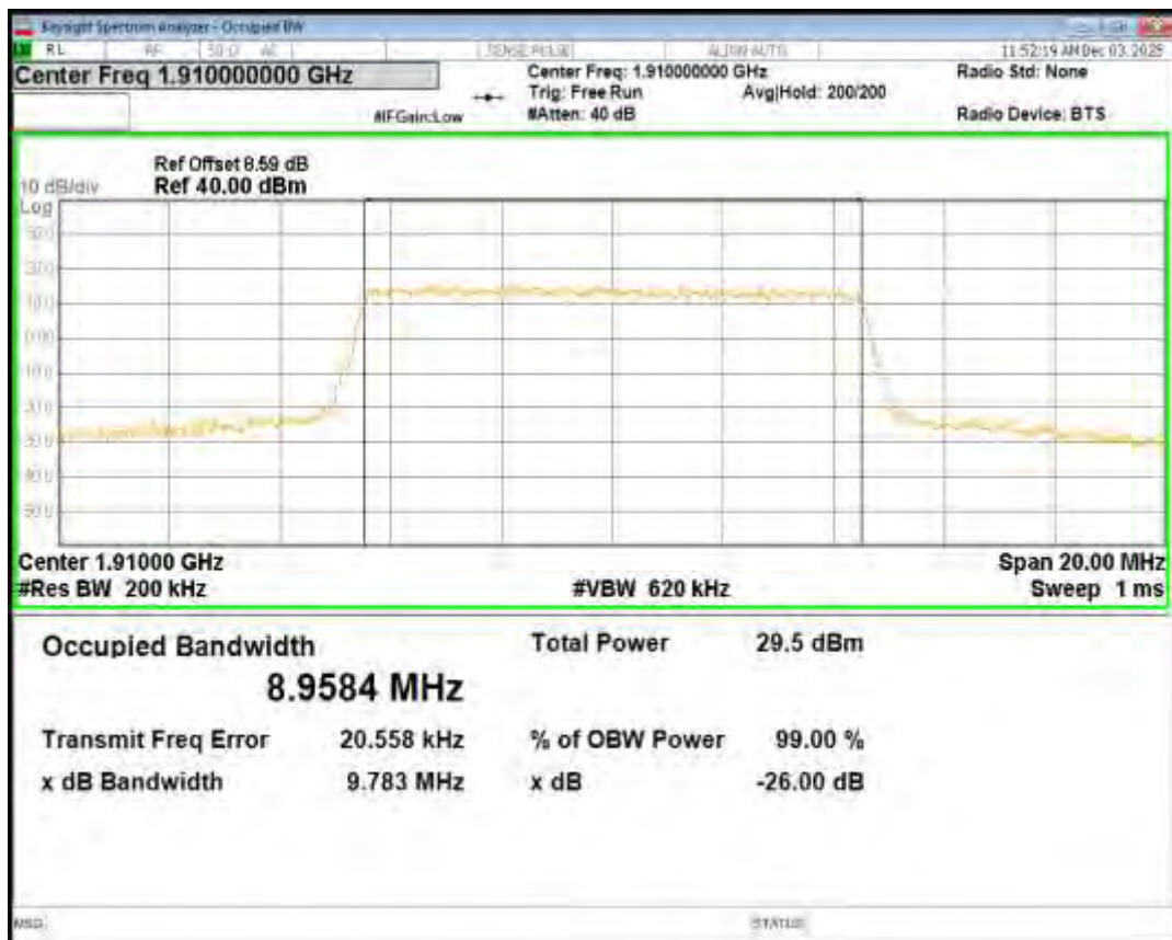
Band25 QPSK BW=15MHz Channel=26115 RB Size=75 Position=#0
