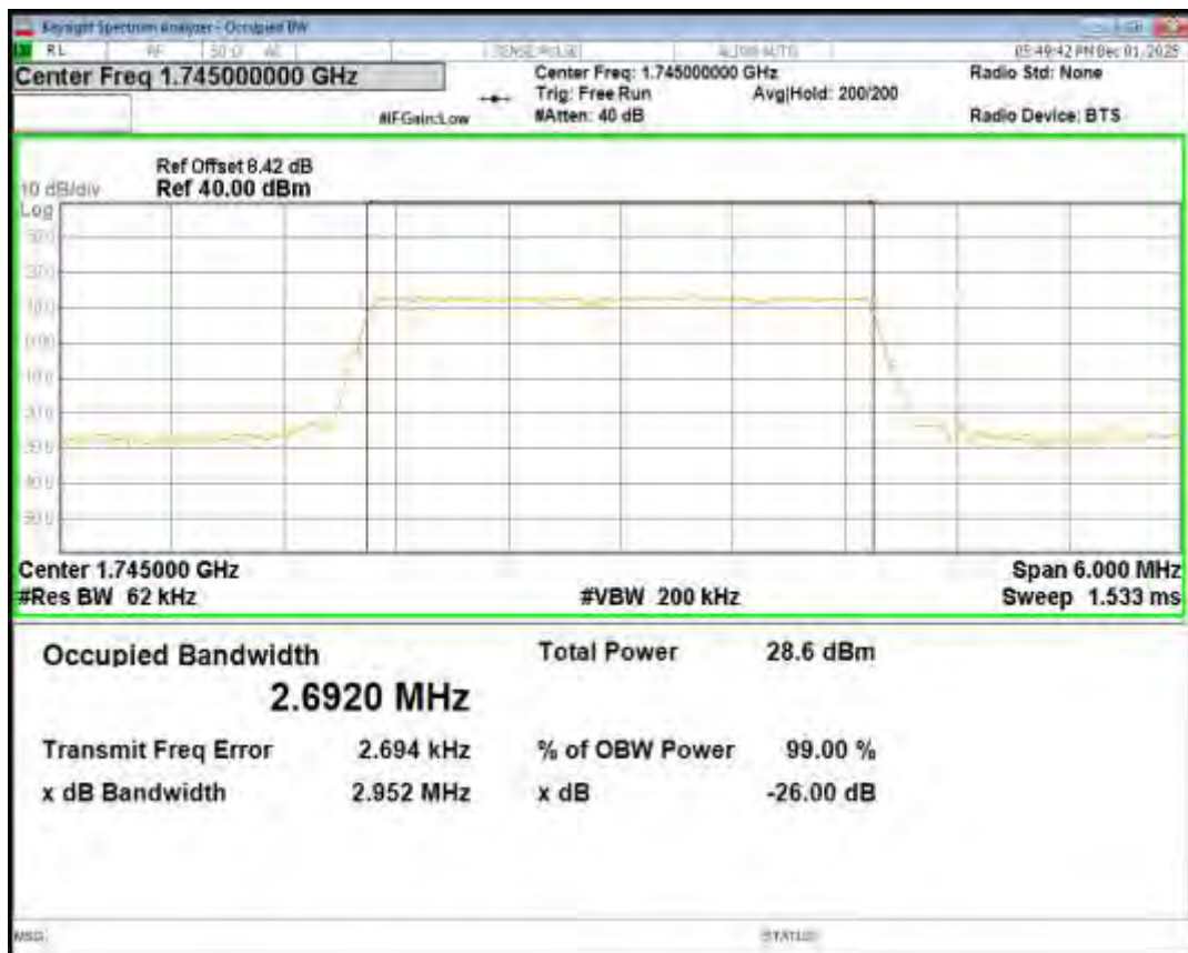
Band66 16QAM BW=3MHz Channel=132657 RB Size=15 Position=#0
