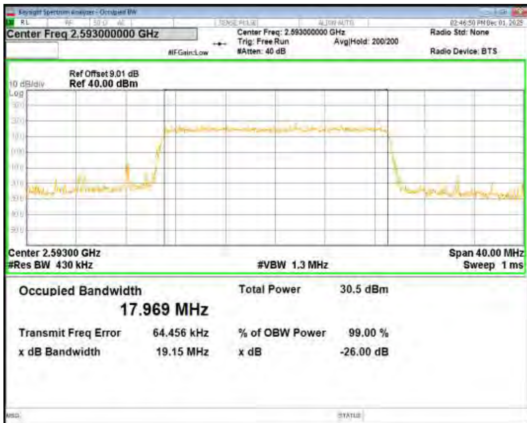
Band41 QPSK BW=20MHz Channel=41490 RB Size=100 Position=#0
