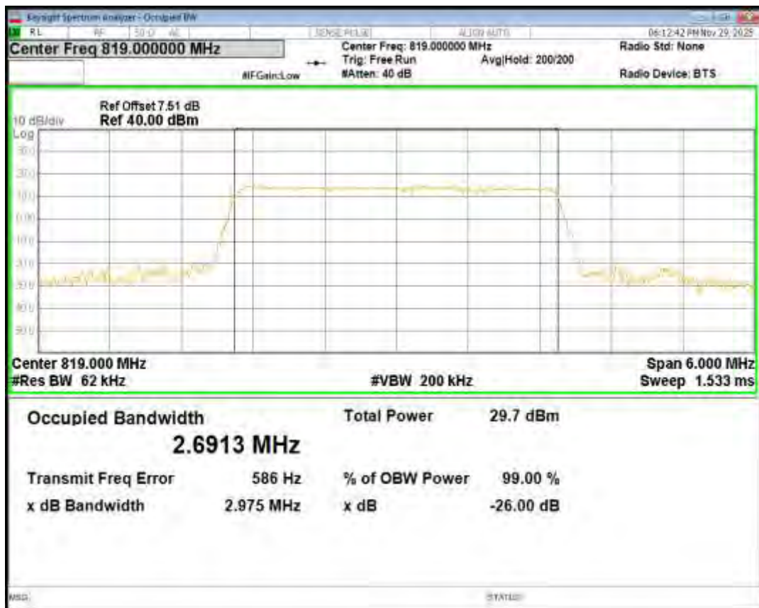
Band26(814-824) 16QAM BW=3MHz Channel=26705 RB Size=15 Position=#0
