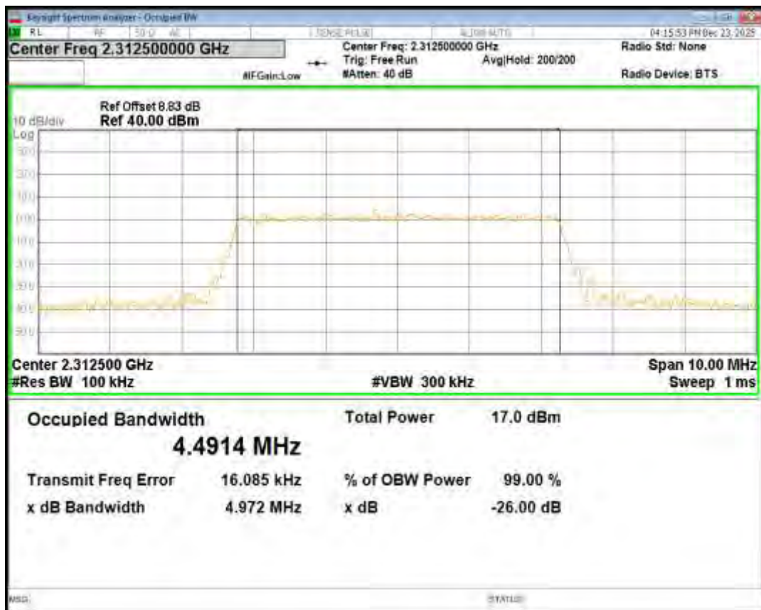
Band40(2350-2360) 16QAM BW=10MHz Channel=39200 RB Size=50 Position=#0
