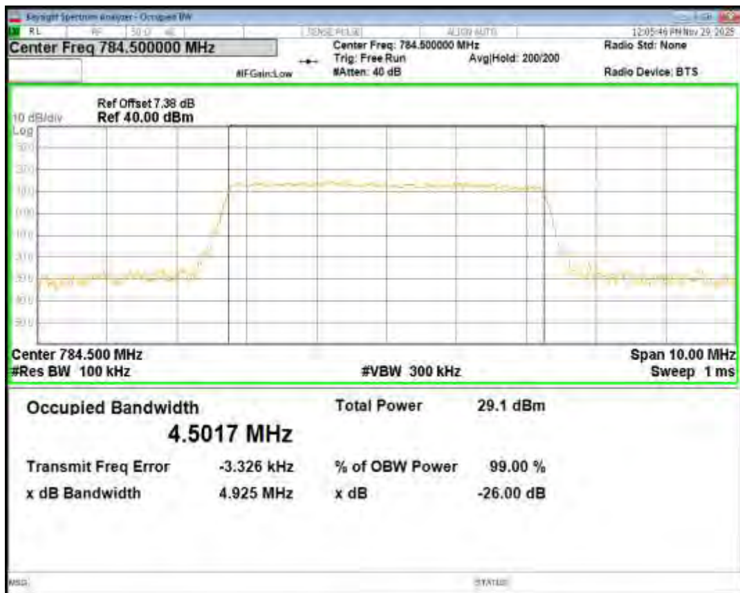
Band13 QPSK BW=10MHz Channel=23230 RB Size=50 Position=#0
