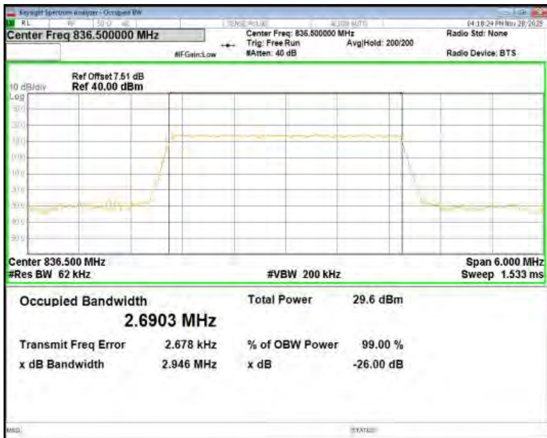
Band5 16QAM BW=5MHz Channel=20525 RB Size=25 Position=#0
