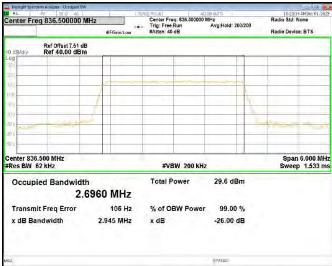
Band26(824-849) 16QAM BW=3MHz Channel=27025 RB Size=15 Position=#0
