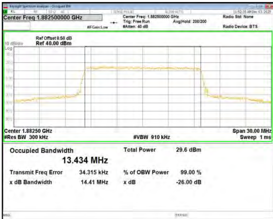
Band25 QPSK BW=15MHz Channel=26615 RB Size=75 Position=#0
