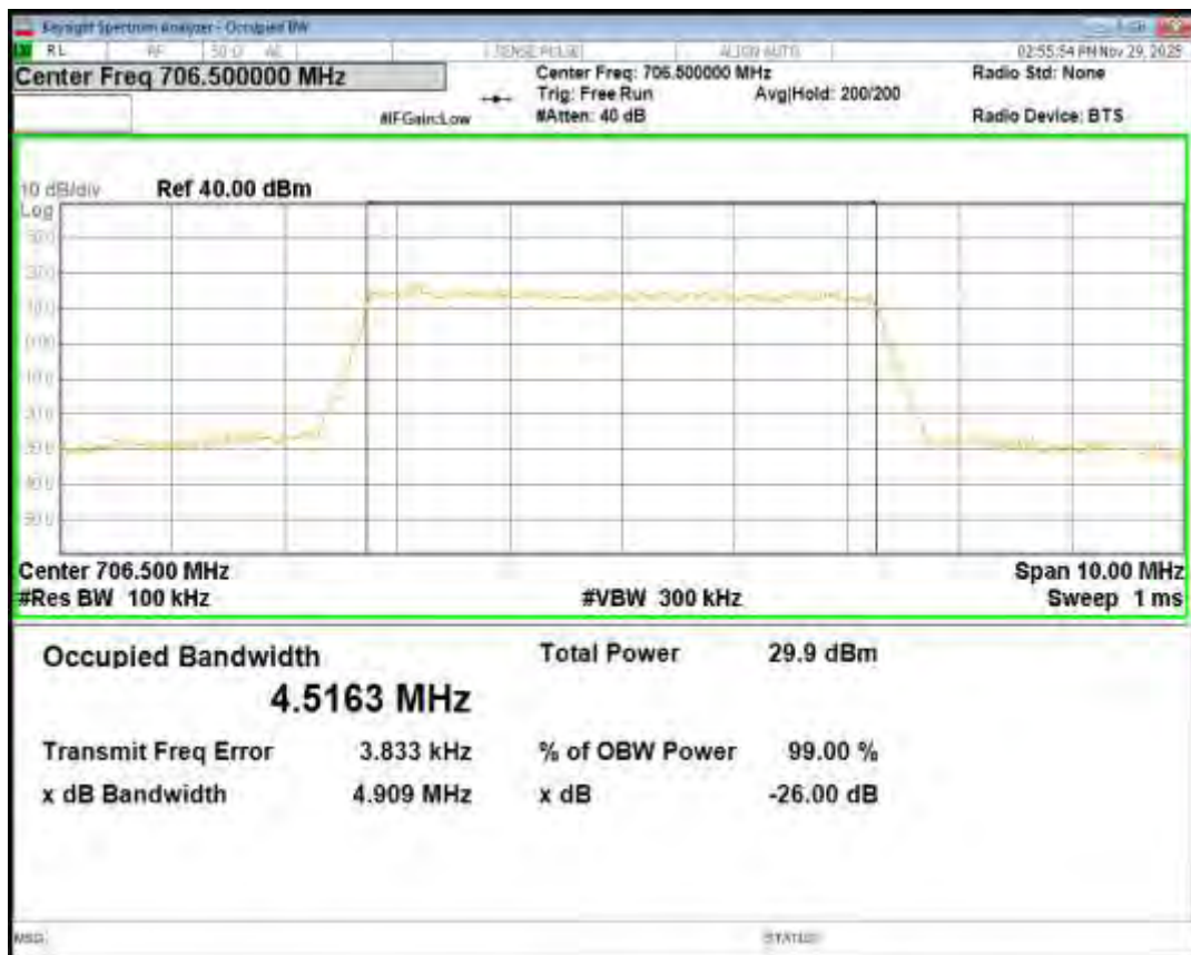
Band17 QPSK BW=5MHz Channel=23790 RB Size=25 Position=#0
