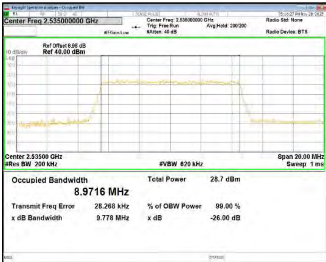
Band7 QPSK BW=10MHz Channel=21400 RB Size=50 Position=#0
