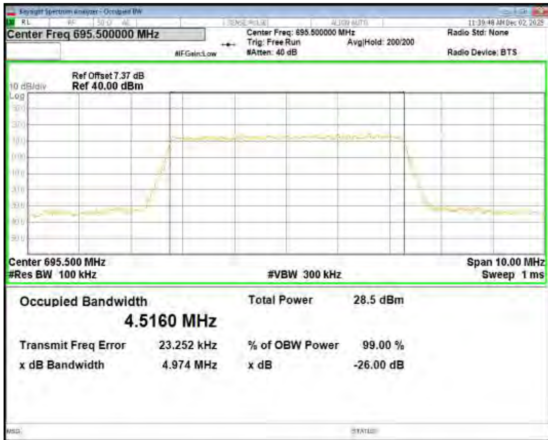
Band71 16QAM BW=5MHz Channel=133297 RB Size=25 Position=#0
