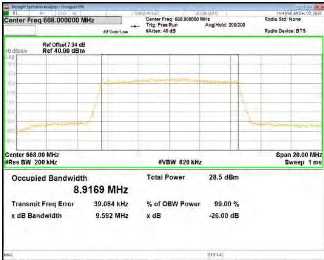
Band71 16QAM BW=10MHz Channel=133297 RB Size=50 Position=#0
