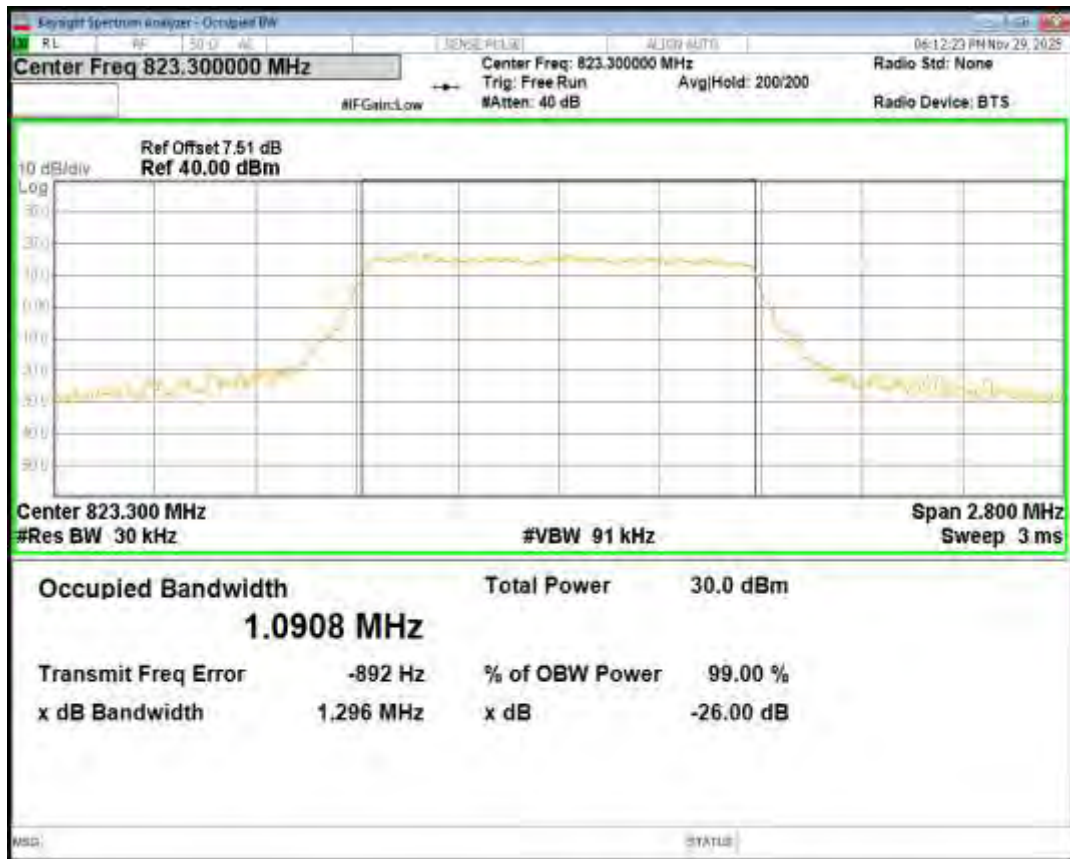
Band26(814-824) QPSK BW=10MHz Channel=26740 RB Size=50 Position=#0
