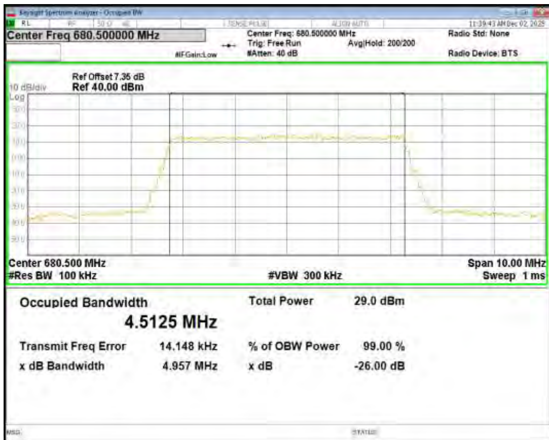
Band71 QPSK BW=10MHz Channel=133172 RB Size=50 Position=#0
