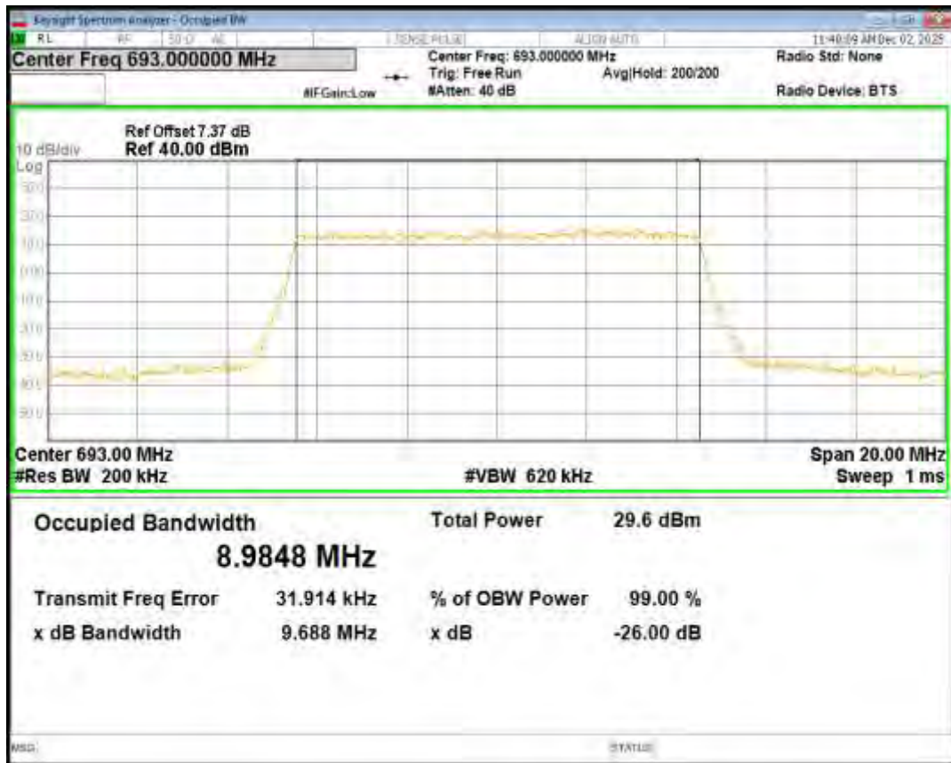
Band71 QPSK BW=10MHz Channel=133297 RB Size=50 Position=#0
