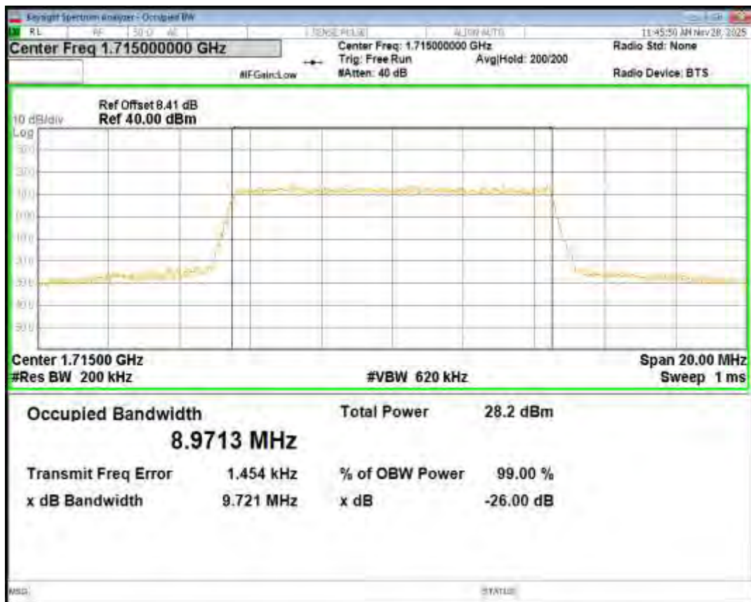
Band4 16QAM BW=10MHz Channel=20175 RB Size=50 Position=#0
