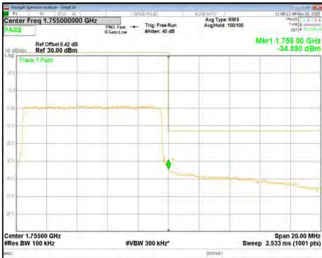
Band4 16QAM BW=15MHz Channel=20025 RB Size=75 Position=#0
