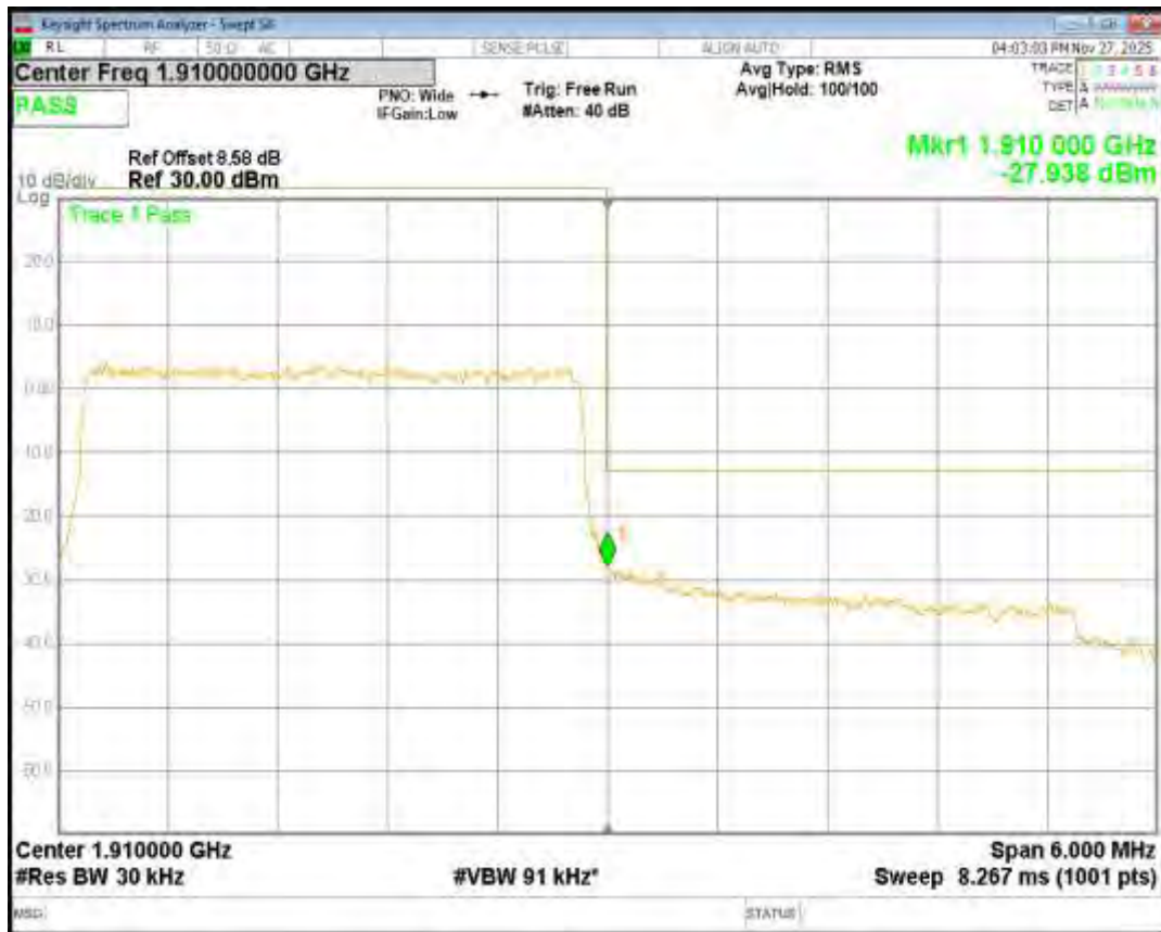
Band2 QPSK BW=5MHz Channel=19175 RB Size=25 Position=#0
