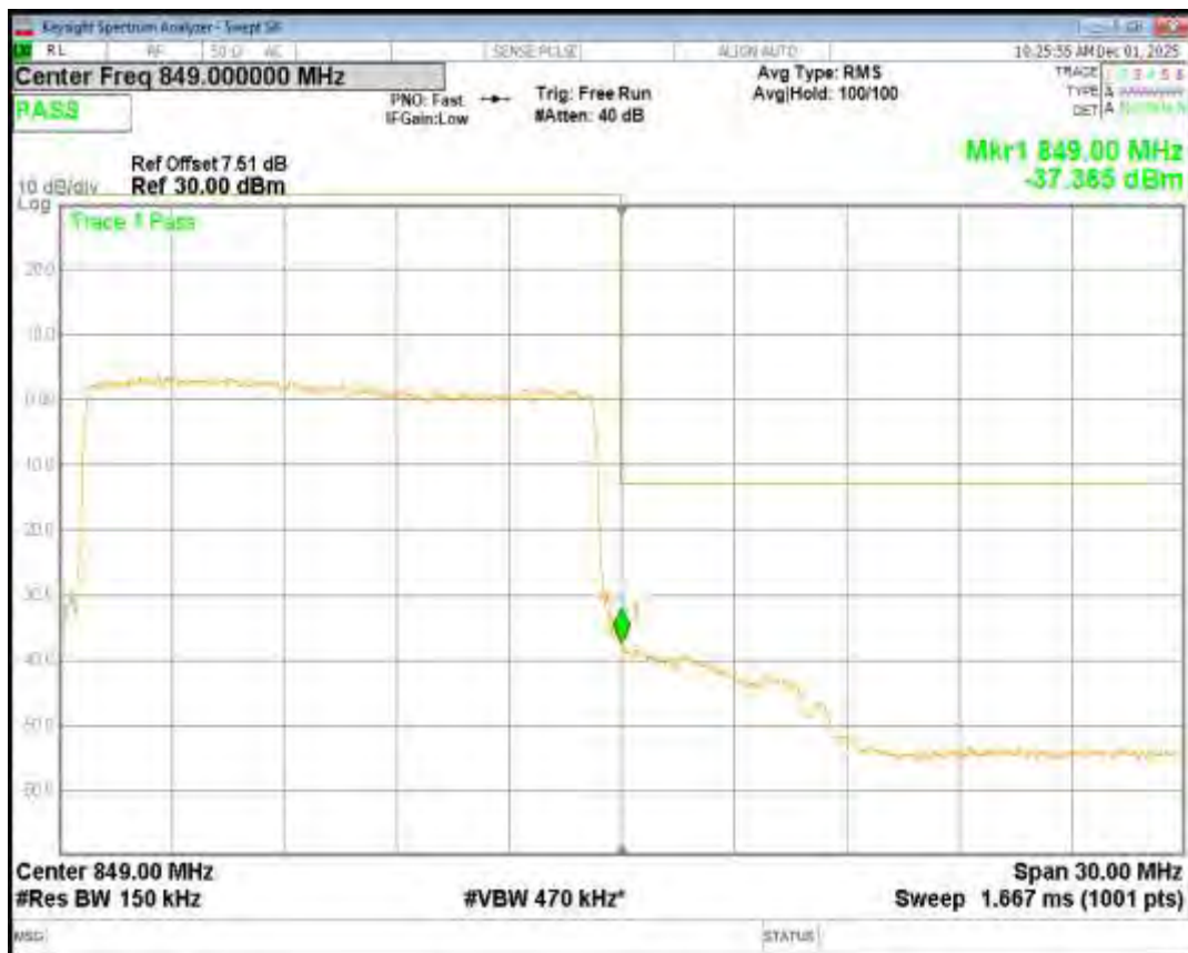
Band26(824-849) QPSK BW=1.4MHz Channel=26797 RB Size=6 Position=#0
