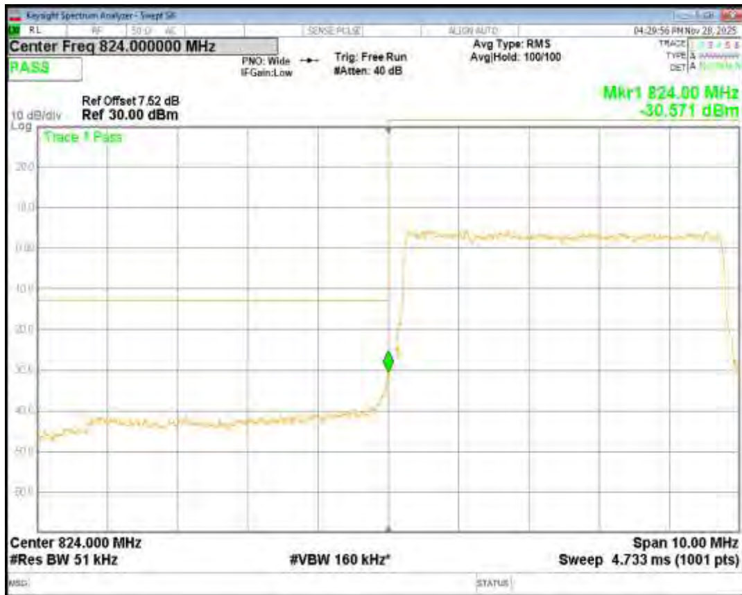
Band5 QPSK BW=5MHz Channel=20625 RB Size=25 Position=#0
