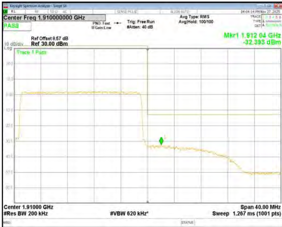
Band2 16QAM BW=3MHz Channel=18615 RB Size=15 Position=#0
