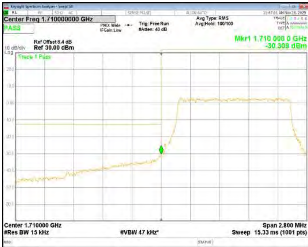
Band4 16QAM BW=1.4MHz Channel=20393 RB Size=6 Position=#0
