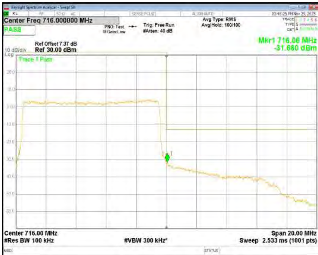
Band17 QPSK BW=5MHz Channel=23755 RB Size=25 Position=#0
