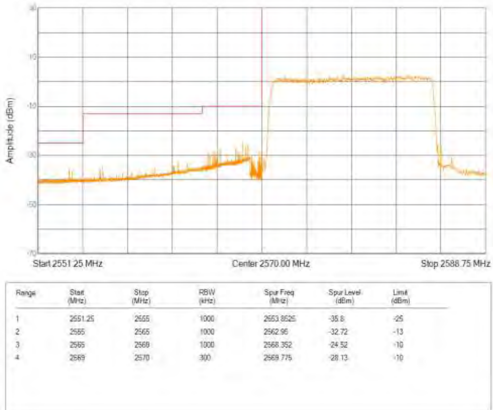
Band38 16QAM BW=15MHz Channel=38175 RB Size=75 Position=#0
