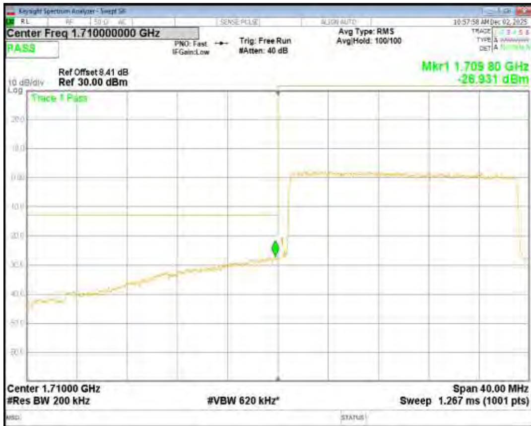
Band66 16QAM BW=20MHz Channel=132572 RB Size=100 Position=#0
