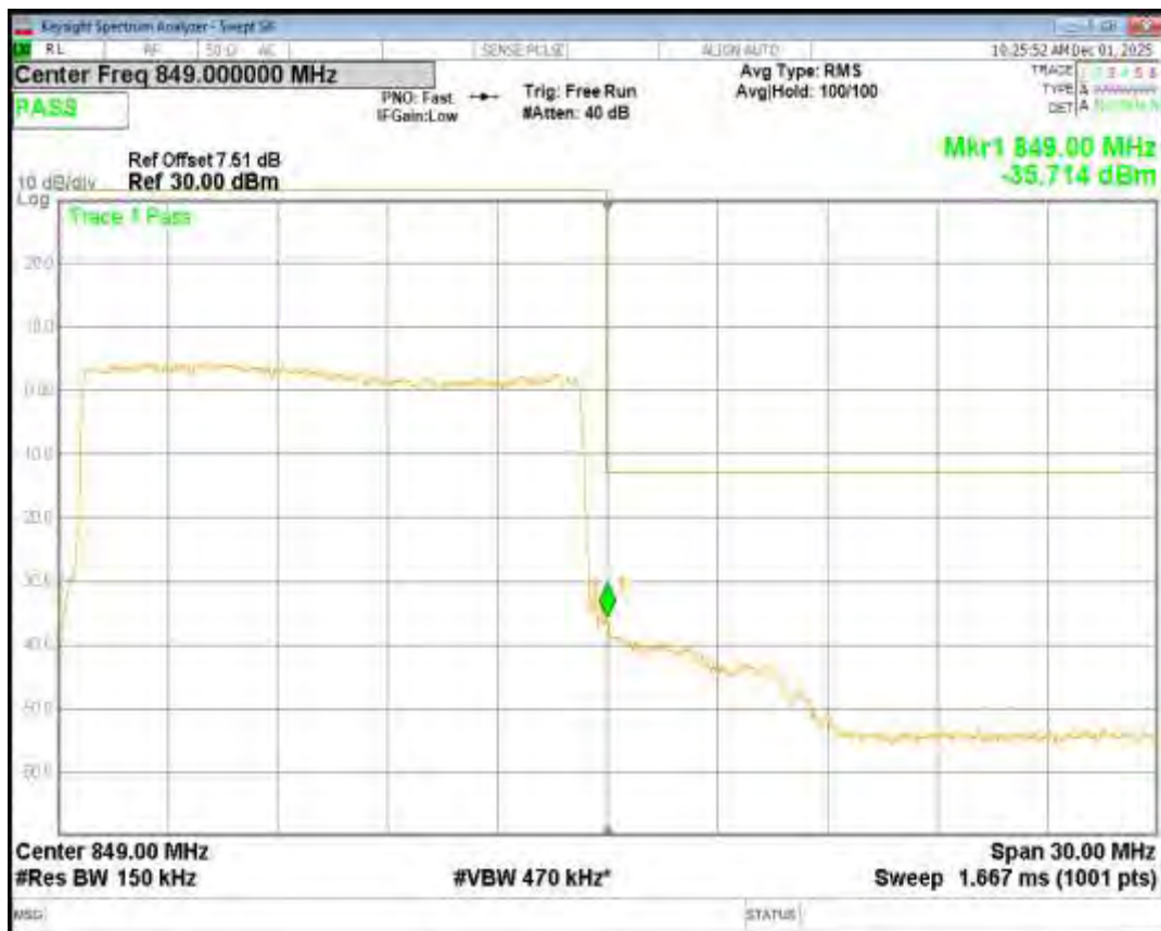
Band26(824-849) QPSK BW=3MHz Channel=26805 RB Size=15 Position=#0
