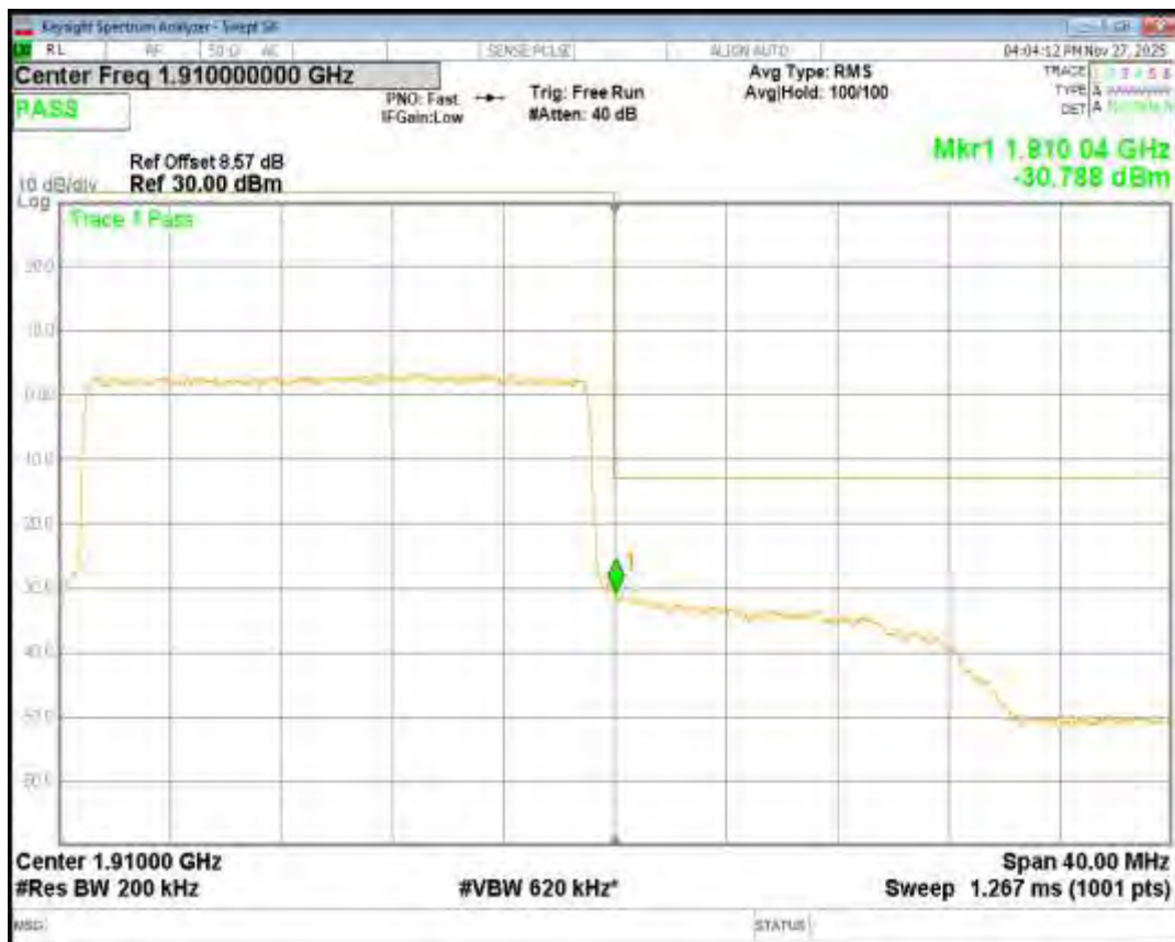
Band2 QPSK BW=5MHz Channel=18625 RB Size=25 Position=#0
