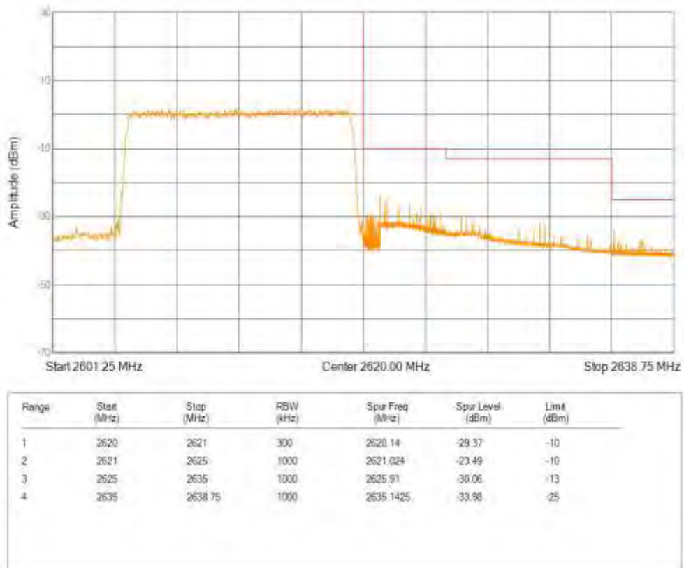
Band38 16QAM BW=20MHz Channel=37850 RB Size=100 Position=#0
