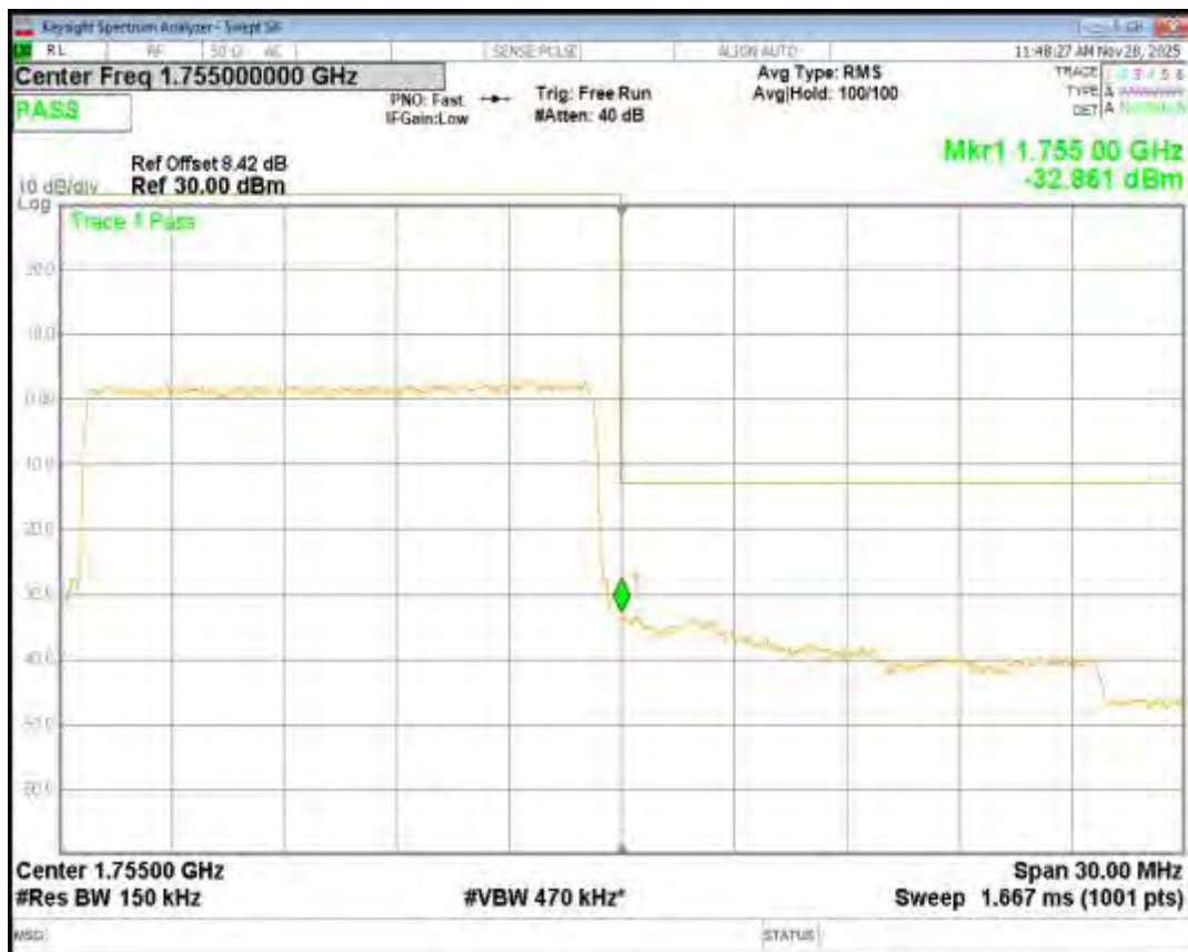
Band4 QPSK BW=20MHz Channel=20050 RB Size=100 Position=#0
