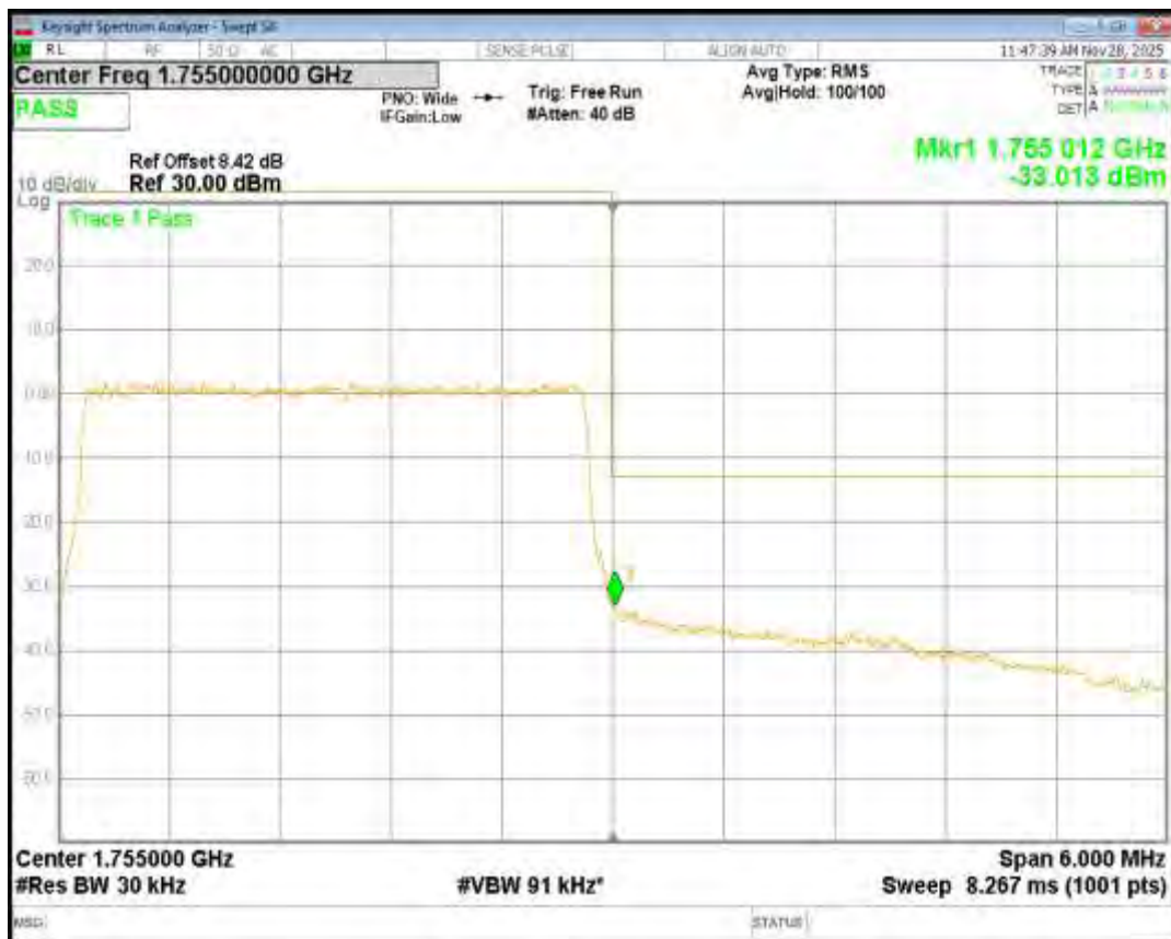
Band4 16QAM BW=5MHz Channel=19975 RB Size=25 Position=#0
