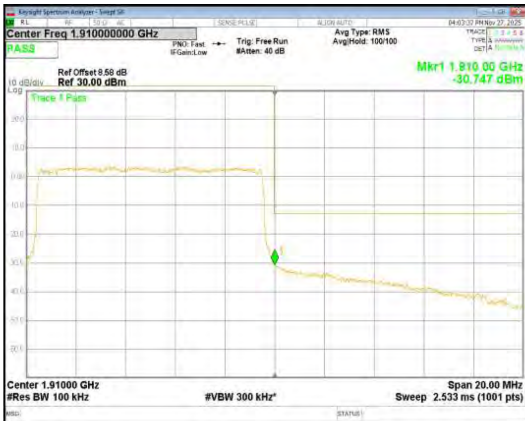
Band2 QPSK BW=15MHz Channel=18675 RB Size=75 Position=#0
