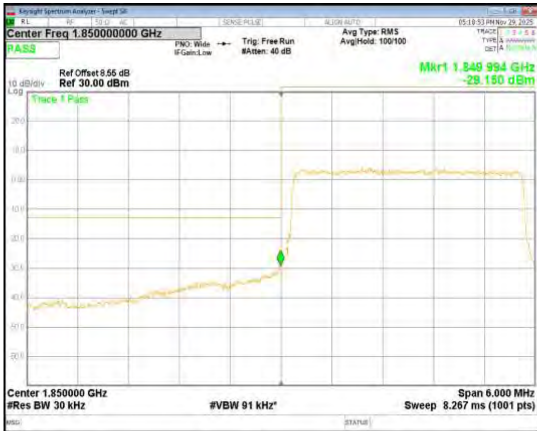
Band25 QPSK BW=3MHz Channel=26675 RB Size=15 Position=#0
