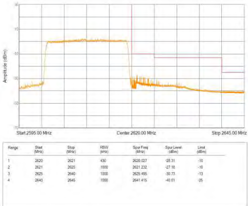
Band38 16QAM BW=5MHz Channel=37775 RB Size=25 Position=#0
