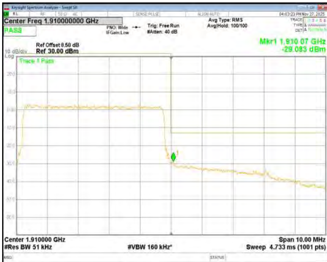
Band2 16QAM BW=20MHz Channel=19100 RB Size=100 Position=#0
