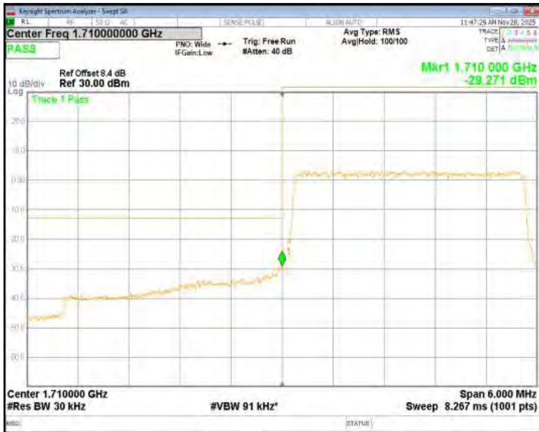
Band4 QPSK BW=5MHz Channel=19975 RB Size=25 Position=#0
