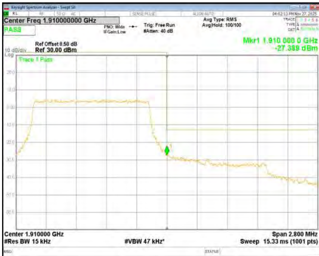
Band2 QPSK BW=10MHz Channel=18650 RB Size=50 Position=#0
