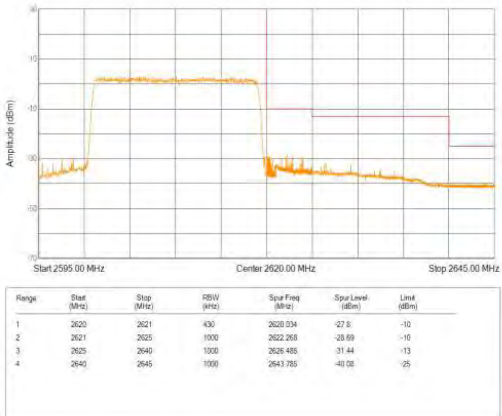
Band38 QPSK BW=5MHz Channel=37775 RB Size=25 Position=#0
