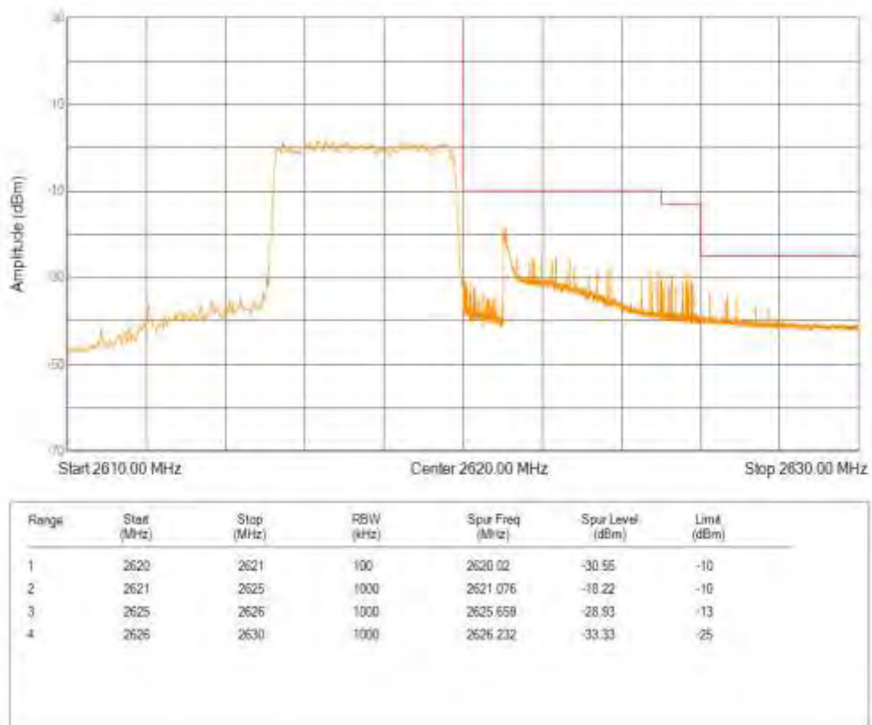
Band38 QPSK BW=10MHz Channel=37800 RB Size=50 Position=#0
