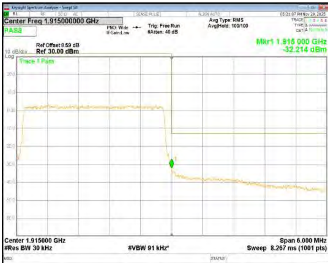
Band25 QPSK BW=1.4MHz Channel=26683 RB Size=6 Position=#0
