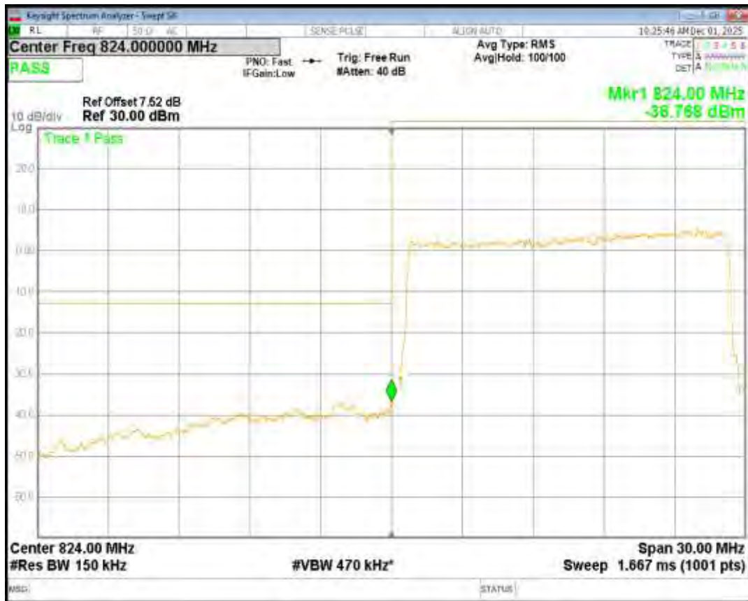
Band26(824-849) QPSK BW=15MHz Channel=26965 RB Size=75 Position=#0
