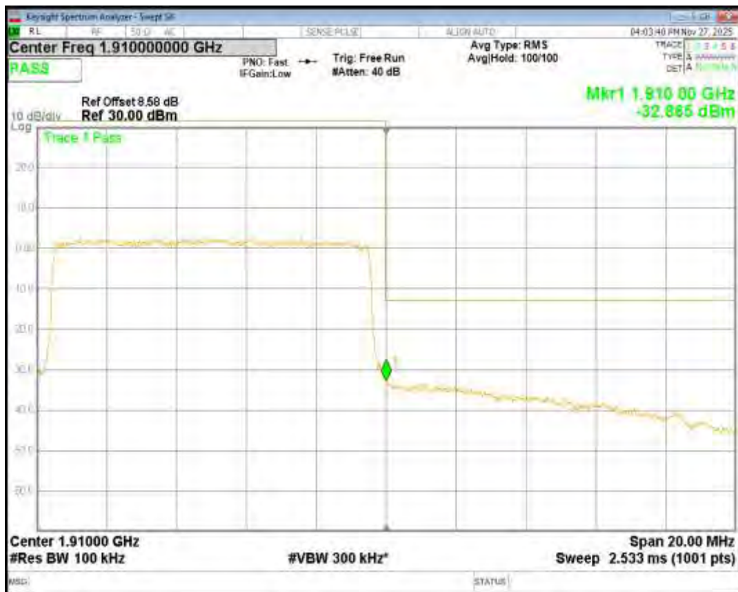
Band2 16QAM BW=15MHz Channel=18675 RB Size=75 Position=#0
