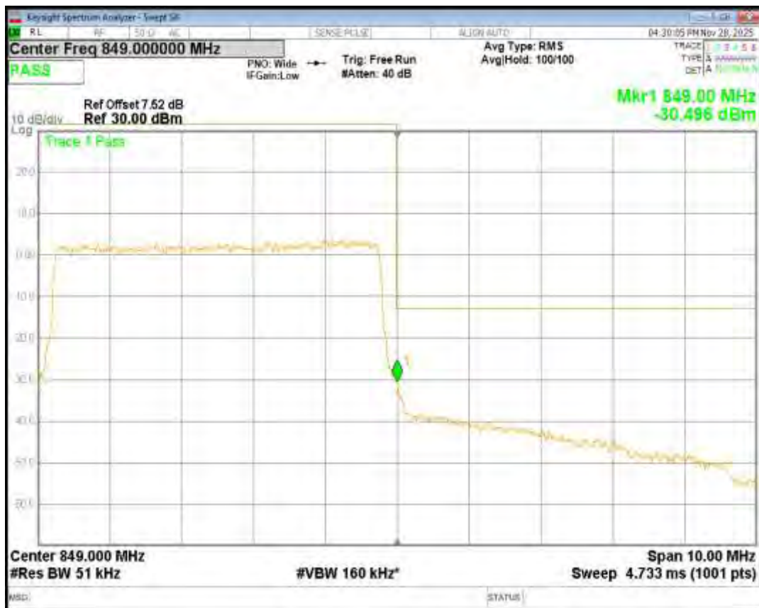
Band5 QPSK BW=1.4MHz Channel=20407 RB Size=6 Position=#0
