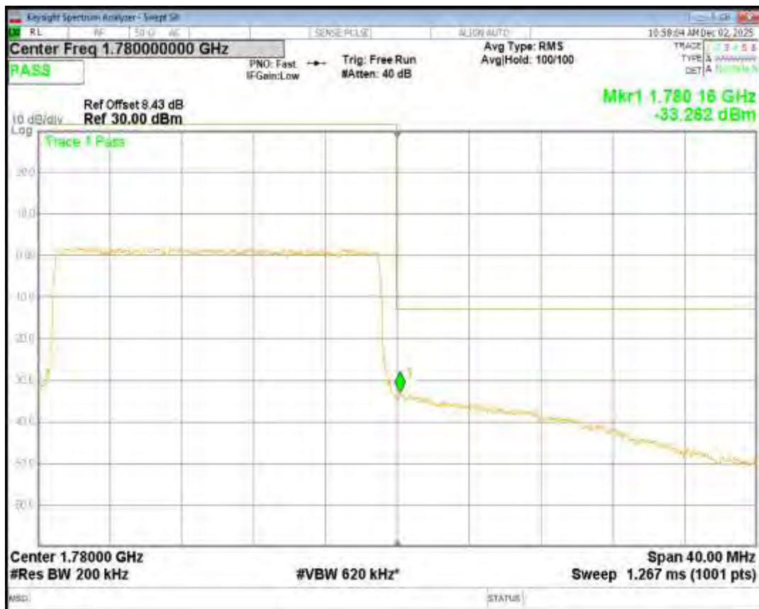
Band66 16QAM BW=3MHz Channel=131987 RB Size=15 Position=#0
