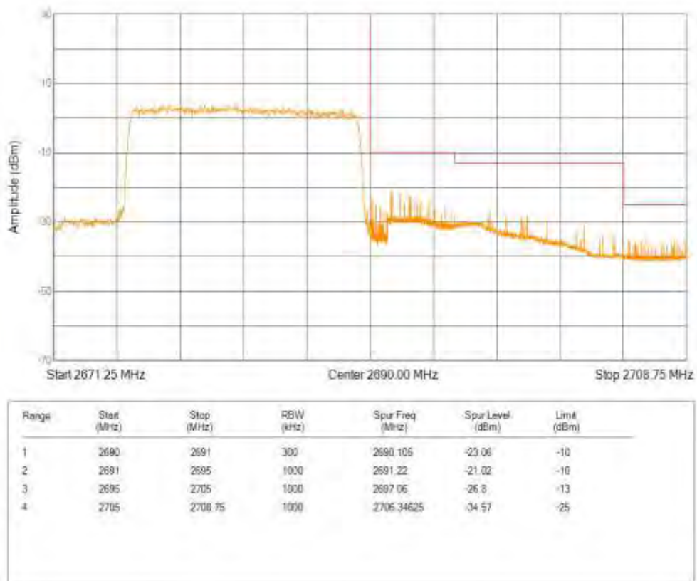
Band41 QPSK BW=20MHz Channel=39750 RB Size=100 Position=#0
