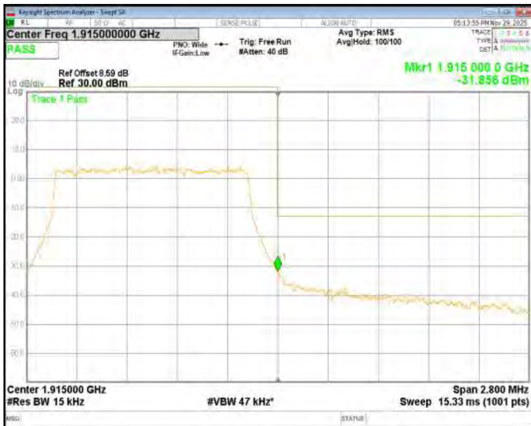
Band25 16QAM BW=10MHz Channel=26090 RB Size=50 Position=#0
