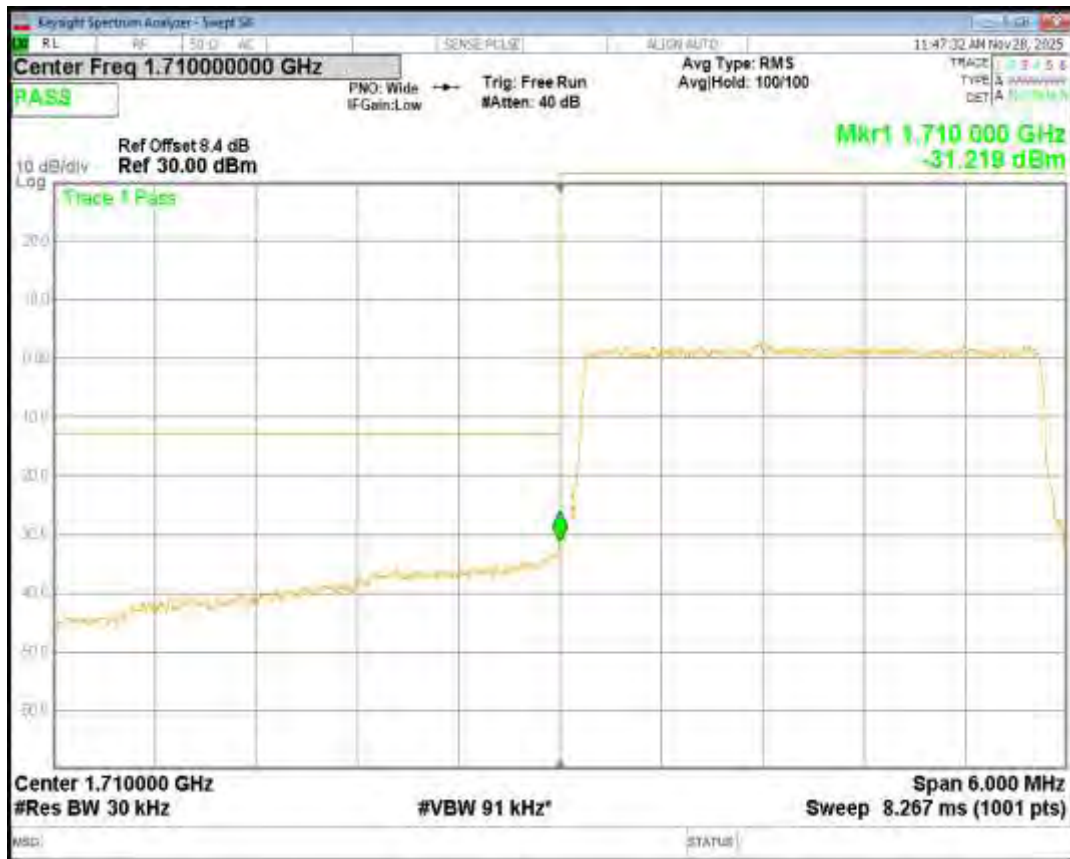
Band4 QPSK BW=1.4MHz Channel=19957 RB Size=6 Position=#0
