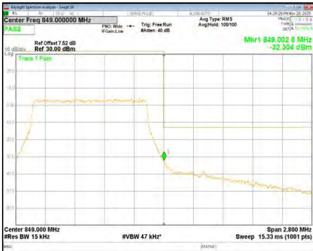
Band5 16QAM BW=10MHz Channel=20450 RB Size=50 Position=#0
