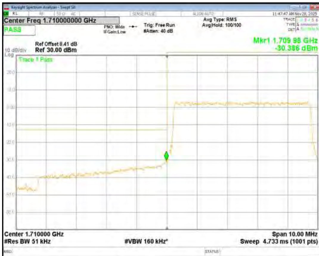
Band4 QPSK BW=3MHz Channel=20385 RB Size=15 Position=#0
