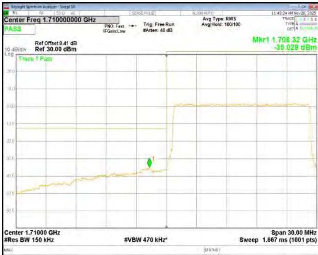
Band4 16QAM BW=15MHz Channel=20325 RB Size=75 Position=#0
