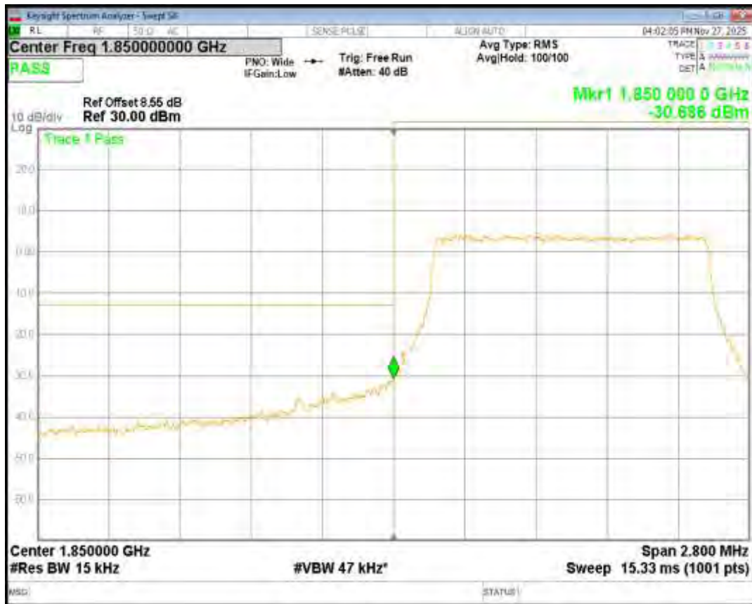
Band2 QPSK BW=1.4MHz Channel=19193 RB Size=6 Position=#0
