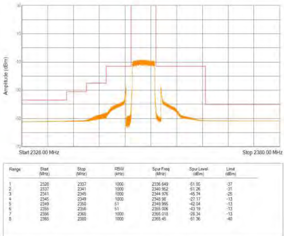
Band40(2350-2360) QPSK BW=5MHz Channel=39225 RB Size=25 Position=#0
