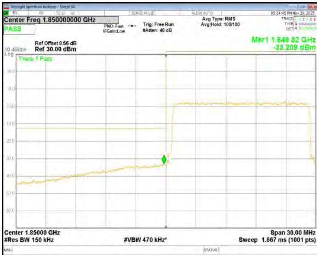
Band25 16QAM BW=15MHz Channel=26615 RB Size=75 Position=#0
