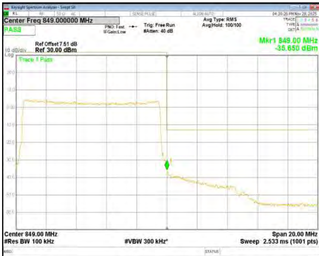
Band5 QPSK BW=3MHz Channel=20415 RB Size=15 Position=#0
