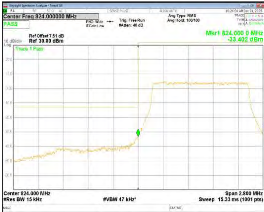
Band26(824-849) 16QAM BW=5MHz Channel=26815 RB Size=25 Position=#0
