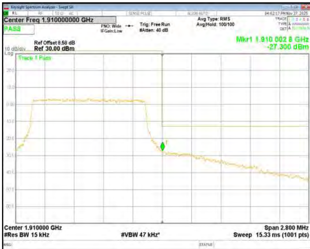
Band2 16QAM BW=10MHz Channel=18650 RB Size=50 Position=#0
