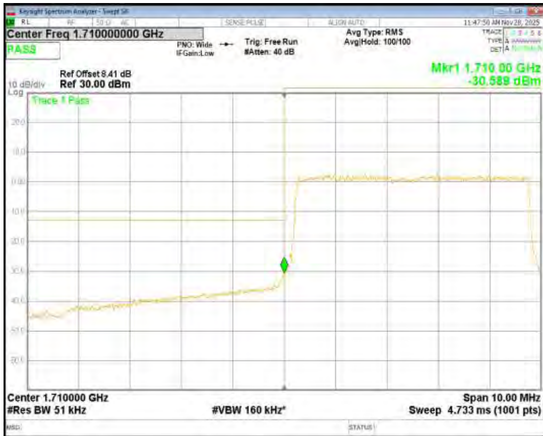
Band4 QPSK BW=1.4MHz Channel=20393 RB Size=6 Position=#0
