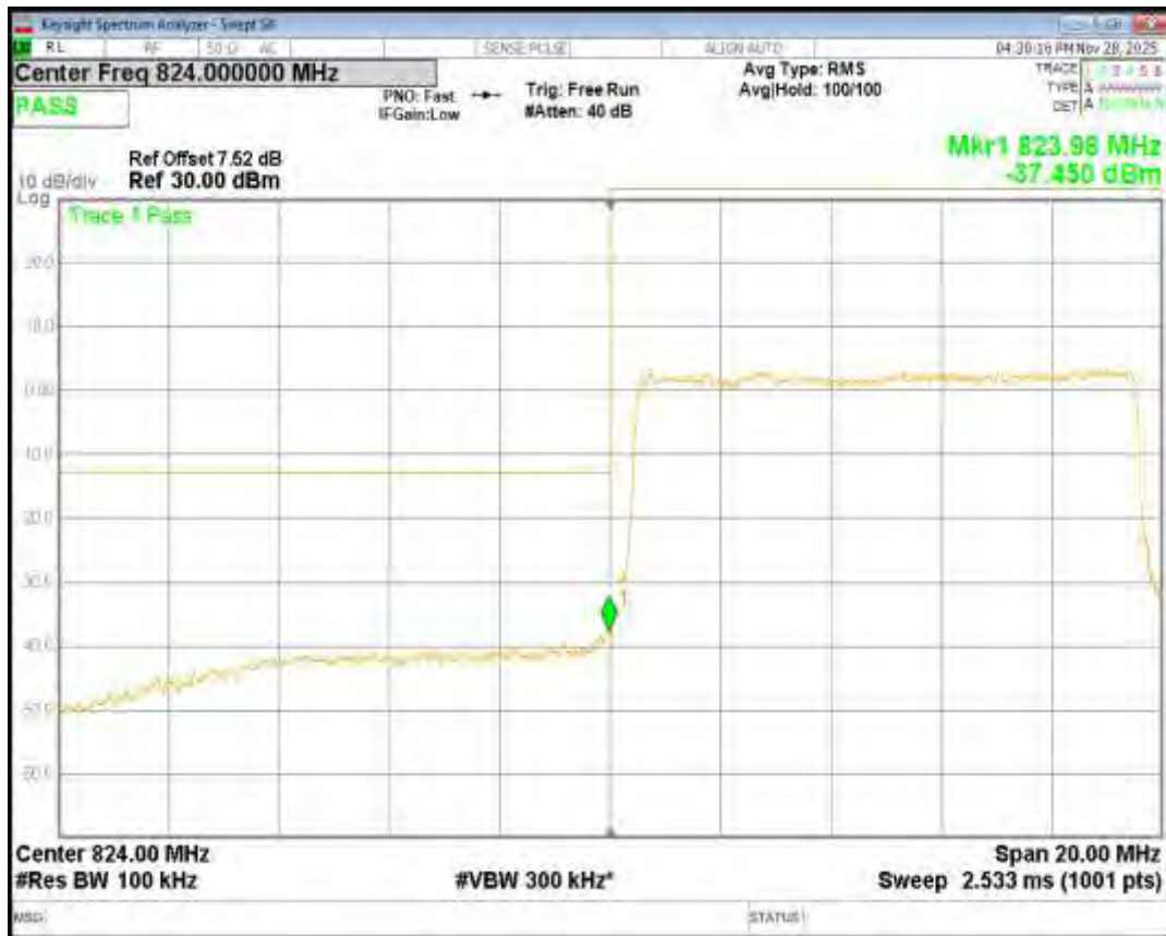
Band5 16QAM BW=10MHz Channel=20600 RB Size=50 Position=#0
