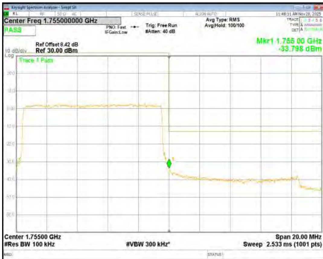
Band4 QPSK BW=15MHz Channel=20025 RB Size=75 Position=#0
