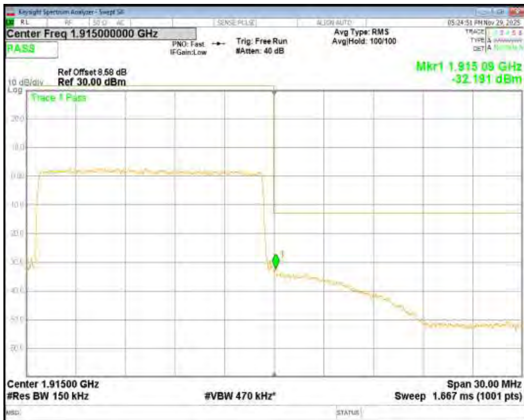
Band25 16QAM BW=20MHz Channel=26140 RB Size=100 Position=#0
