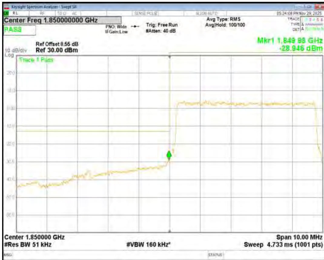
Band25 QPSK BW=5MHz Channel=26665 RB Size=25 Position=#0
