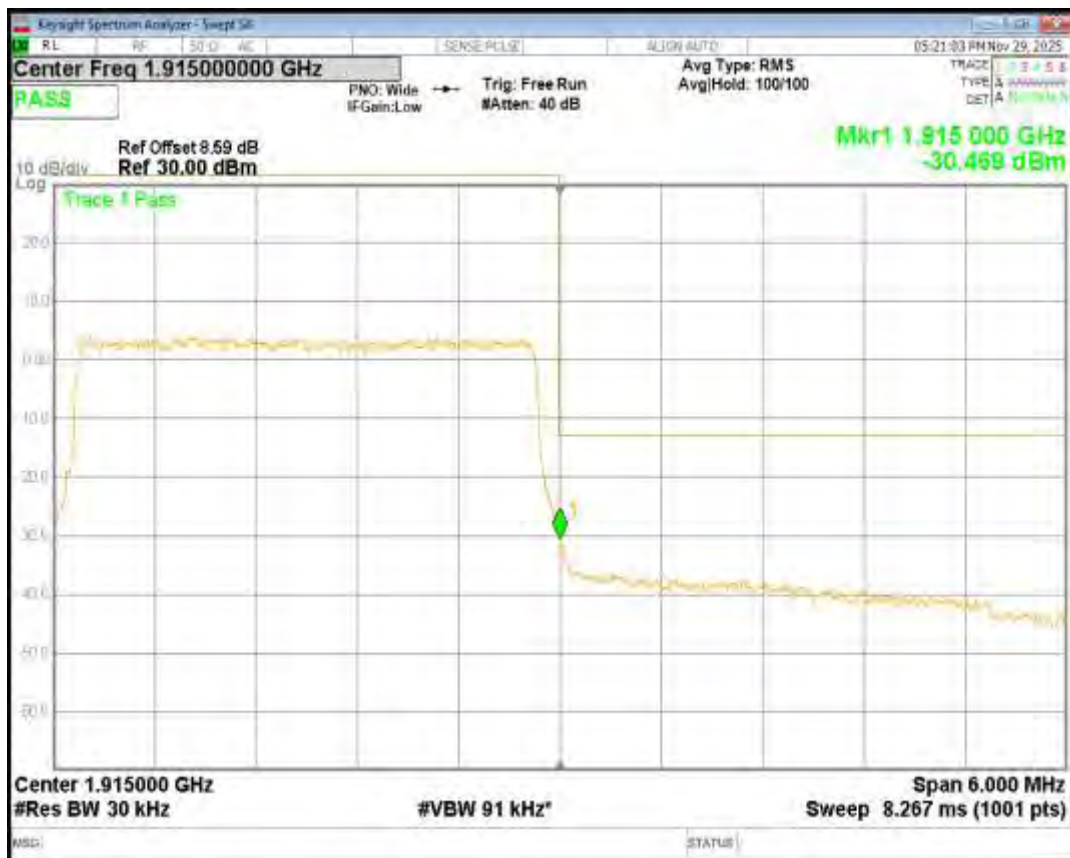
Band25 QPSK BW=5MHz Channel=26065 RB Size=25 Position=#0
