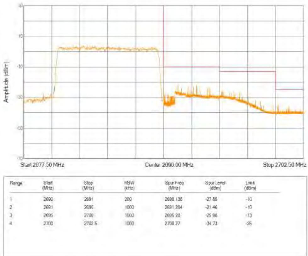
Band41 QPSK BW=15MHz Channel=39725 RB Size=75 Position=#0
