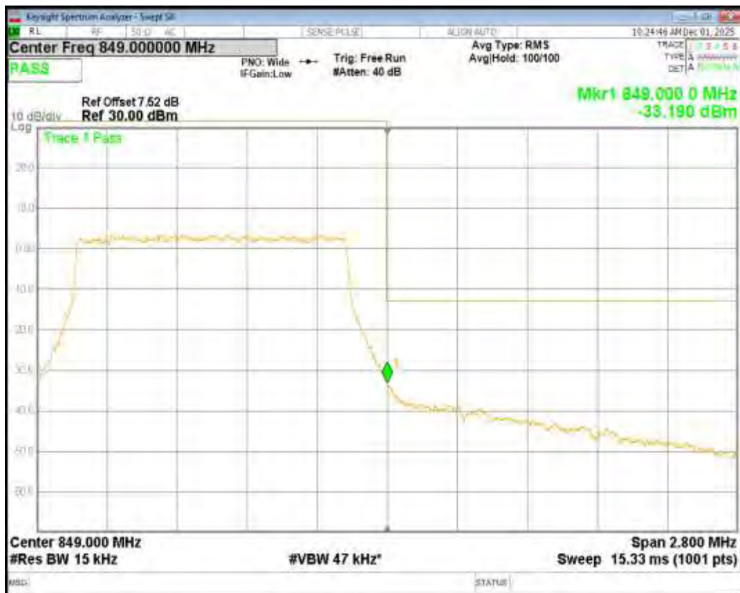
Band26(824-849) 16QAM BW=10MHz Channel=26840 RB Size=50 Position=#0
