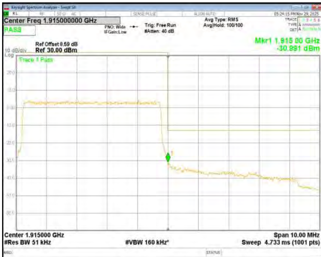
Band26(814-824) 16QAM BW=1.4MHz Channel=26697 RB Size=6 Position=#0
