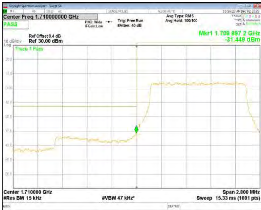
Band66 16QAM BW=5MHz Channel=132647 RB Size=25 Position=#0
