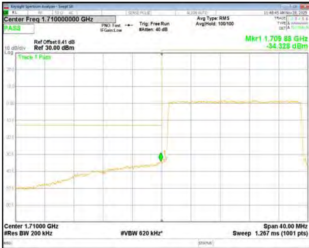
Band4 16QAM BW=20MHz Channel=20300 RB Size=100 Position=#0
