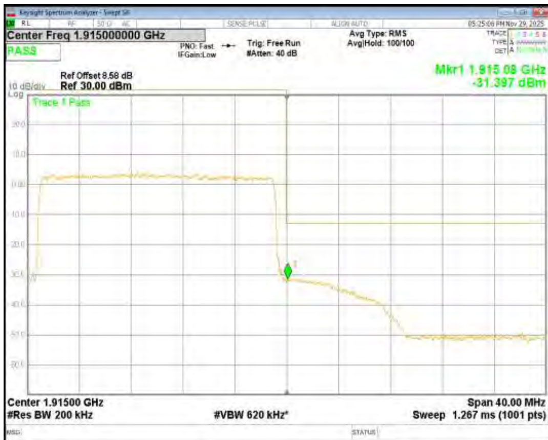
Band25 QPSK BW=3MHz Channel=26055 RB Size=15 Position=#0
