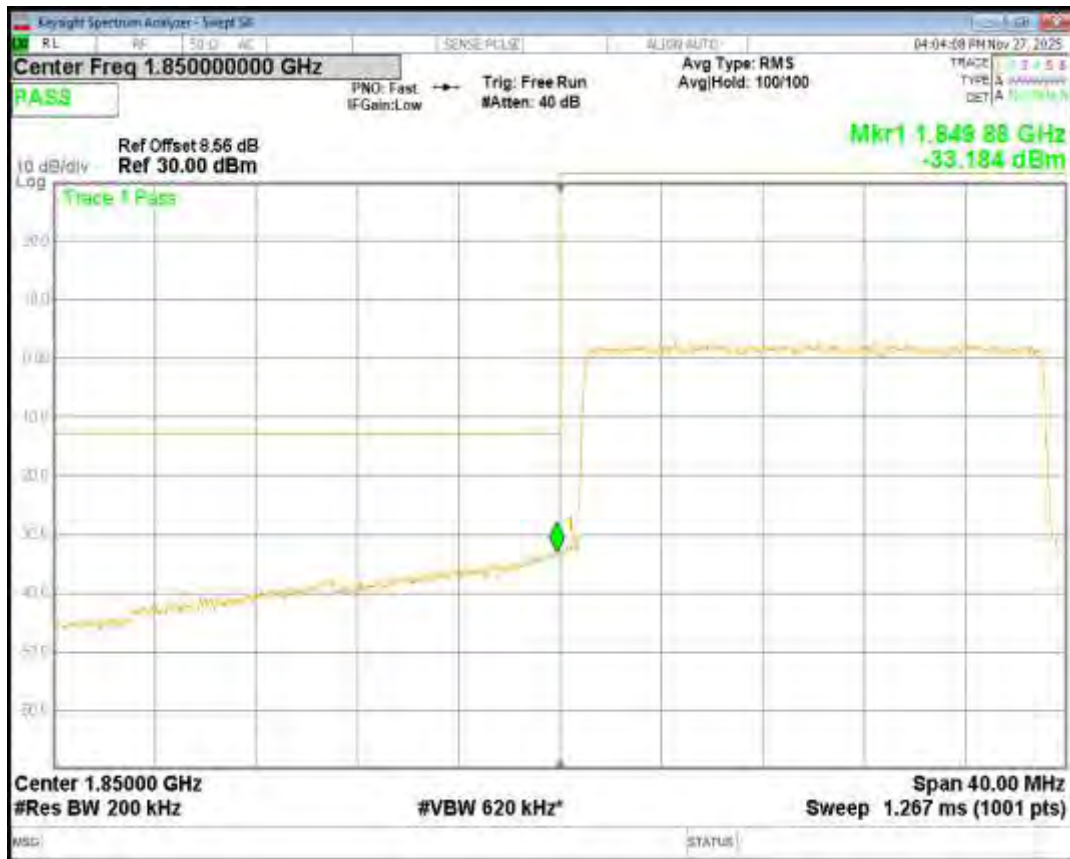
Band2 16QAM BW=5MHz Channel=18625 RB Size=25 Position=#0
