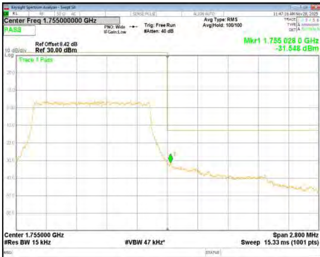
Band4 QPSK BW=10MHz Channel=20000 RB Size=50 Position=#0
