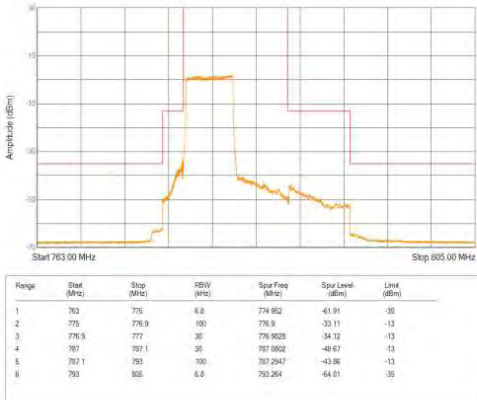
Band13 QPSK BW=5MHz Channel=23255 RB Size=25 Position=#0
