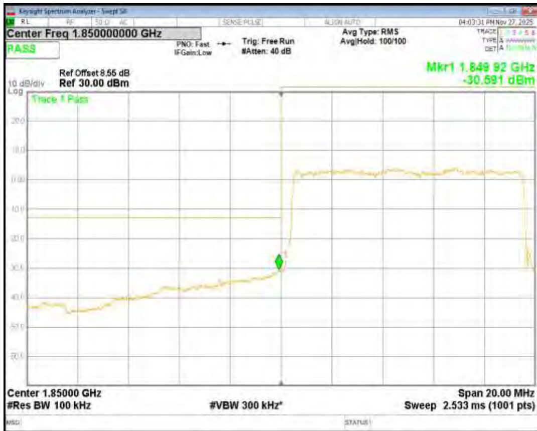
Band2 QPSK BW=10MHz Channel=19150 RB Size=50 Position=#0
