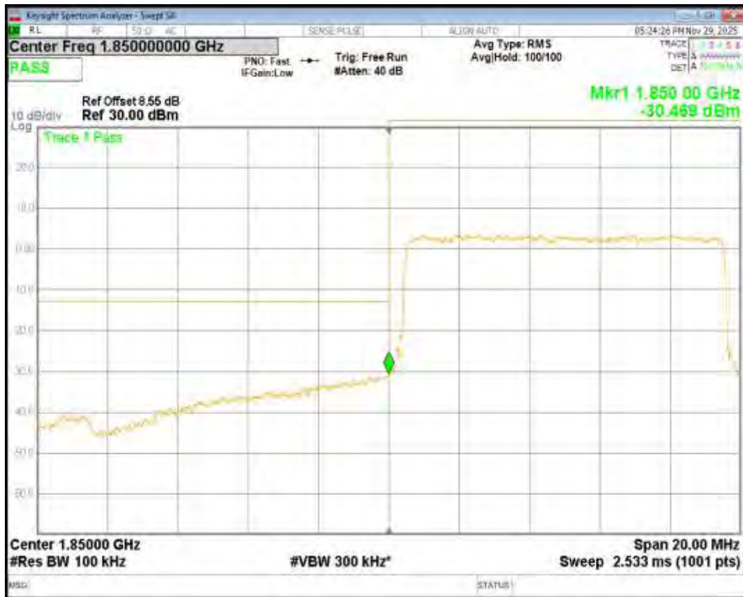
Band25 QPSK BW=10MHz Channel=26640 RB Size=50 Position=#0
