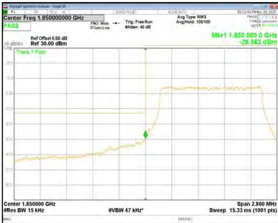
Band25 16QAM BW=5MHz Channel=26665 RB Size=25 Position=#0
