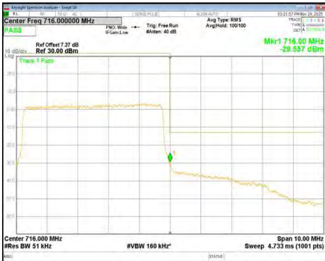
Band17 QPSK BW=10MHz Channel=23780 RB Size=50 Position=#0
