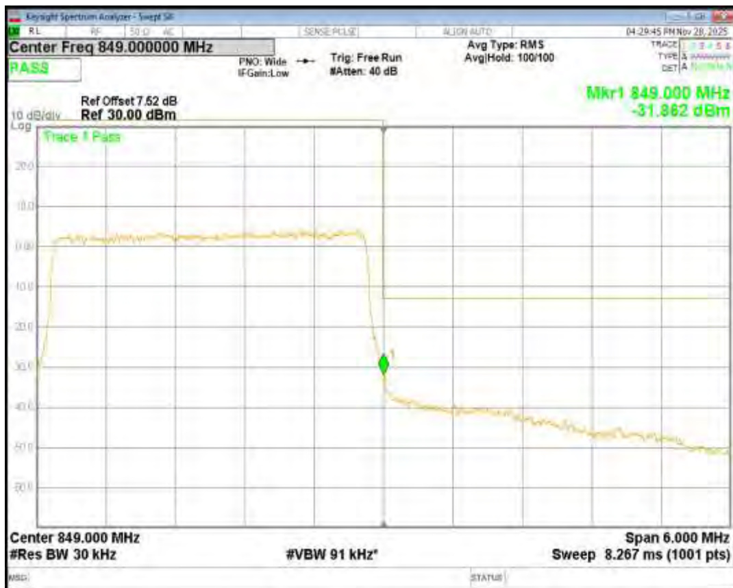
Band5 QPSK BW=5MHz Channel=20425 RB Size=25 Position=#0
