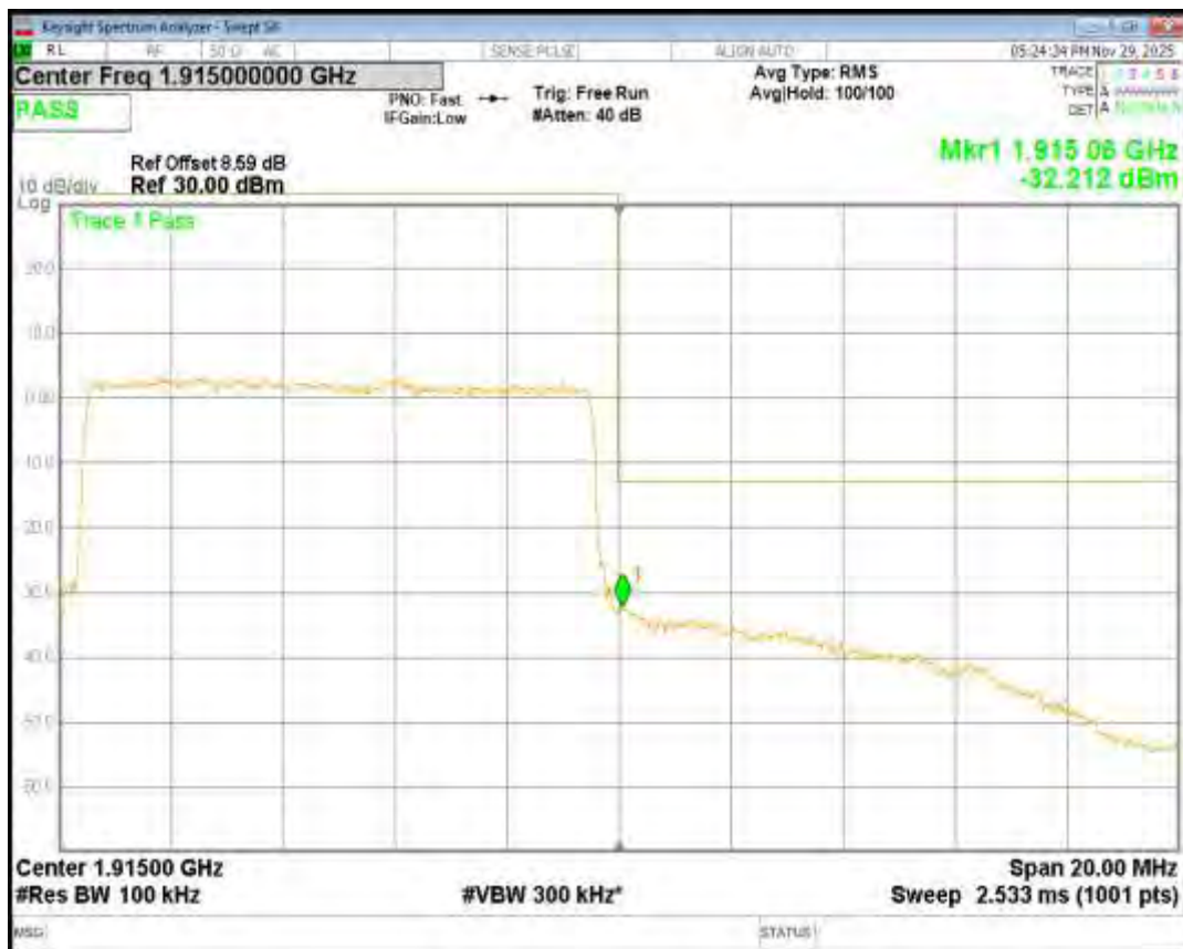
Band25 16QAM BW=15MHz Channel=26115 RB Size=75 Position=#0
