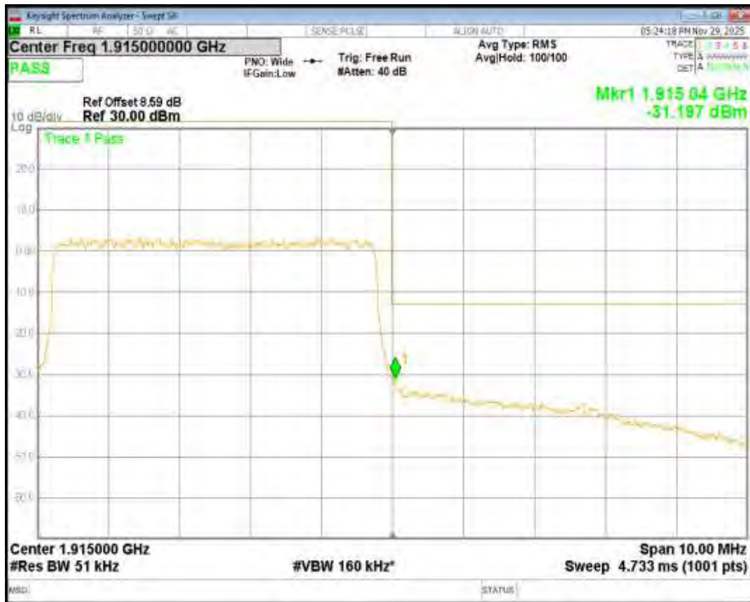
Band25 16QAM BW=5MHz Channel=26065 RB Size=25 Position=#0
