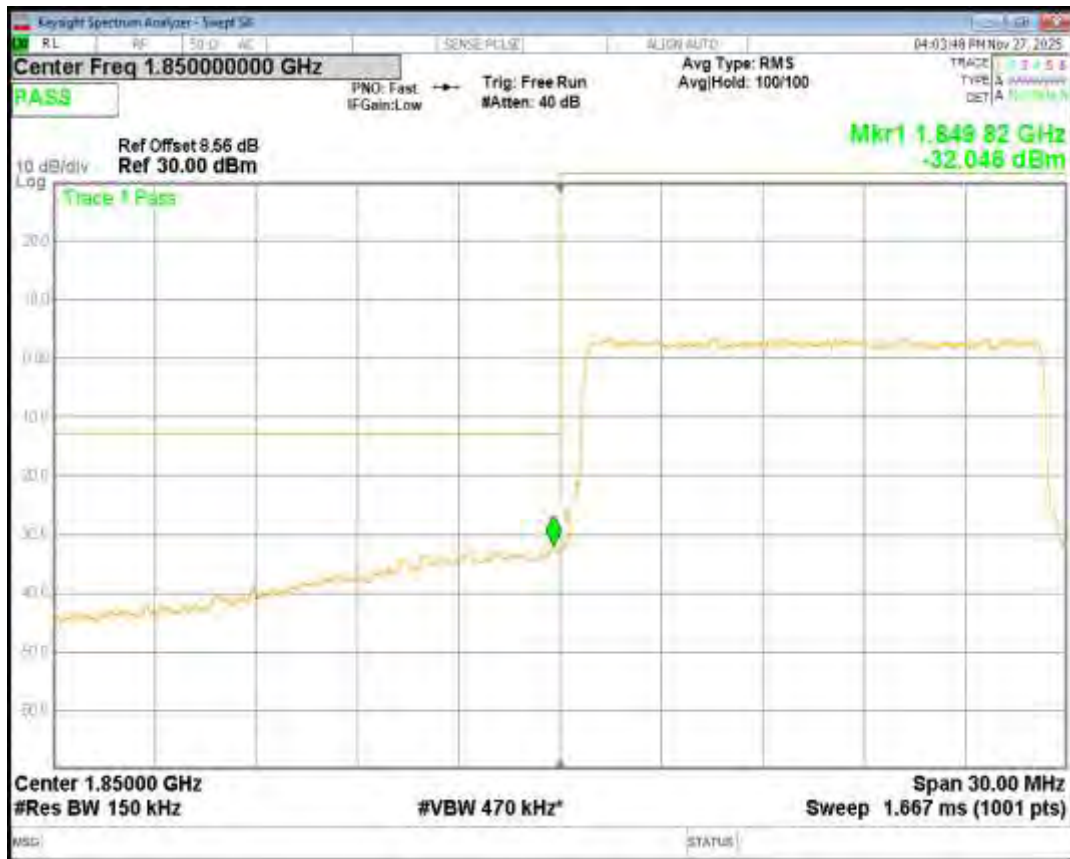
Band2 QPSK BW=15MHz Channel=19125 RB Size=75 Position=#0
