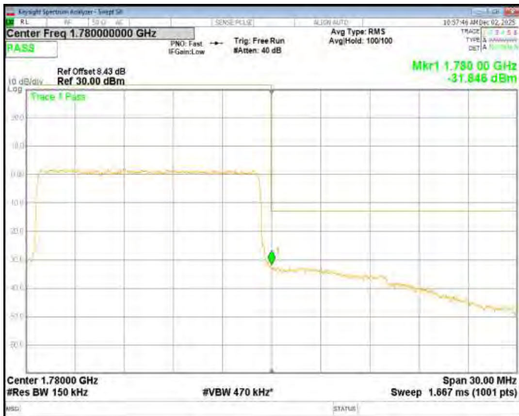
Band66 16QAM BW=20MHz Channel=132072 RB Size=100 Position=#0
