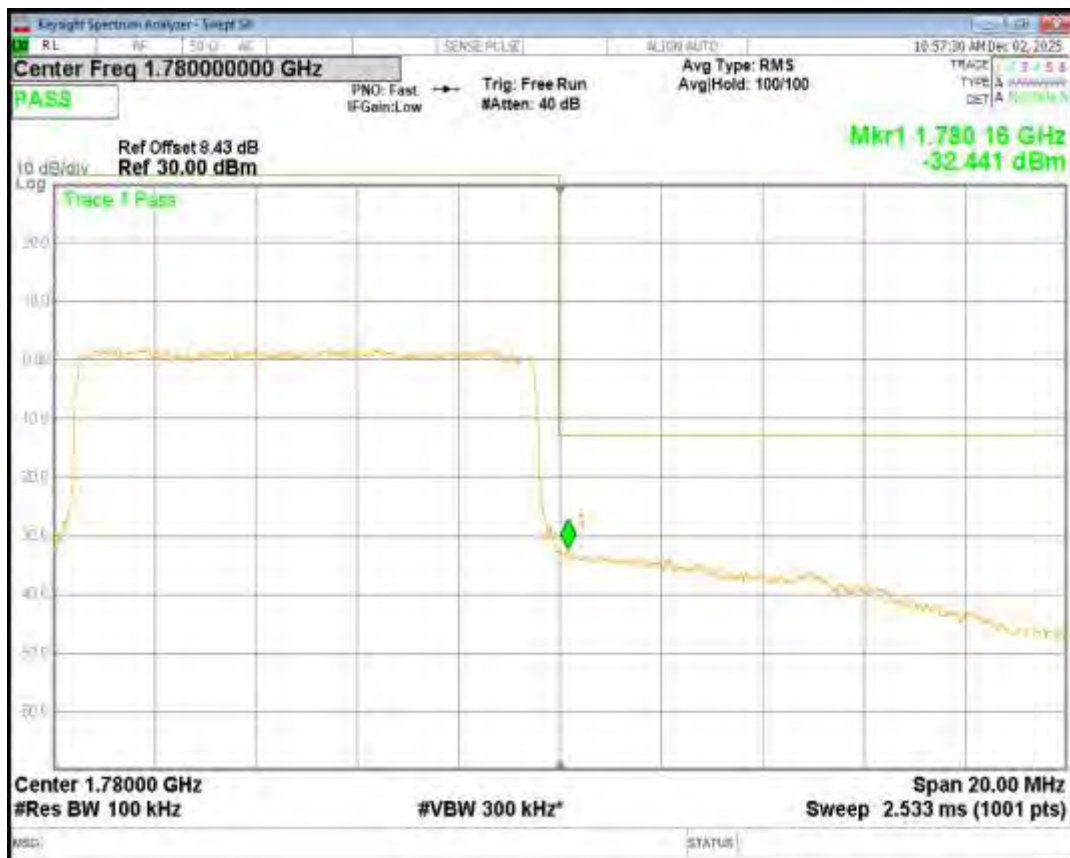
Band66 16QAM BW=15MHz Channel=132047 RB Size=75 Position=#0
