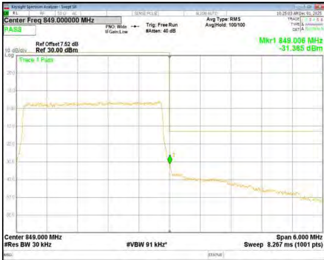
Band26(824-849) QPSK BW=5MHz Channel=27015 RB Size=25 Position=#0
