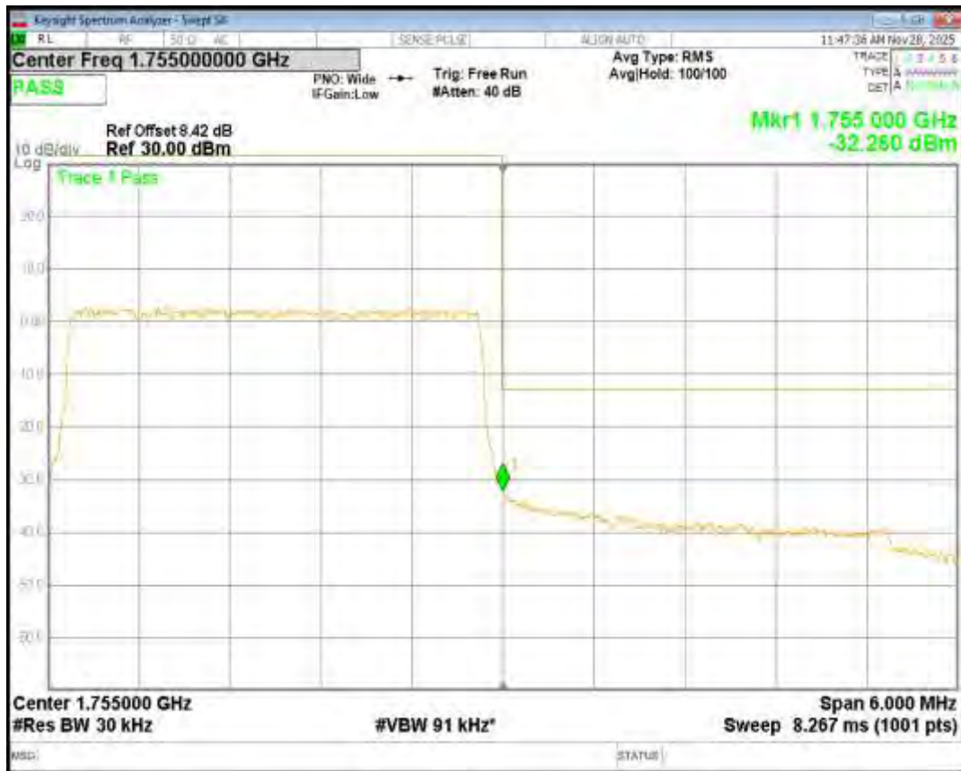
Band4 QPSK BW=5MHz Channel=20375 RB Size=25 Position=#0
