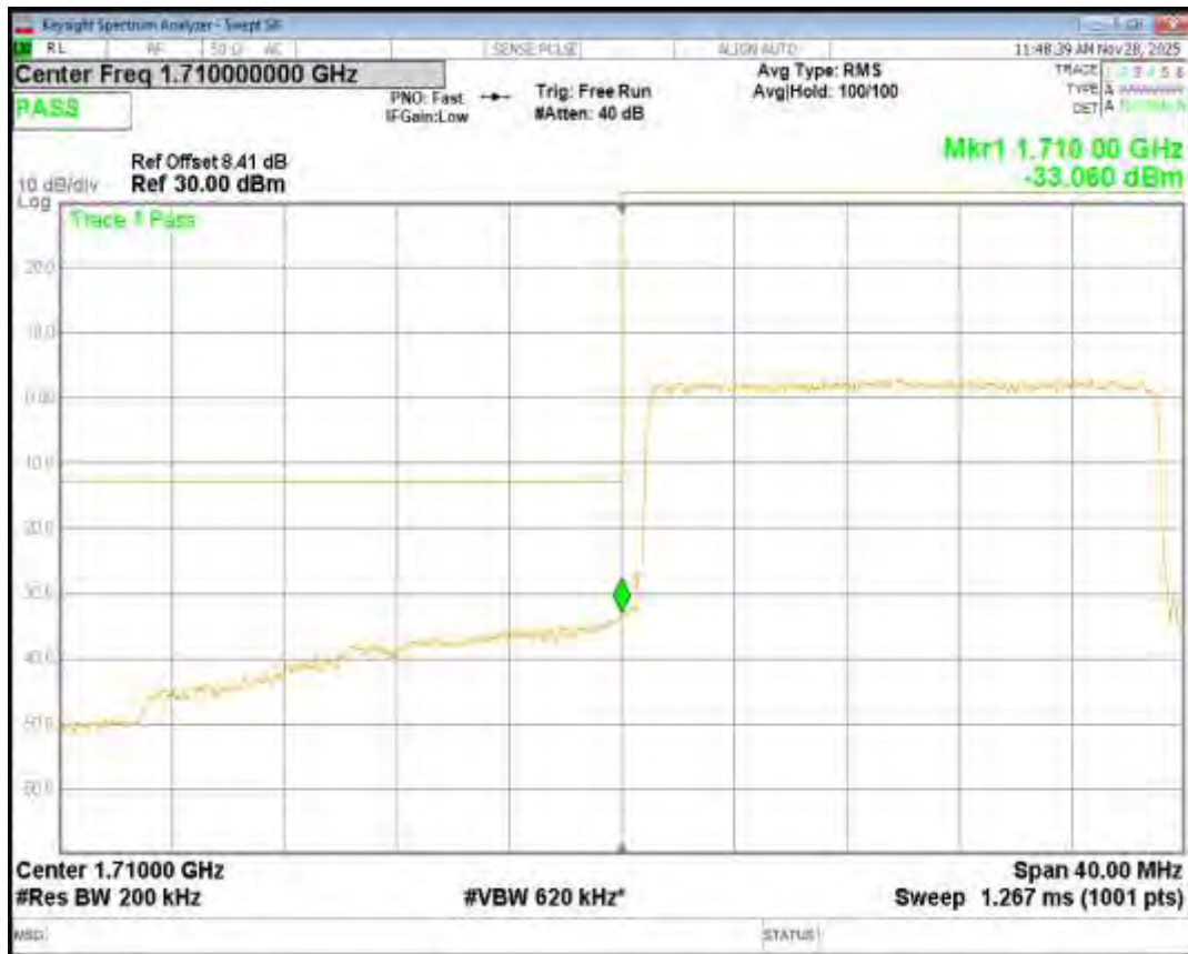
Band4 QPSK BW=20MHz Channel=20300 RB Size=100 Position=#0
