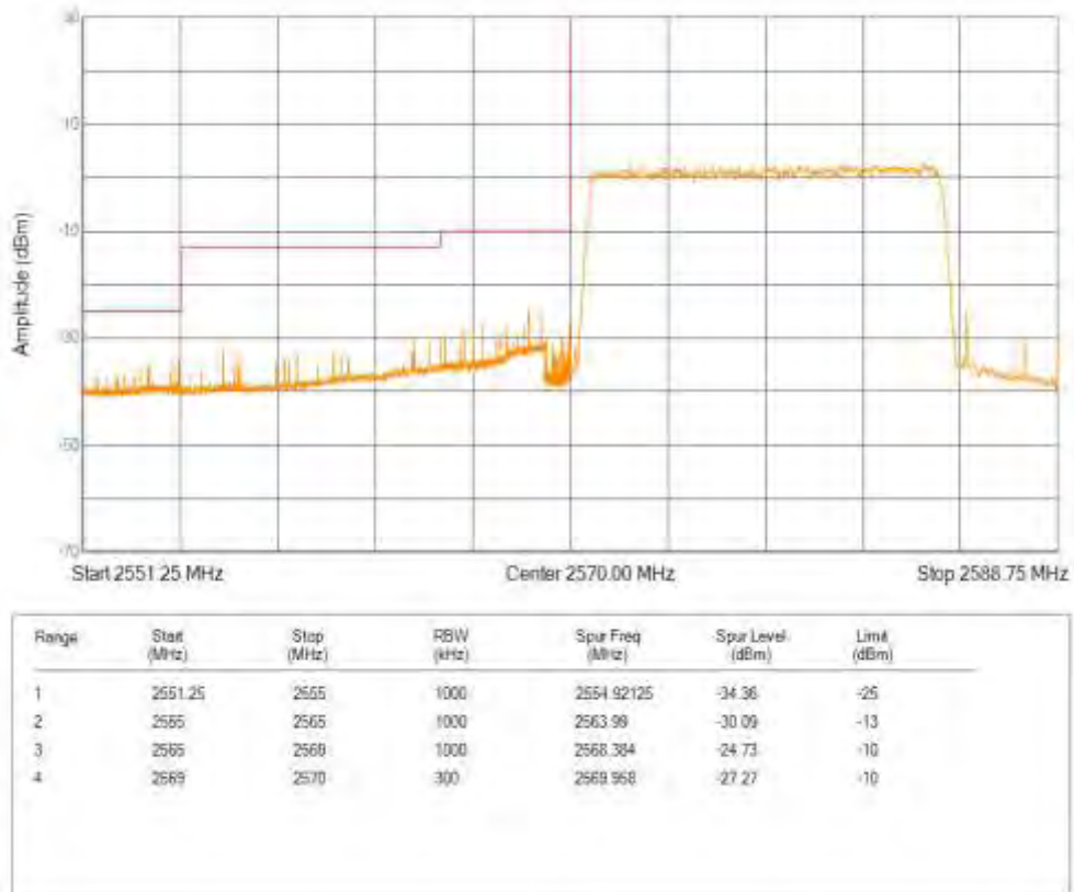
Band38 QPSK BW=15MHz Channel=38175 RB Size=75 Position=#0
