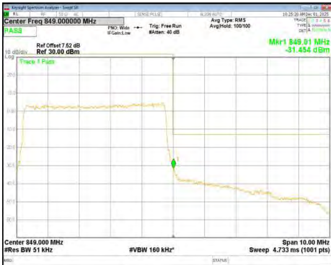
Band38 16QAM BW=10MHz Channel=37800 RB Size=50 Position=#0
