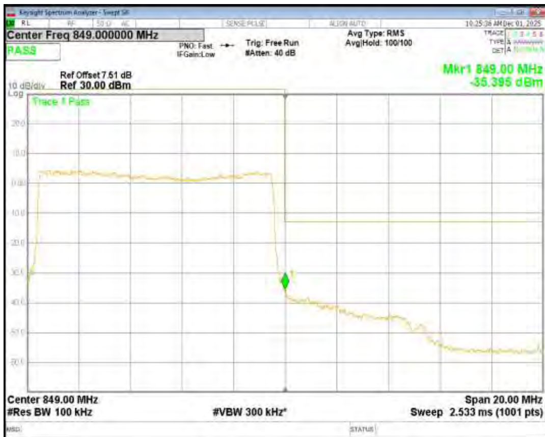
Band26(824-849) QPSK BW=15MHz Channel=26865 RB Size=75 Position=#0
