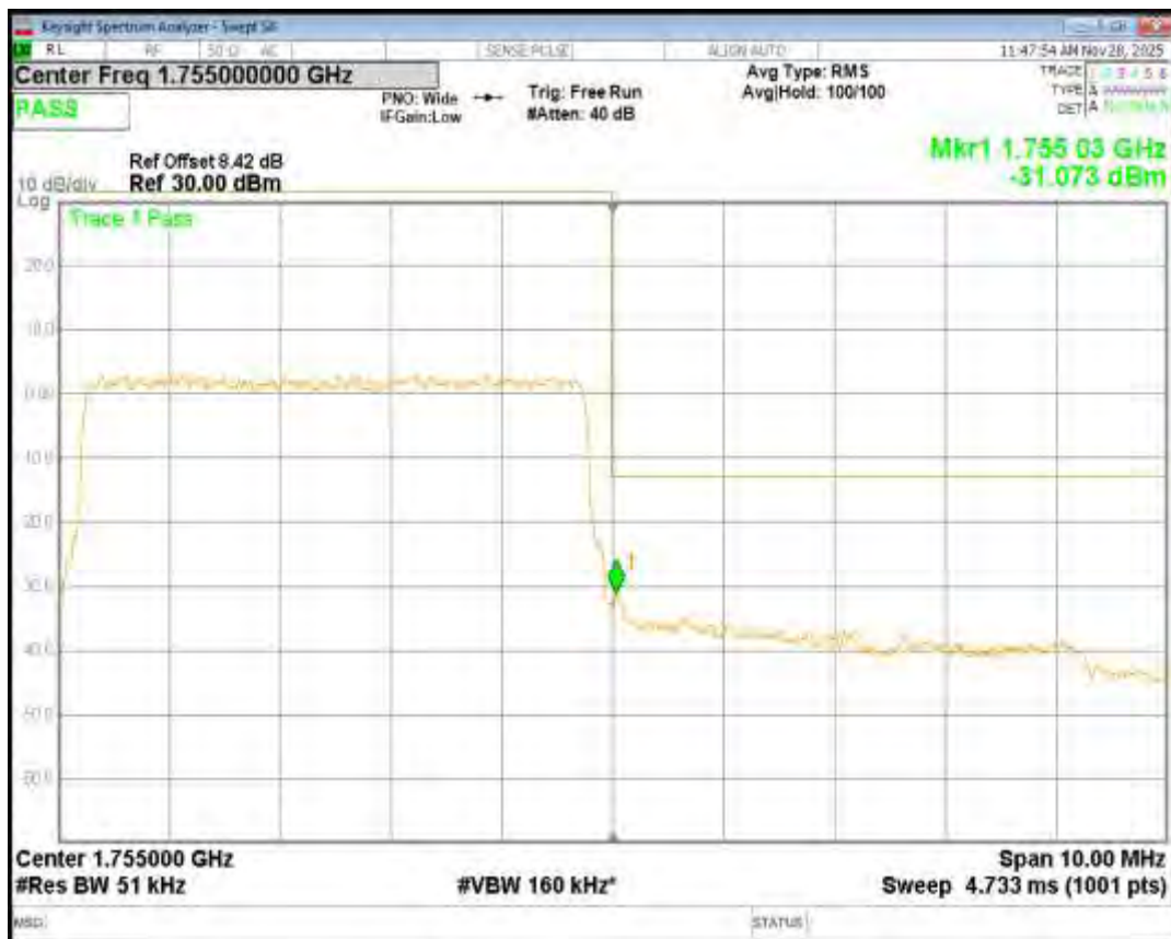
Band40(2305-2315) 16QAM BW=10MHz Channel=38750 RB Size=50 Position=#0
