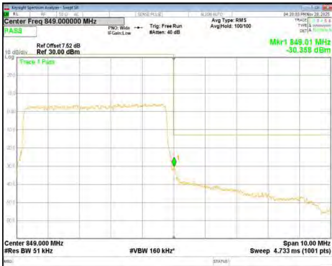
Band66 16QAM BW=1.4MHz Channel=131979 RB Size=6 Position=#0
