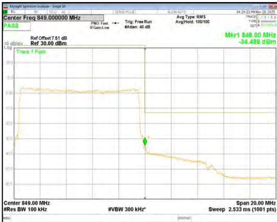
Band5 16QAM BW=3MHz Channel=20415 RB Size=15 Position=#0
