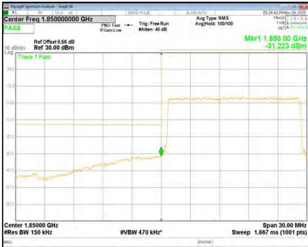
Band25 QPSK BW=15MHz Channel=26615 RB Size=75 Position=#0
