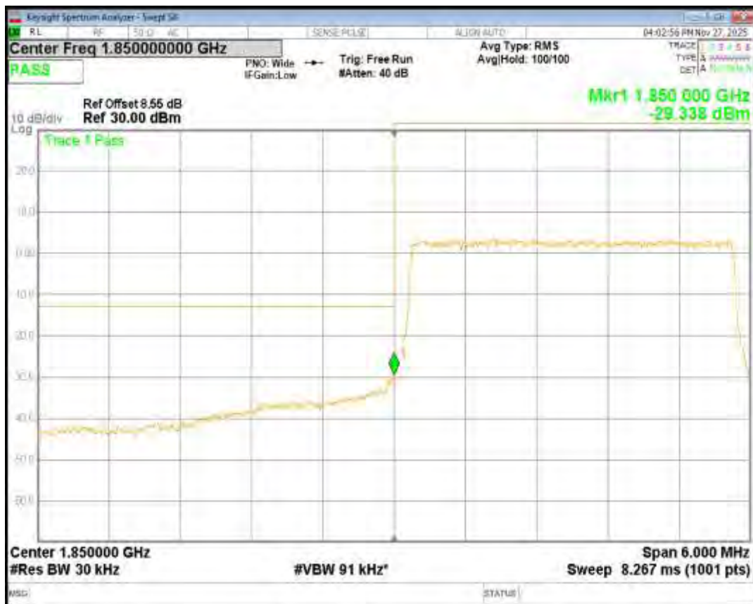
Band2 QPSK BW=3MHz Channel=19185 RB Size=15 Position=#0
