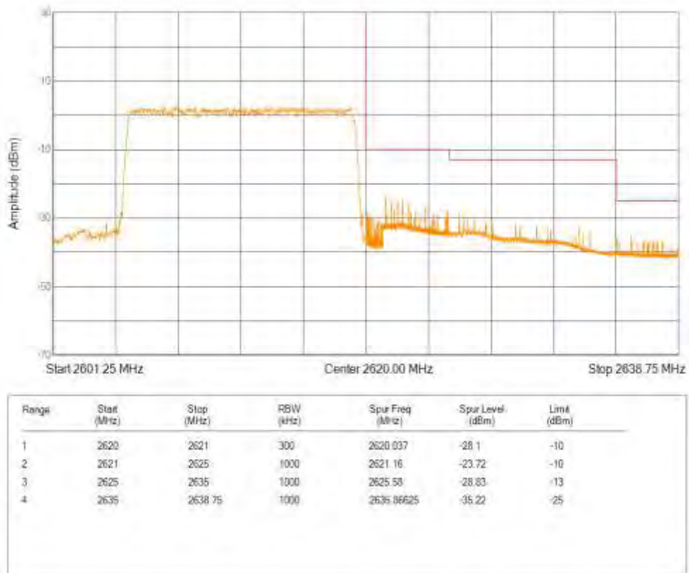
Band38 QPSK BW=20MHz Channel=37850 RB Size=100 Position=#0
