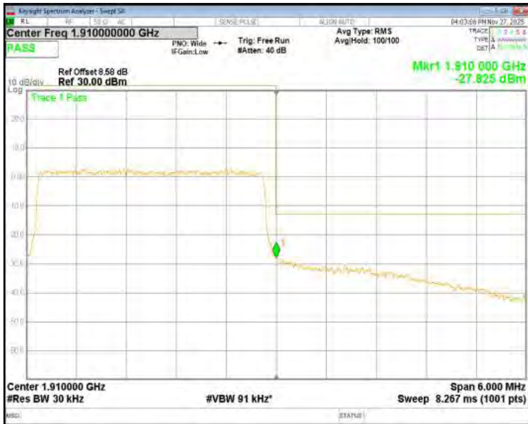
Band2 16QAM BW=5MHz Channel=19175 RB Size=25 Position=#0
