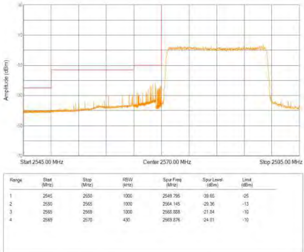
Band38 QPSK BW=20MHz Channel=38150 RB Size=100 Position=#0
