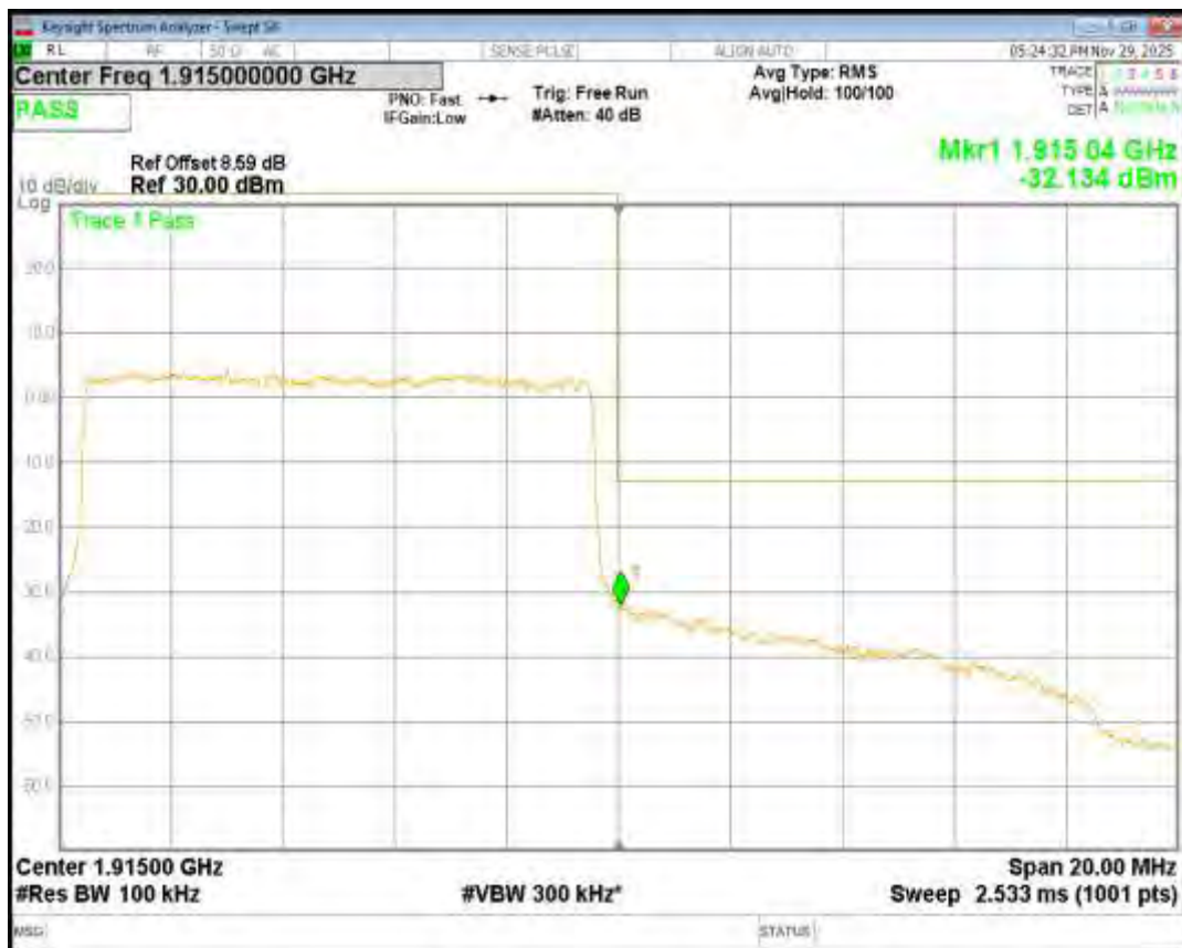
Band25 QPSK BW=15MHz Channel=26115 RB Size=75 Position=#0
