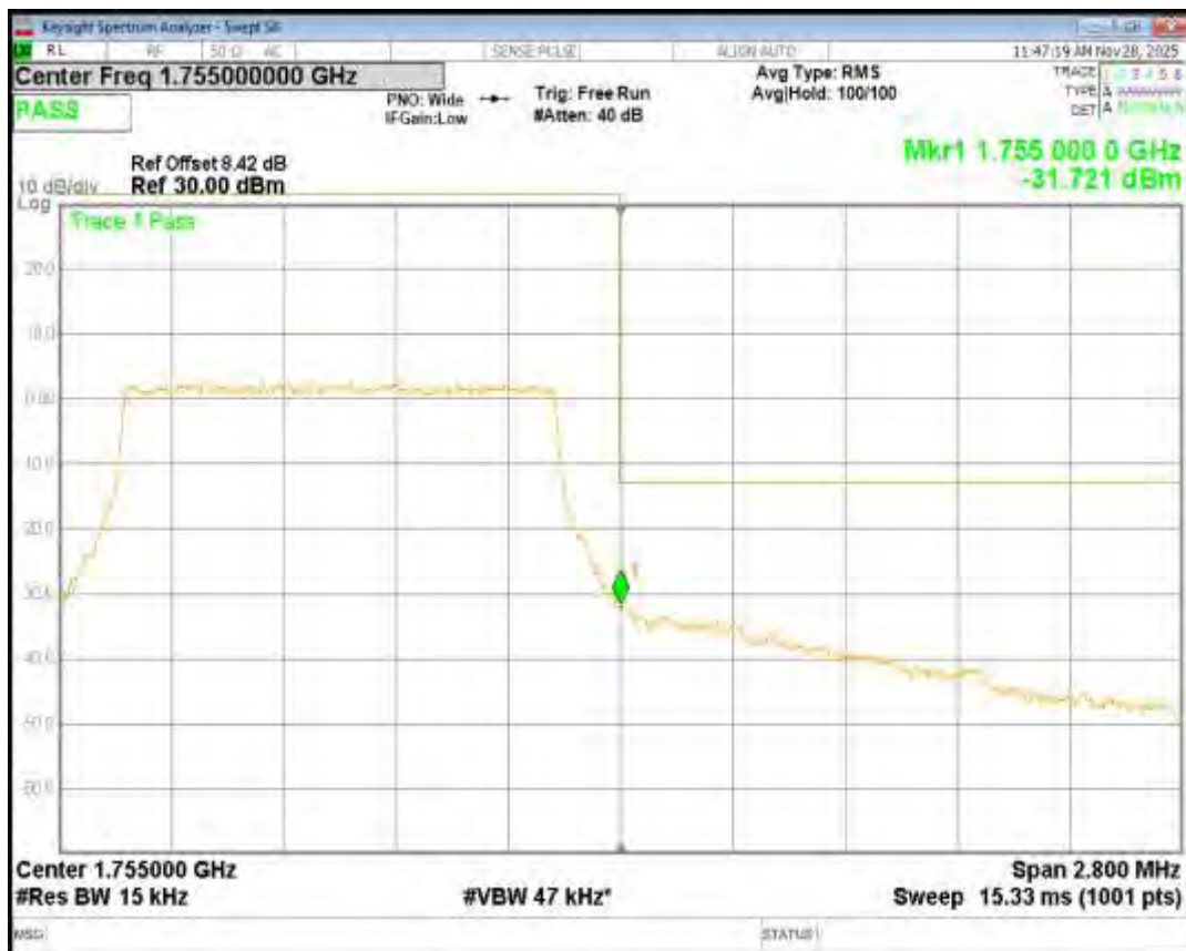
Band4 16QAM BW=10MHz Channel=20000 RB Size=50 Position=#0
