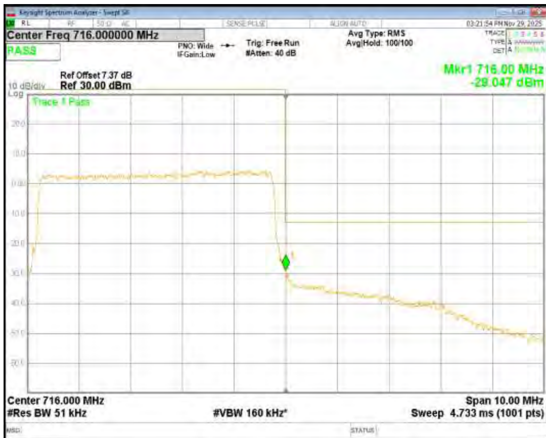
Band2 16QAM BW=1.4MHz Channel=18607 RB Size=6 Position=#0
