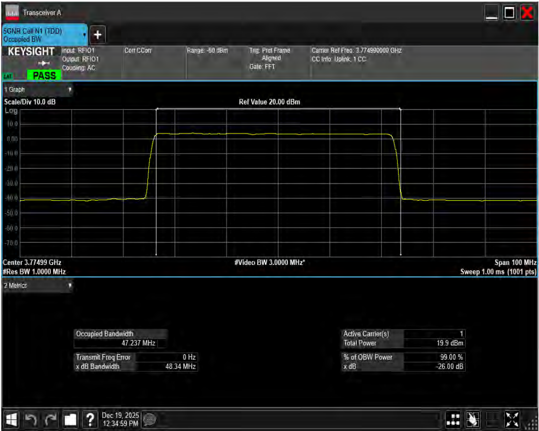
n78(3700-3800) SCS=30kHz DFT QPSK BW=100MHz Channel=650000 RB=270@0
