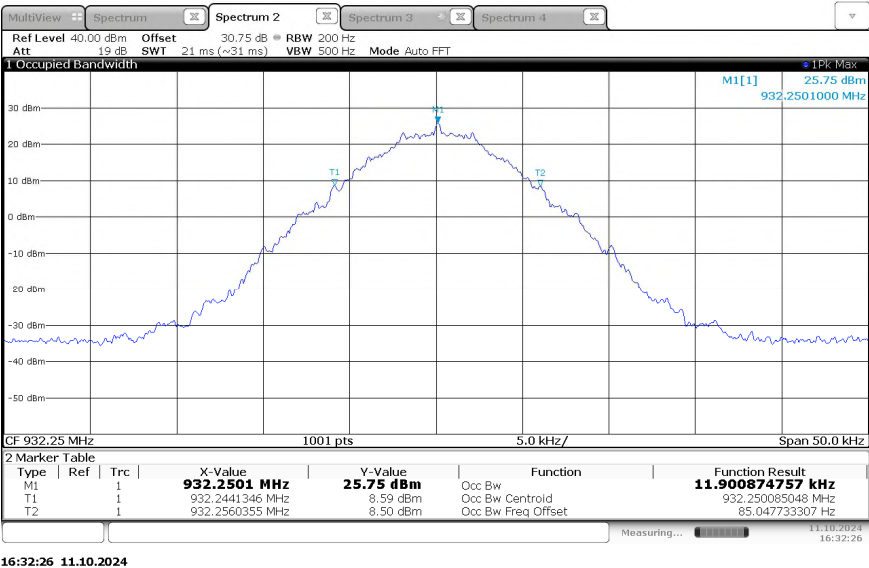
Figure 2.3.6-13 - 99% Bandwidth – TXC TCXO – 932.25 MHz - Normal Mode
