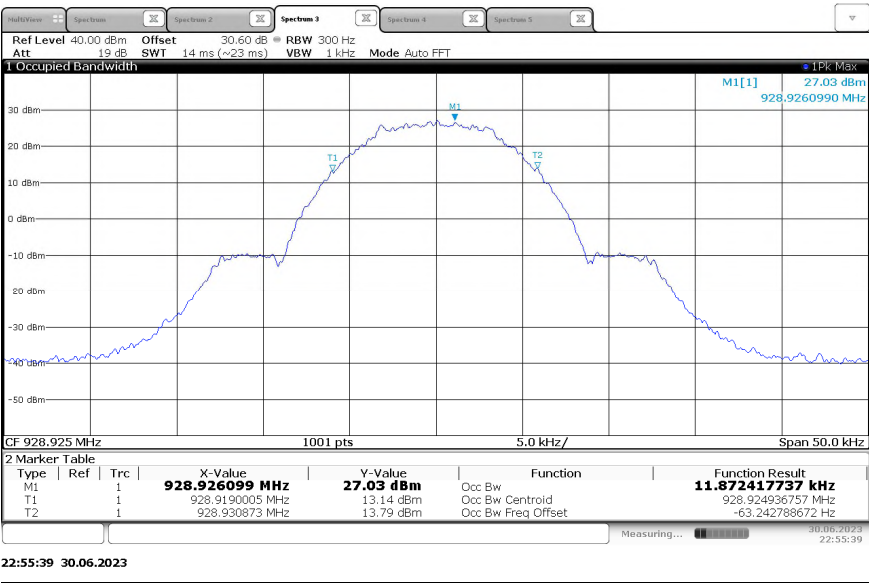
Figure 2.3.6-18 - 99% Bandwidth – KDS TCXO – 928.925 MHz - 2FSK Mode
