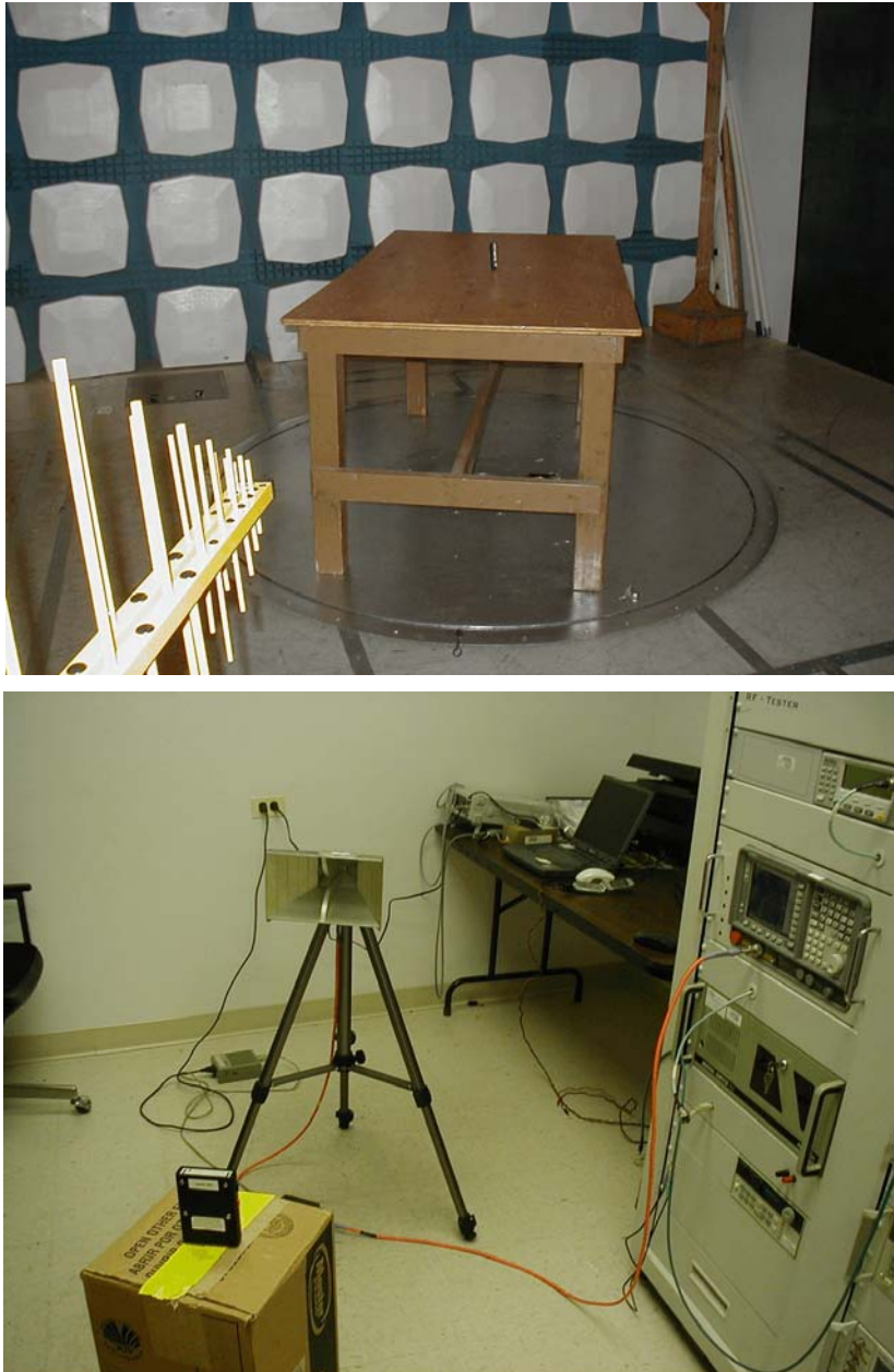
Figure 1. FCC Intentional Radiators Test Setup Photo
