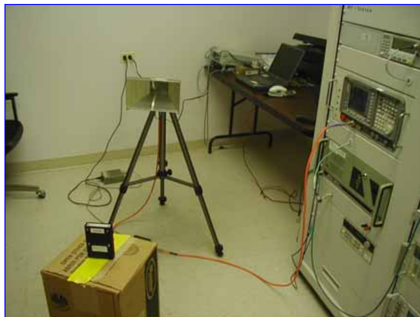
Photograph 1. Radiated Emission Limits Test Setup Photos
