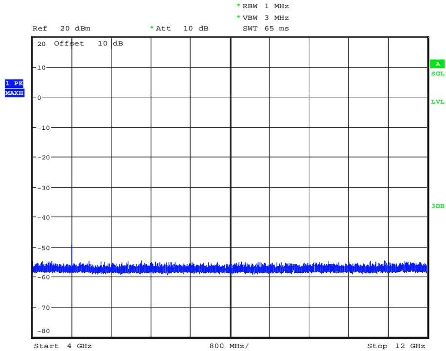
170297\_SpurEmiss12-18G\_BT\_DH5\_BT1.wmf: conducted spurious emissions (operation mode 1):
