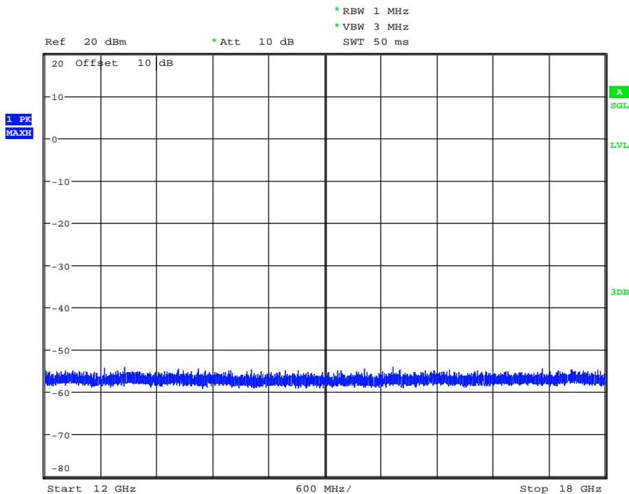
170297 SpurEmiss18-26G BT DH5 BT1.wmf: conducted spurious emissions (operation mode 1):
