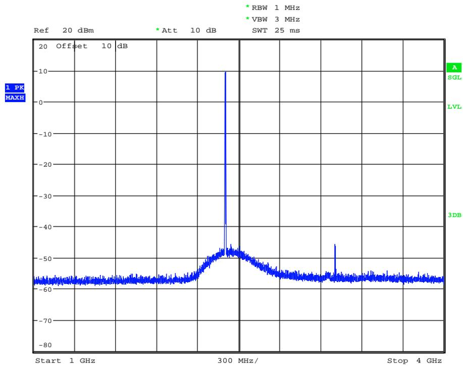
170297\_SpurEmiss4-12G\_BTLE\_BT1.wmf: conducted spurious emissions (operation mode 10):
