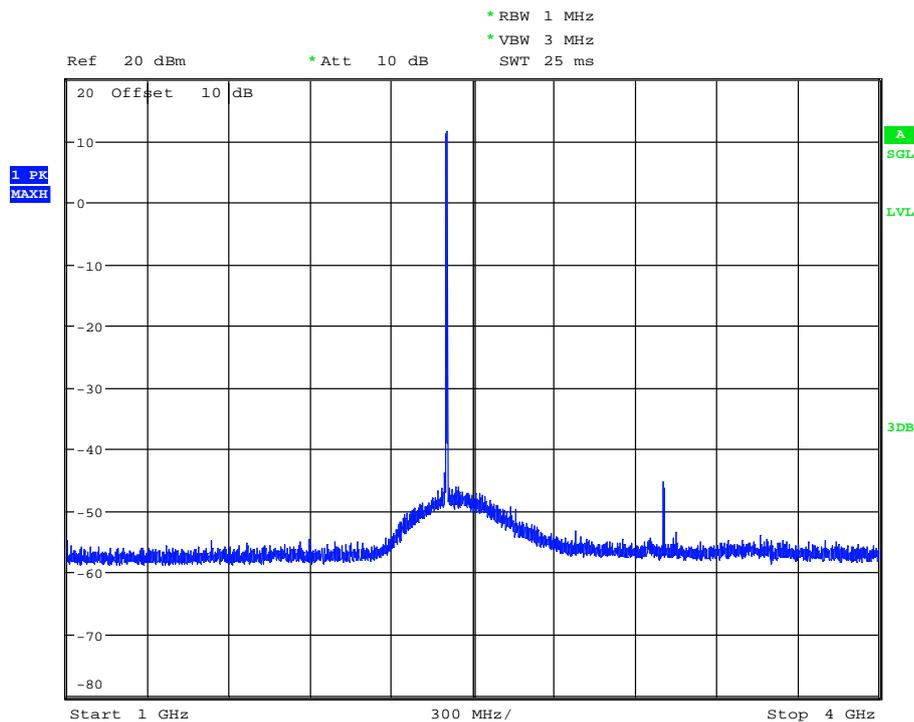
170297\_SpurEmiss4-12G\_BT\_DH5\_BT1.wmf: conducted spurious emissions (operation mode 1):
