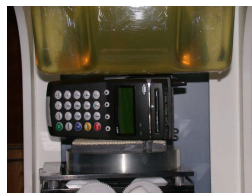
Figure 14.1 Body SAR Test Setup - Side
