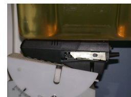
Figure 14.2 Body SAR Test Setup - Back
