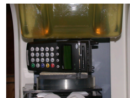
Figure 14.4 Body SAR Test Setup - Side
