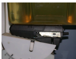
Figure 14.3 Body SAR Test Setup - Back
