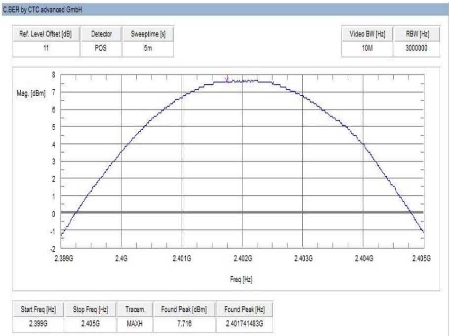
Plot 1: lowest channel – 2402 MHz, GFSK modulation
