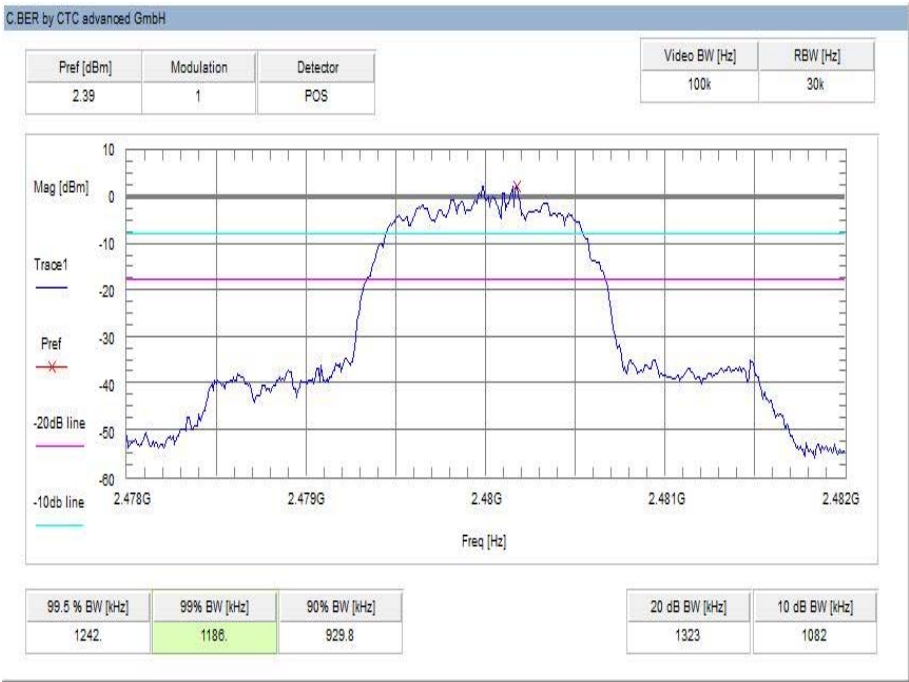
Plot 6: highest channel – 2480 MHz, Pi / DQPSK modulation
