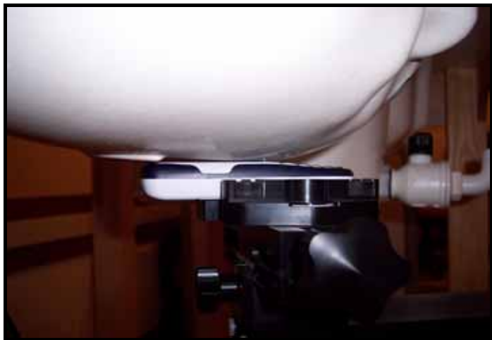
Figure 9.1 Right Head SAR Test Setup -- Cheek / Touch Position --
