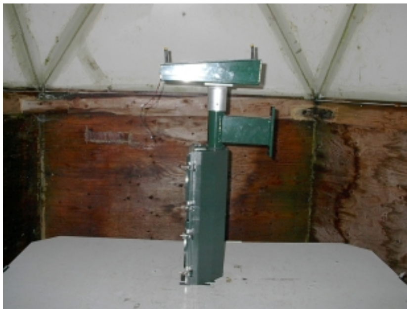
Emissions Test Setup SZF Mounted on Sample Lighting Post Side View
