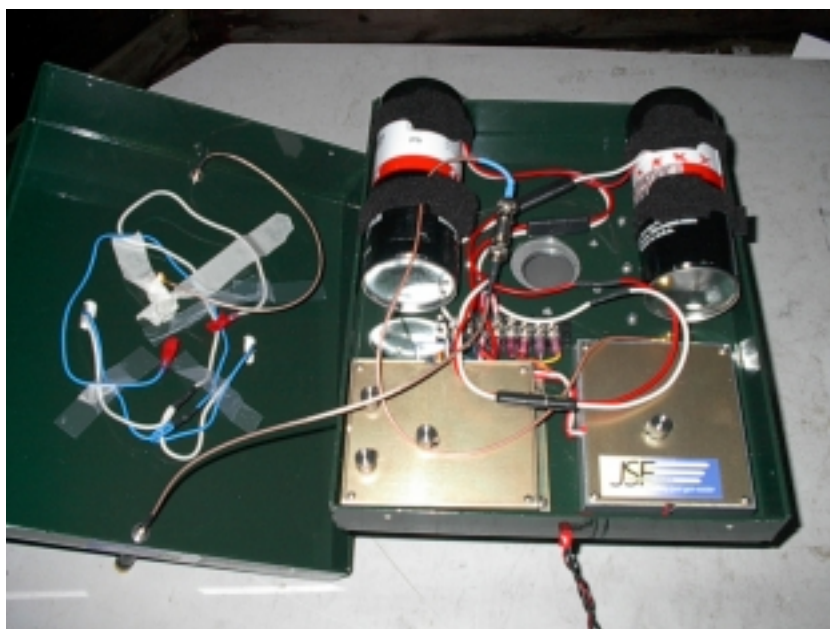
Emissions Test Setup of SZF Module Internal View Showing Batteries & RF Module
