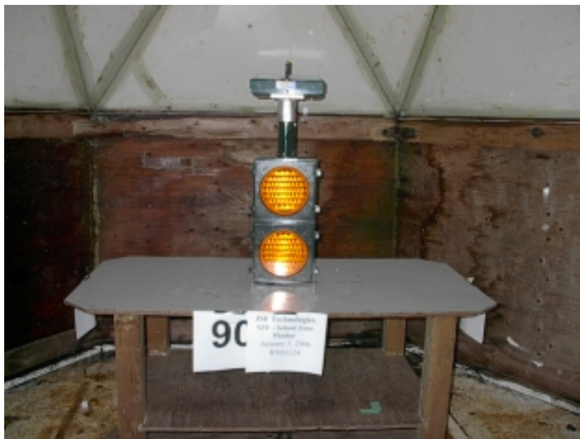
Emissions Test Setup SZF Mounted on Sample Lighting Post
