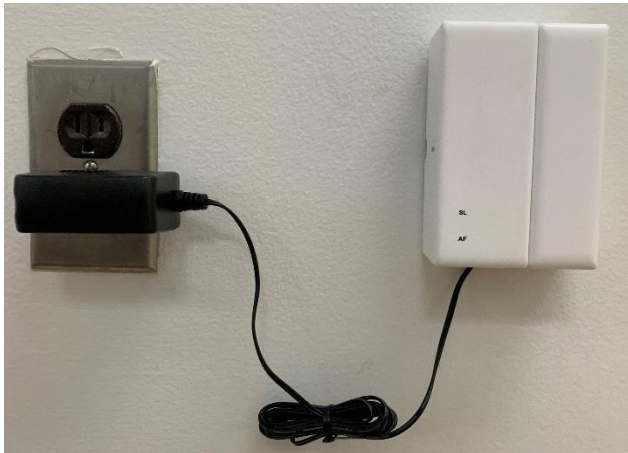
Figure 3: Front view of AP attached to Power Cradle and wall transformer
