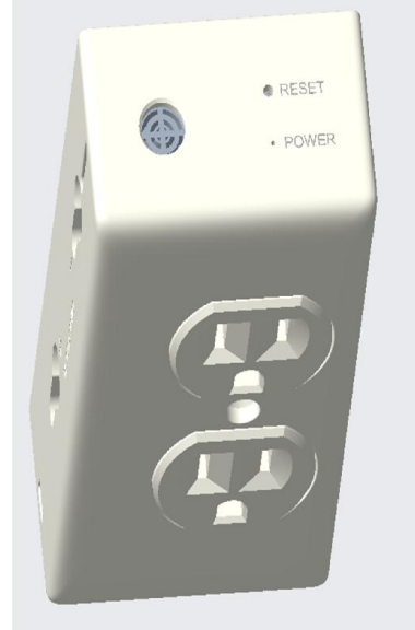
Image 12: Top view of Location Beacon AC Power
