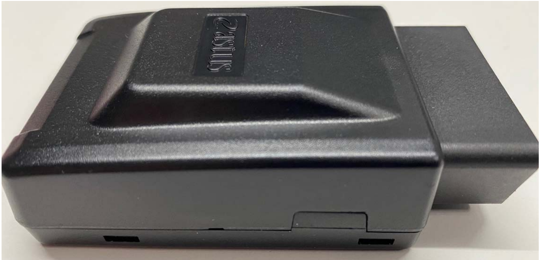
Side: Housing that hides the auxiliary connector
