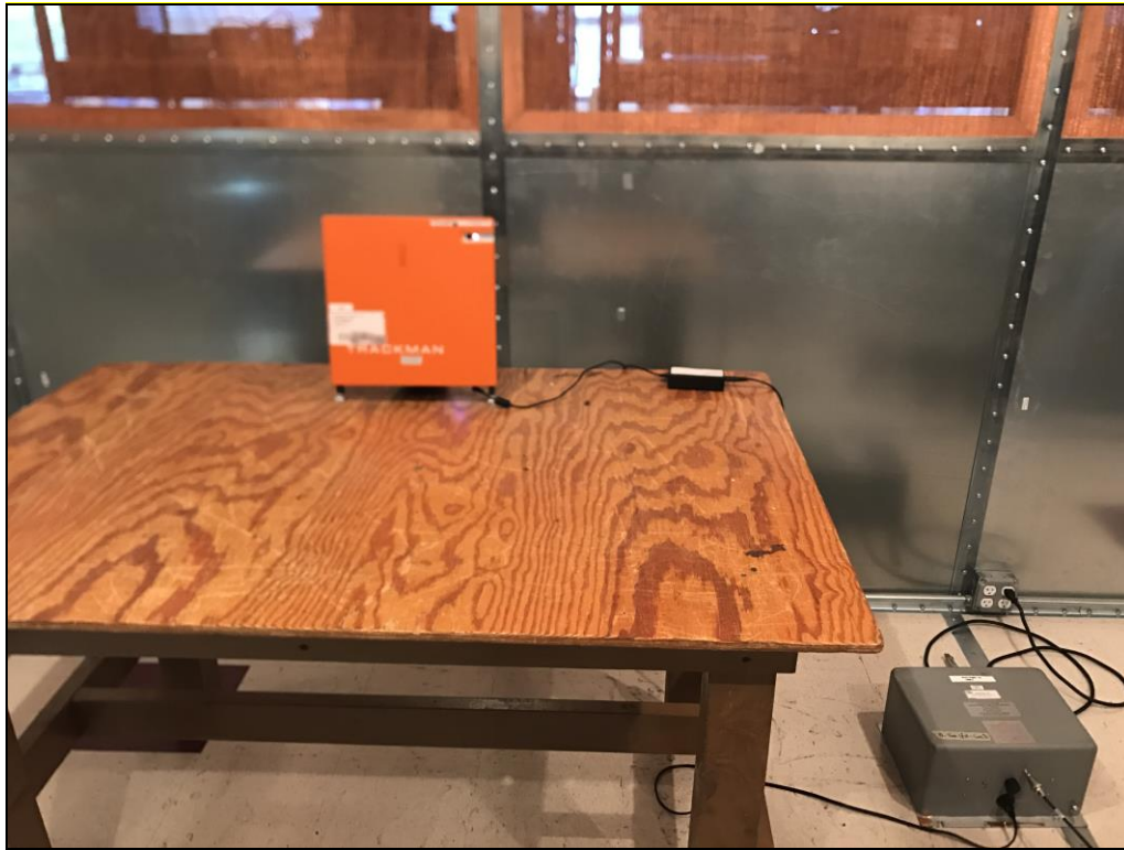
Photograph 2. Conducted Emissions, 15.207(a), Test Setup
