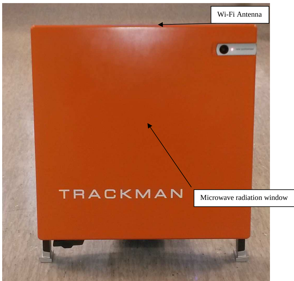
Figure 2: TrackMan™ radar unit, model TMAN4 front view
