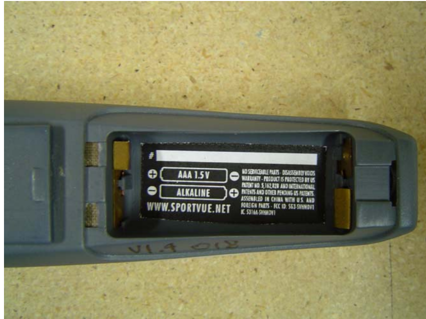
Fig. 4 - HMD battery location (need new photo with correct polarity indicated)
