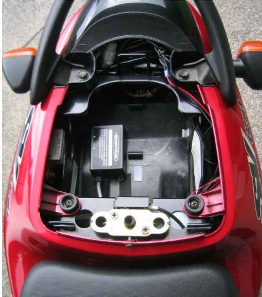
Fig. 8 Typical MSU Location
