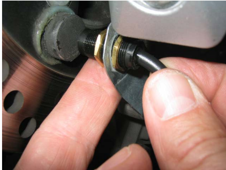
Fig.9 – Wheel Speed Sensor and magnet Installation
