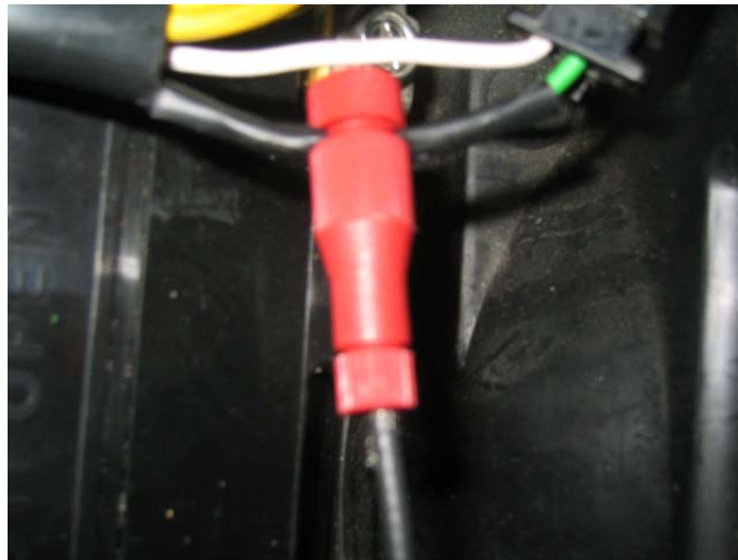
Fig. 11 – RPM wire tap
