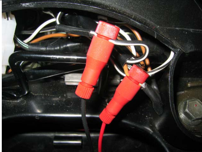
Fig. 12 - Power and ground wire taps
