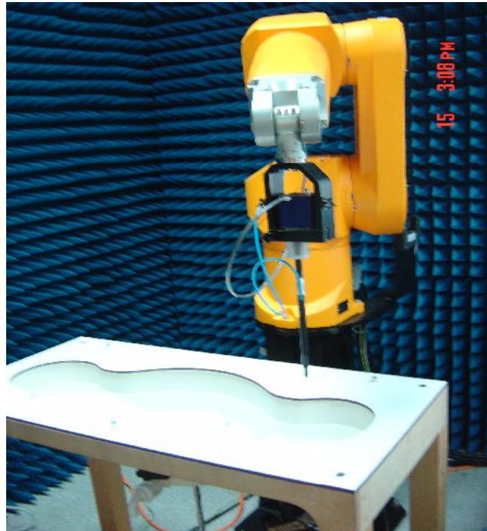
Fig.1 Photograph of the SAR measurement System
