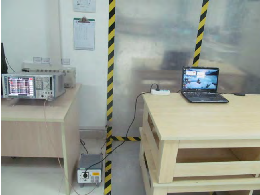
FCC RADIATED EMISSION TEST SETUP
