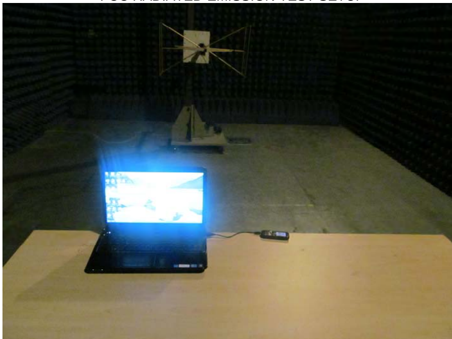
FCC RADIATED EMISSION TEST SETUP
