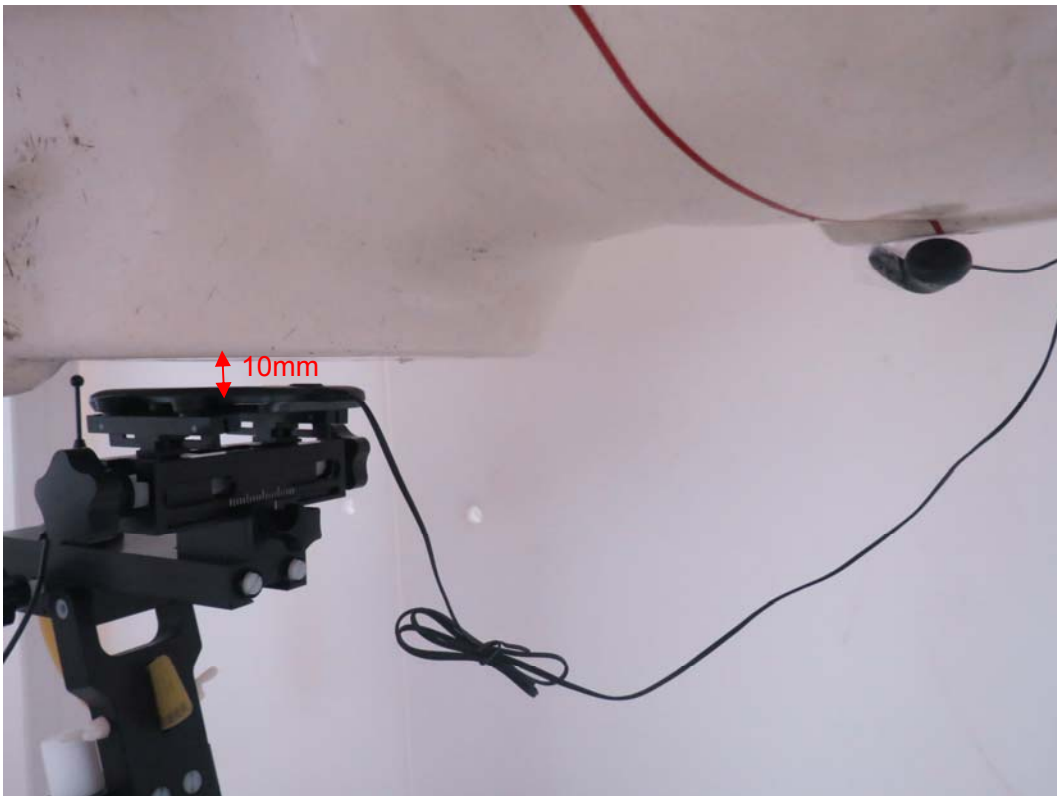
Picture 20: Back Side with earphone 2, the distance from handset to the bottom of the Phantom is 10mm
