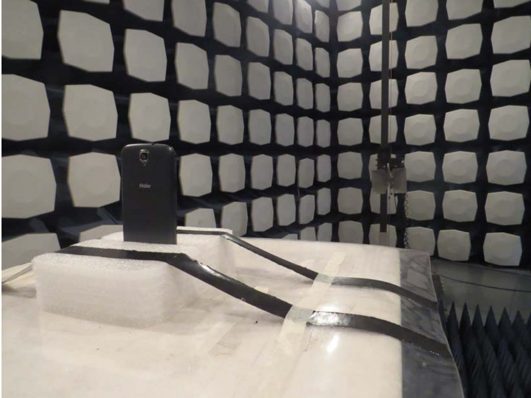
Picture 2: Radiated Spurious Emissions Test setup
