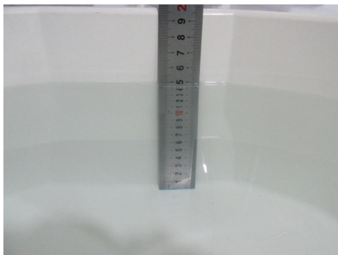
Fig.13 Body Liquid of 835MHz(15cm)
