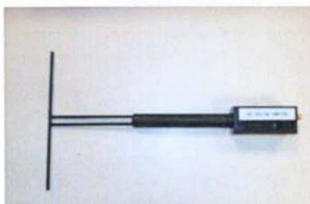
Figure 1 – Satimo COMOSAR Validation Dipole
