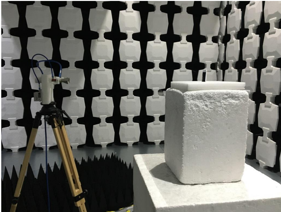
Description: Radiated Emission Test Setup (Above 18GHz)
