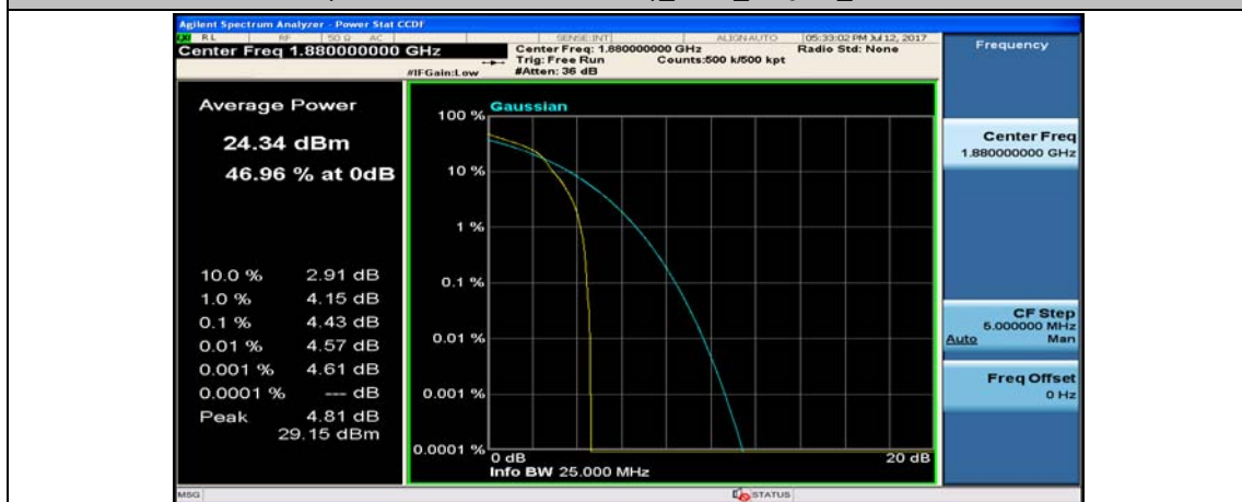
(Channel Bandwidth: 5 MHz)_MCH_16QAM_1RB#12
