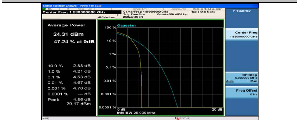
(Channel Bandwidth: 3 MHz)_MCH_16QAM_1RB#7
