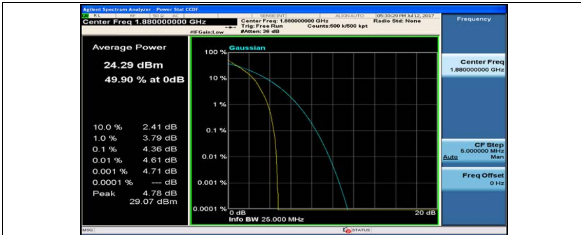
(Channel Bandwidth: 5 MHz)_MCH_QPSK_25RB#0
