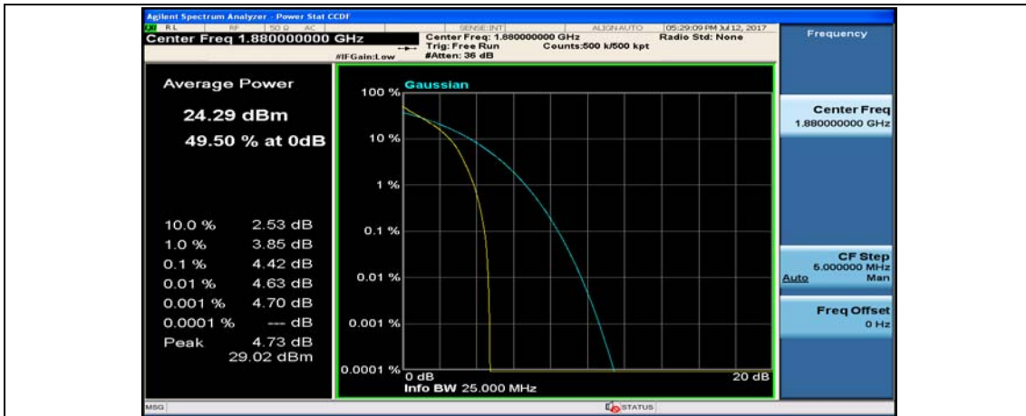
(Channel Bandwidth: 3 MHz)_MCH_QPSK_15RB#0
