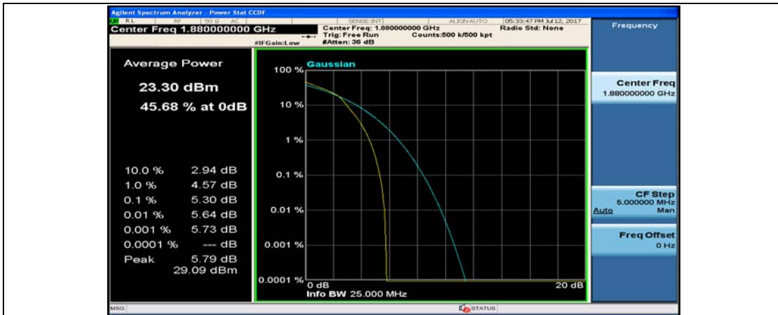
(Channel Bandwidth: 5 MHz)_MCH_16QAM_25RB#0
