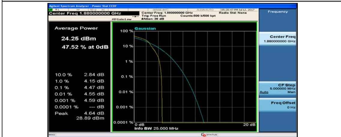
(Channel Bandwidth: 3 MHz)_MCH_16QAM_1RB#14
