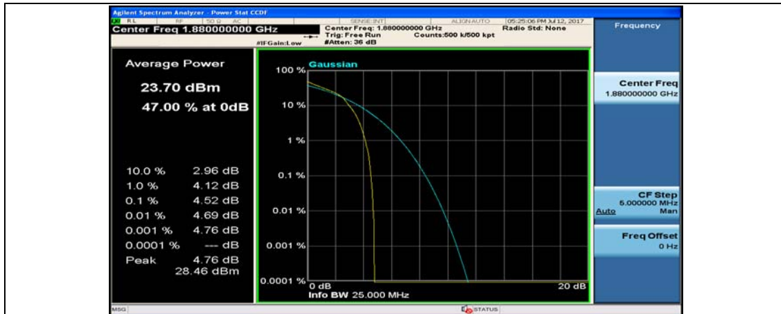
(Channel Bandwidth: 1.4 MHz)_MCH_16QAM_6RB#0
