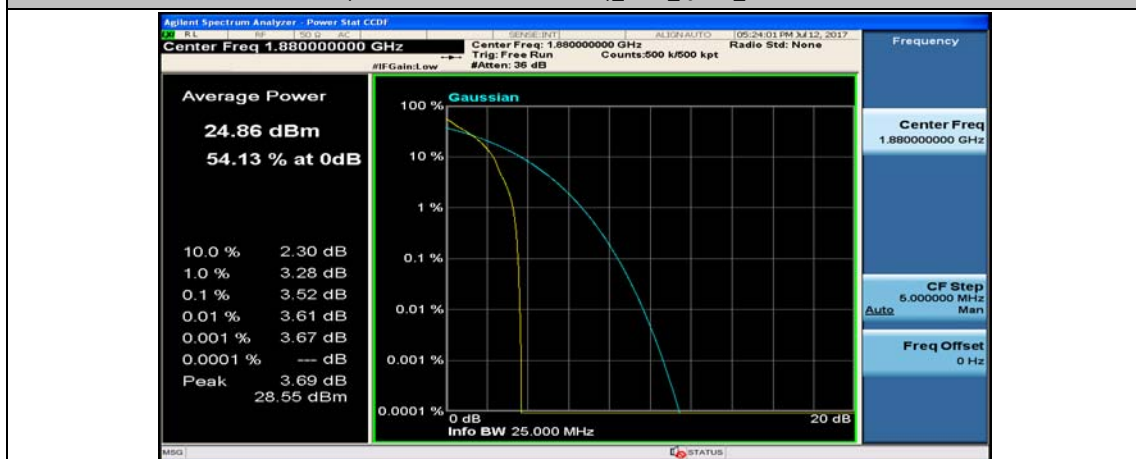
(Channel Bandwidth: 1.4 MHz)_MCH_QPSK_1RB#3
