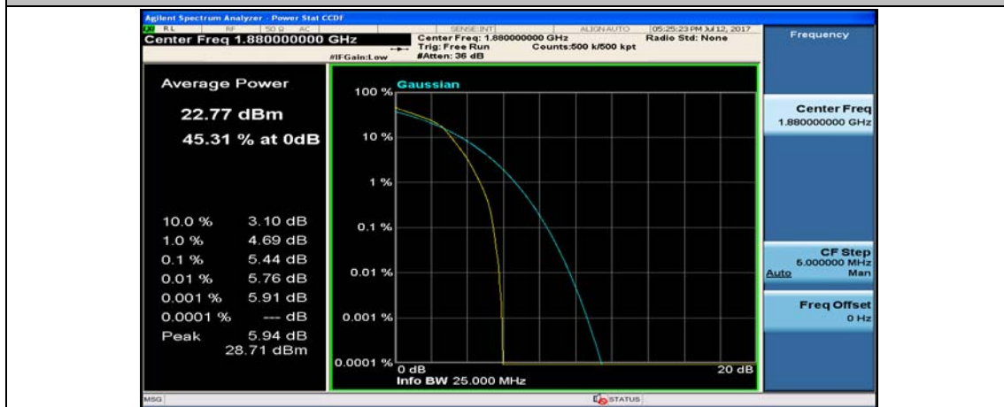
(Channel Bandwidth: 1.4 MHz)_MCH_16QAM_6RB#0
