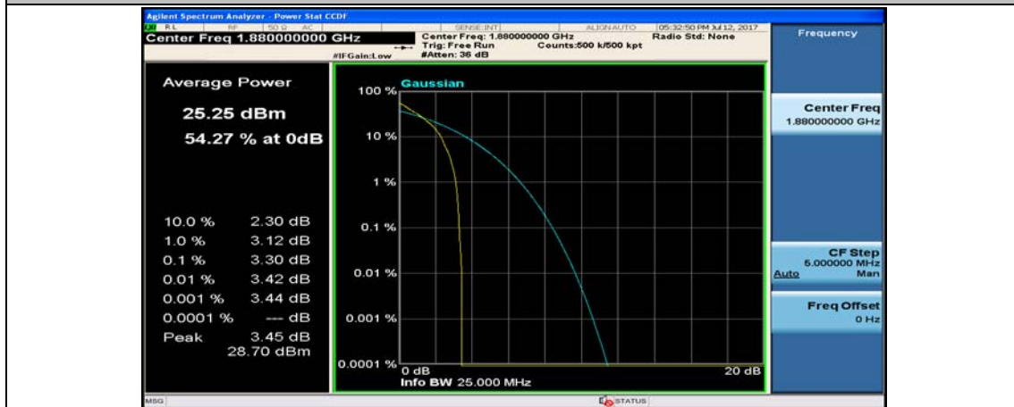
(Channel Bandwidth: 5 MHz)_MCH_QPSK_1RB#24
