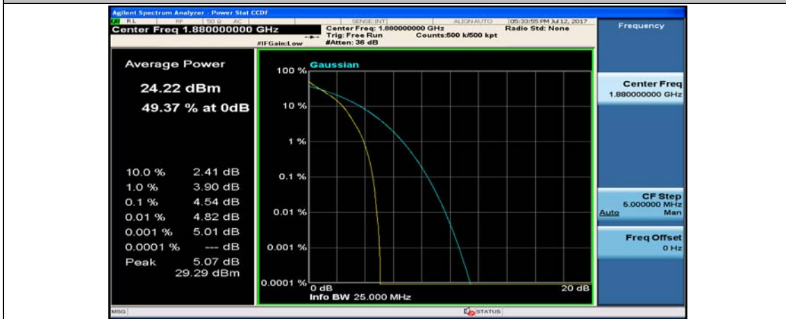
(Channel Bandwidth: 5 MHz)_MCH_QPSK_25RB#0
