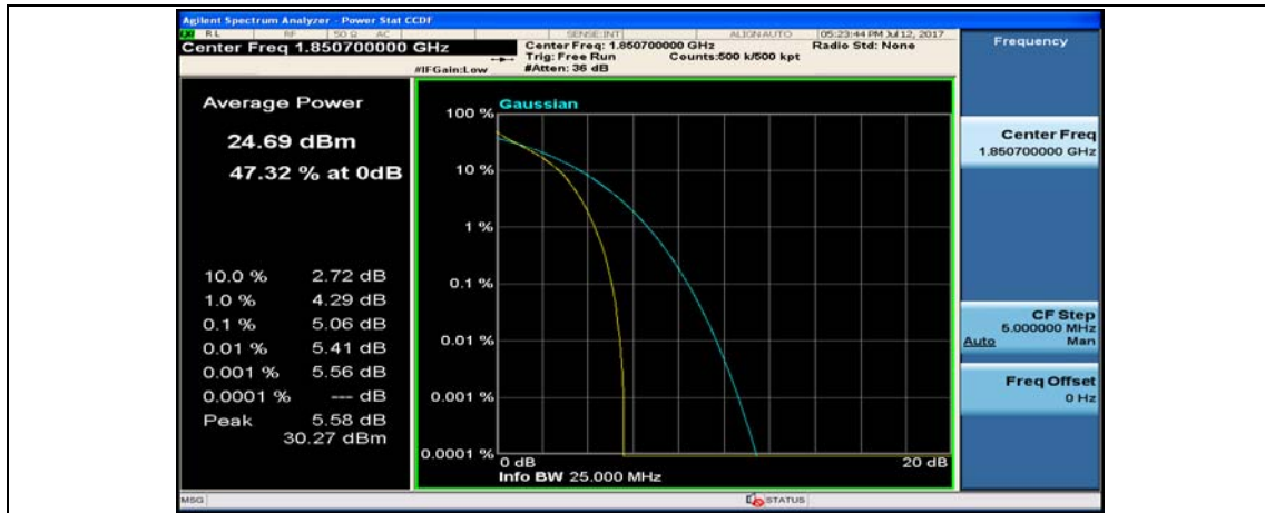
(Channel Bandwidth: 1.4 MHz)_MCH_QPSK_1RB#0
