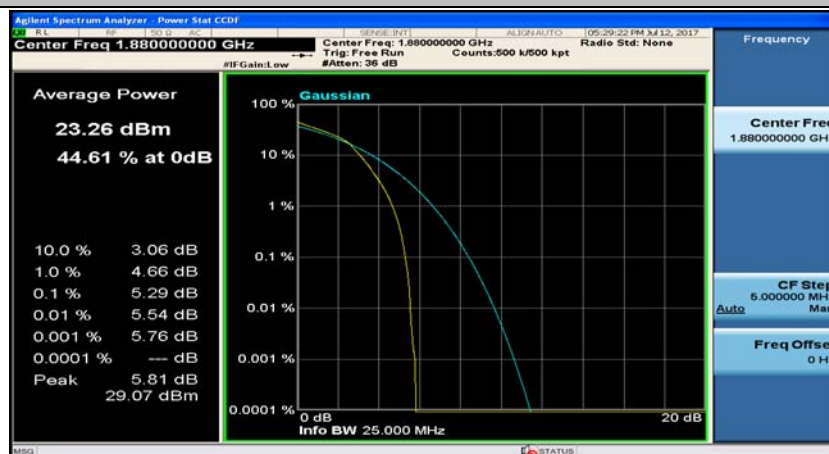
(Channel Bandwidth: 3 MHz)_MCH_16QAM_8RB#7
