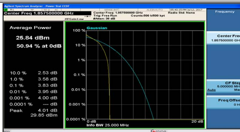
(Channel Bandwidth:15 MHz)_LCH_QPSK_37RB#0
