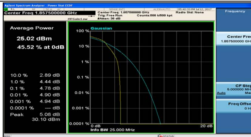
(Channel Bandwidth:15 MHz)_LCH_16QAM_37RB#0
