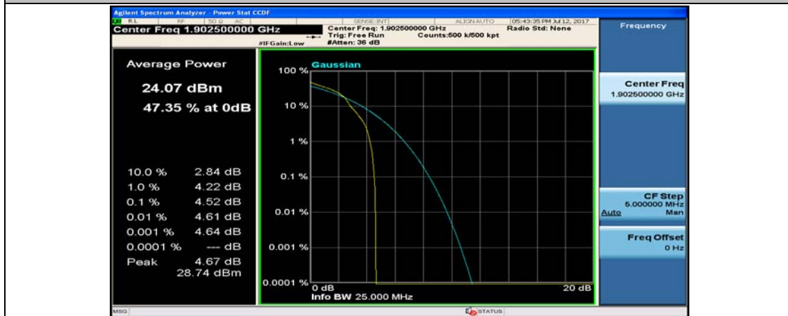
(Channel Bandwidth:15 MHz)_HCH_16QAM_1RB#37
