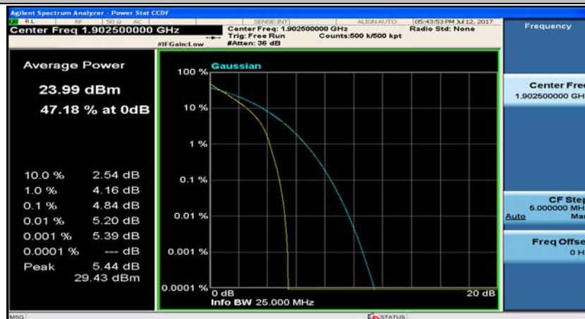
(Channel Bandwidth:15 MHz)_HCH_QPSK_37RB#18
