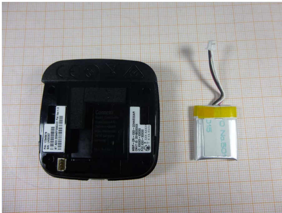
Photo 2: Battery pack removed
