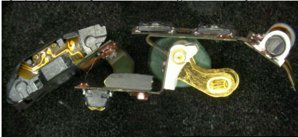
Fig 2: two versions (with/ without plastic shell) of stripped CAD pictures from the inside of Type RIC 13 hearing aid
