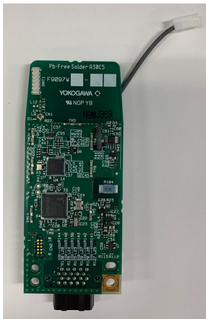
Figure 1.2.2. WCM ASSY A-side (Removed the shield)
