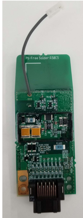
Figure 1.2.3. WCM ASSY B-side (Before molding)
