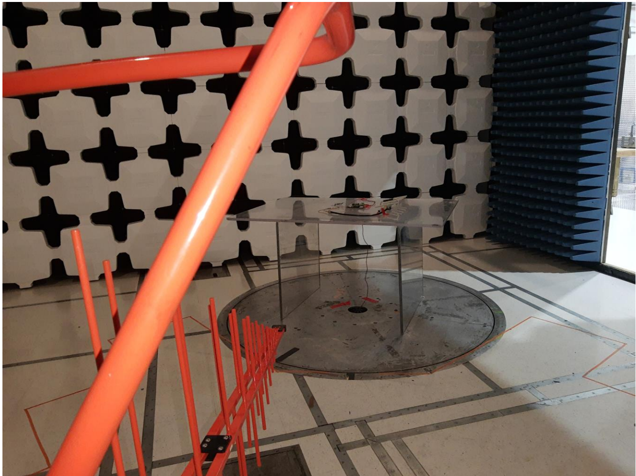
Figure 3: Radiated Emissions Test Setup - 30-1000MHz - 12dBi configuration
