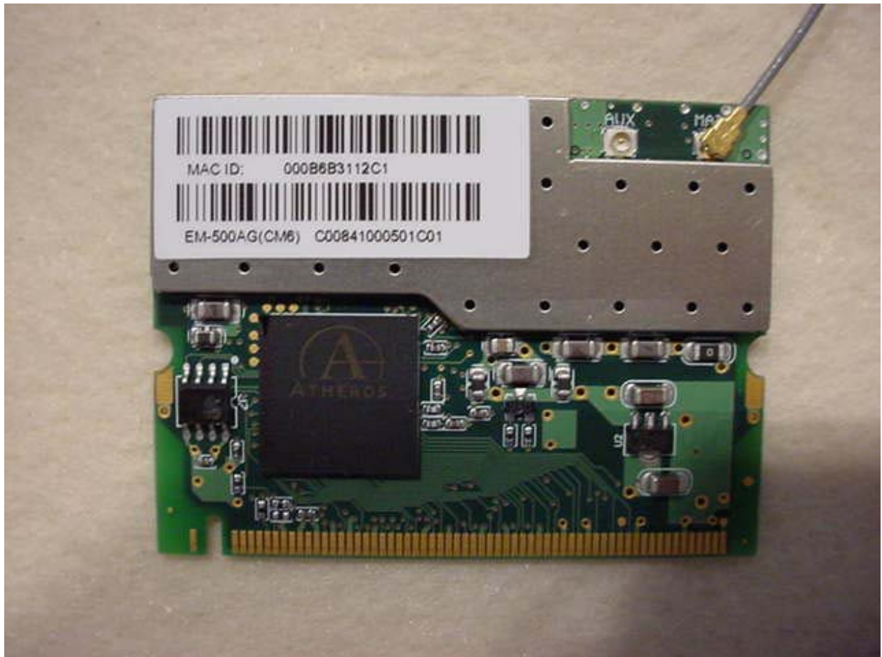
Figure 6: Mini-PCI 802.11 a/b/g Radio Card – Bottom View
