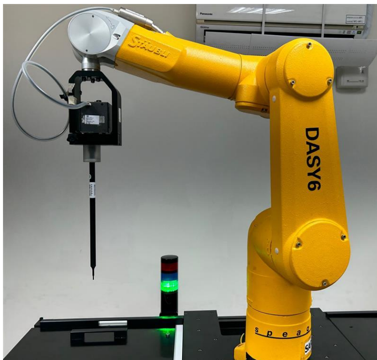
Fig.1 Photograph of the SAR measurement system
