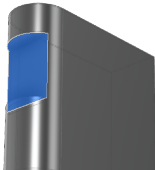
Optimal antenna placement is against the glass on the interior of the faceplate (blue area)
