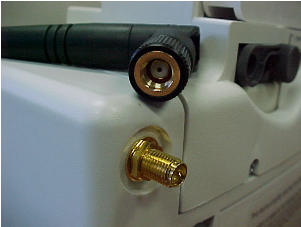
Photo Six – External Close-Up of Antenna connection – Reverse SMA
