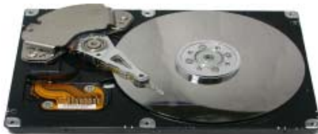
Figure 2. Internal structure of HDD Drive
