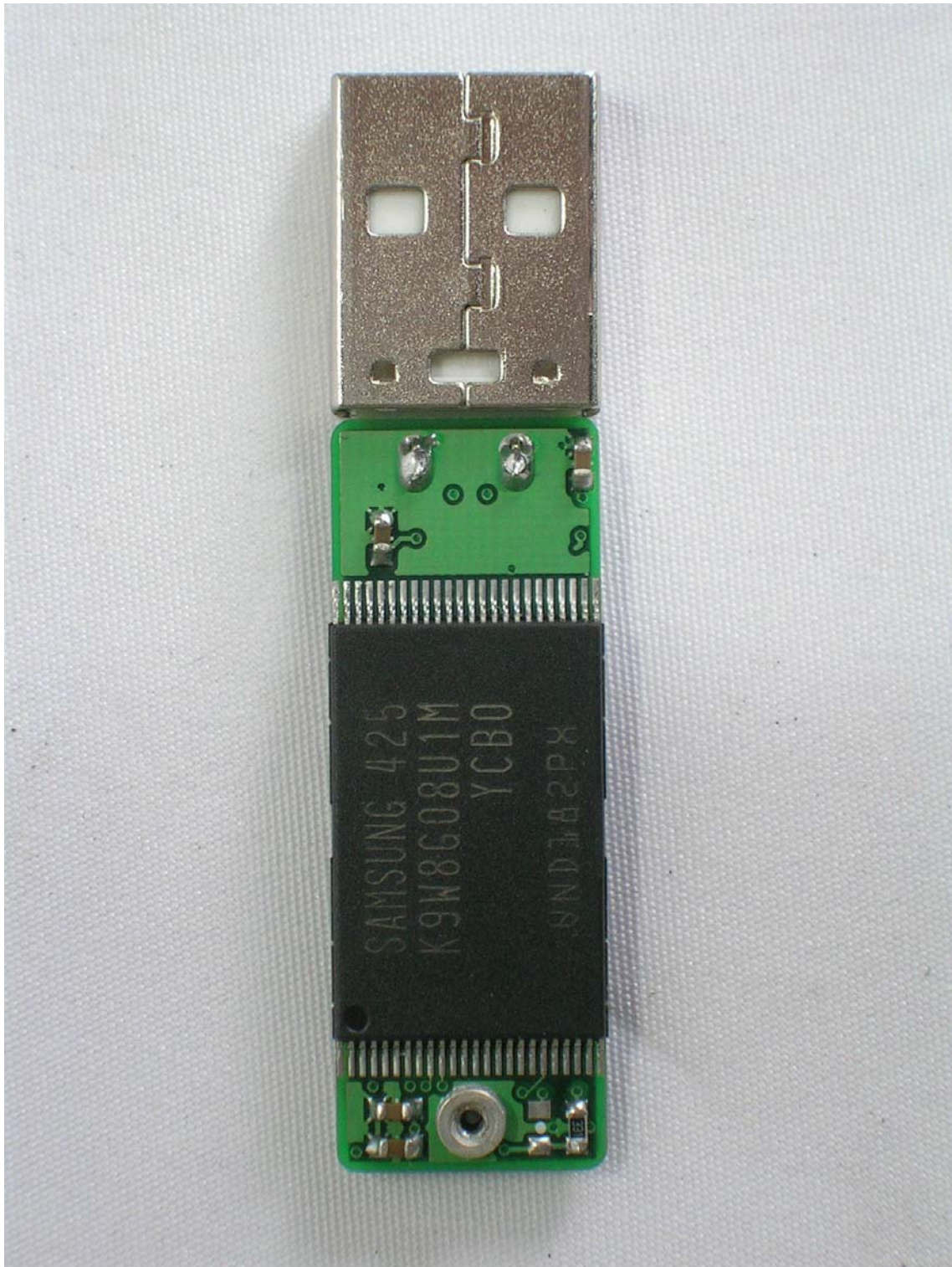
<REAR VIEW OF MAIN BOARD>
