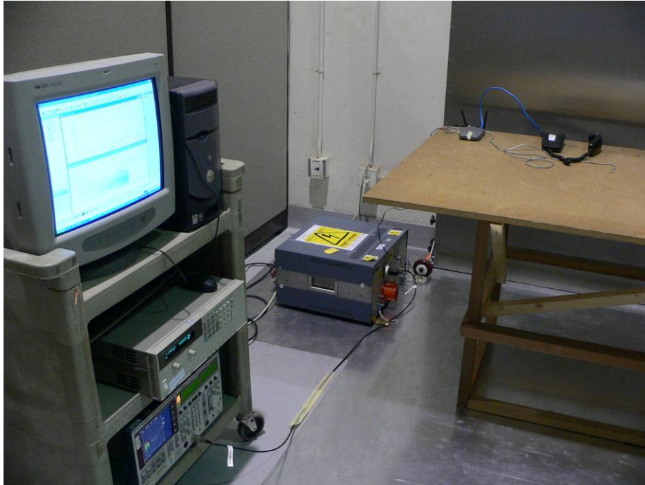
Conducted Emission - Front View
