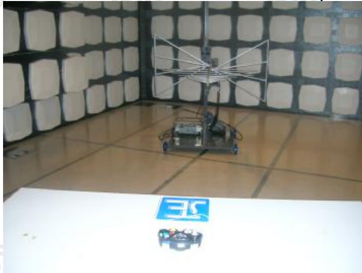
Measurement of Radiated Emission Test Set Up
